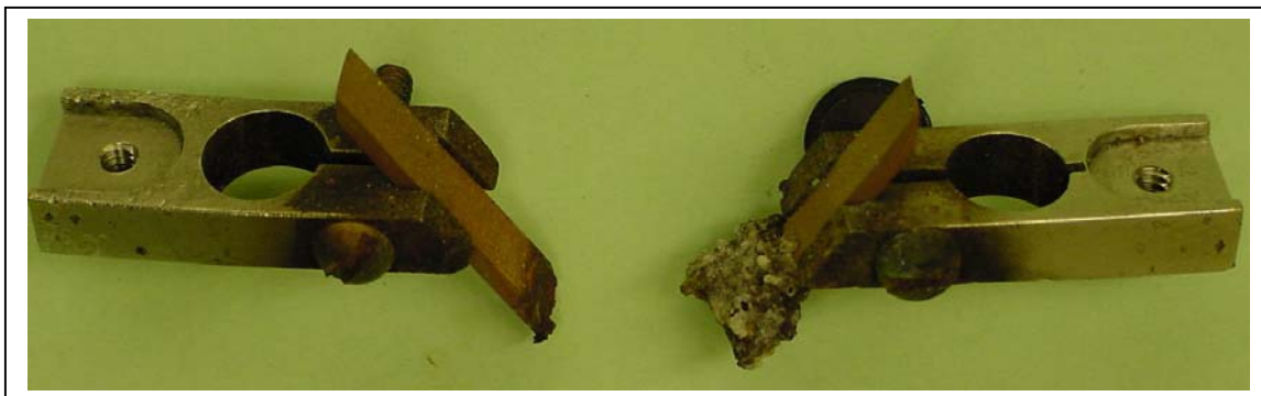
Figure 5 - Test Electrodes Following Completion of Test 6
