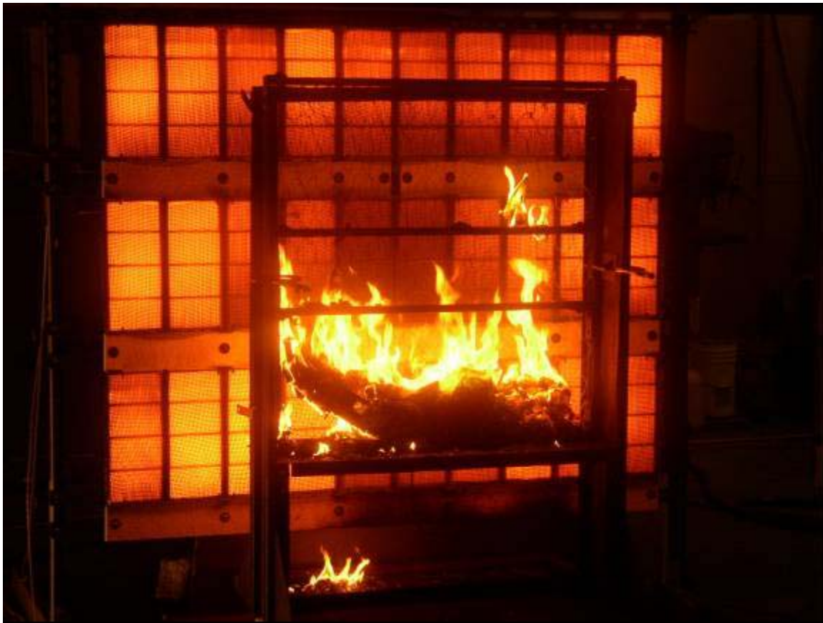
Figure 12. Windshield – ICAL Test in Progress.
