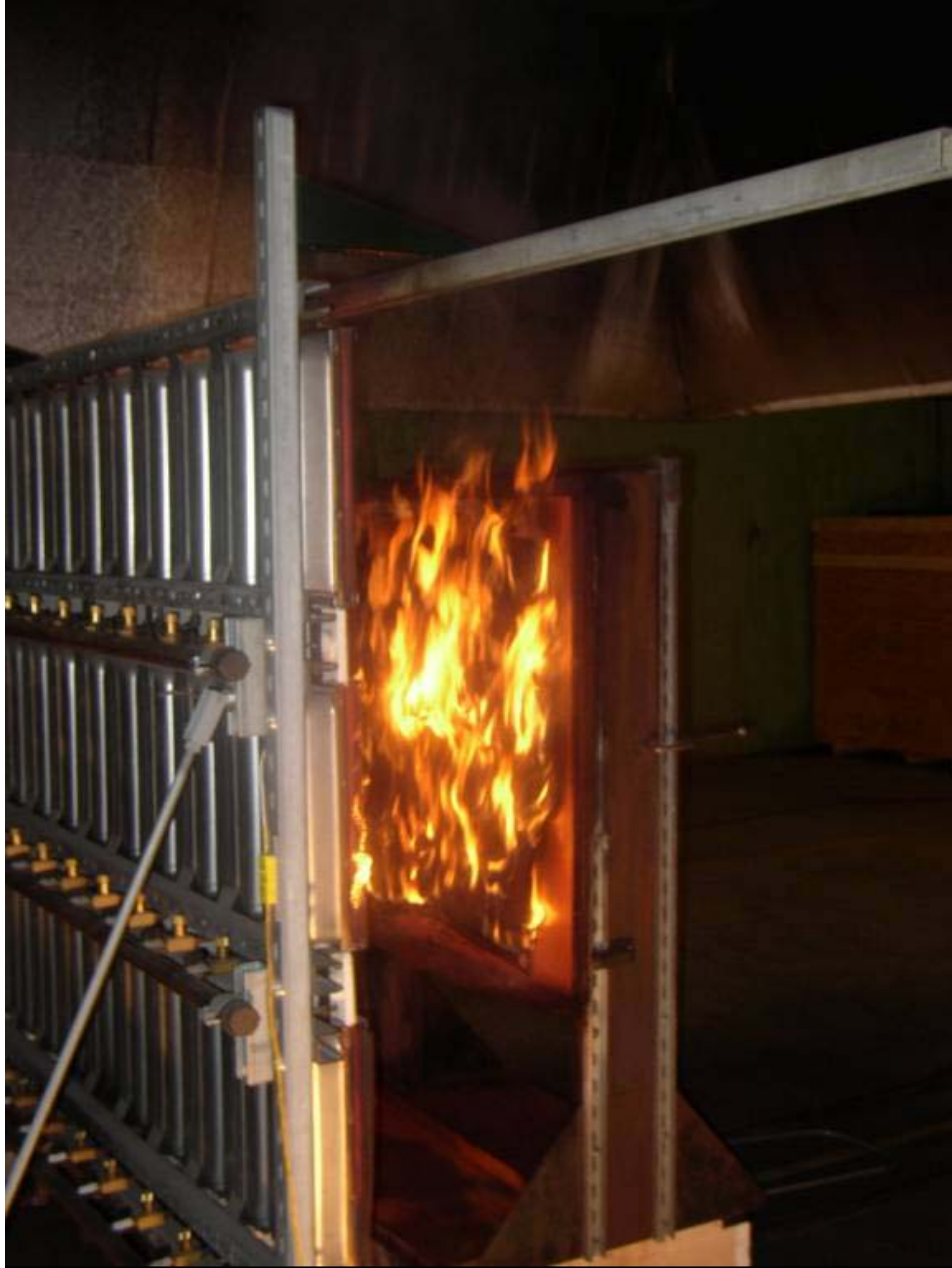
Figure 10. Hood Liner Face – ICAL Test in Progress.
