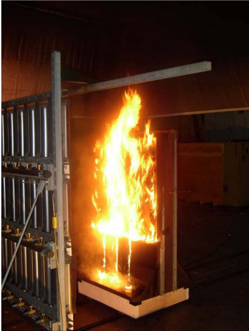
Figure 7. Battery Cover – ICAL Test in Progress.
