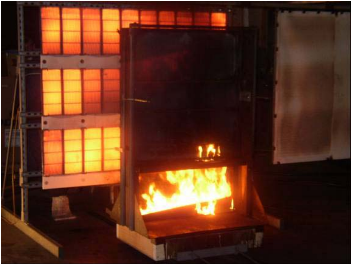
Figure 8. Air Ducts – ICAL Test in Progress.
