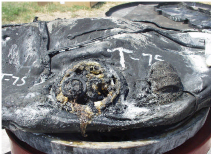
Figure A-180. Test No. 7S, Top View of New 1998 Plymouth Grand Voyager Fuel Tank After Fire Exposure With Leak Location at Sending Unit of Fuel Tank.
