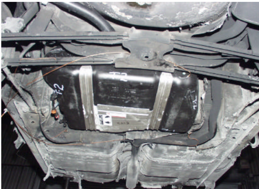
Figure A-70. Test No. 2, Repeatability Evaluation on a New 1998 Saturn Twin Cam 4-Door Fuel Tank Mounted in the Test Platform Prior to Testing.
