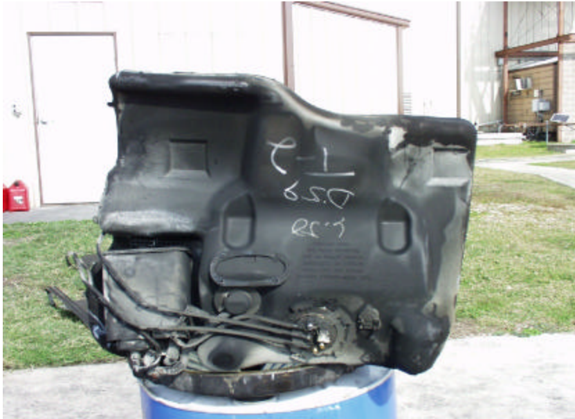
Figure A-58. Test No. 2, Top View of New 1998 Saturn Twin Cam 4-Door Fuel Tank After Fire Exposure.
