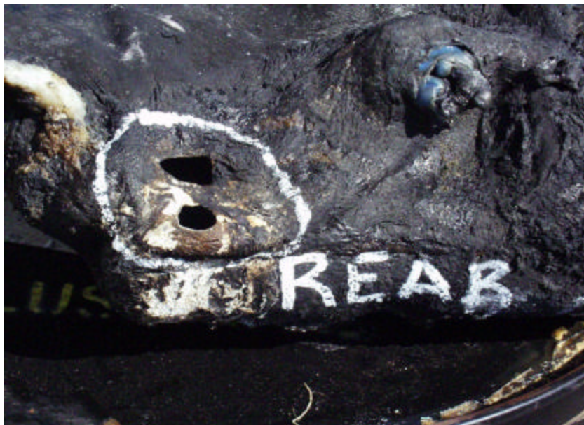
Figure A-193. Test No. 1 (January 21, 2003), Driver Side Fire Exposure Hole, Rear Topside of New 2000 Chevrolet Cavalier Plastic Fuel Tank.
