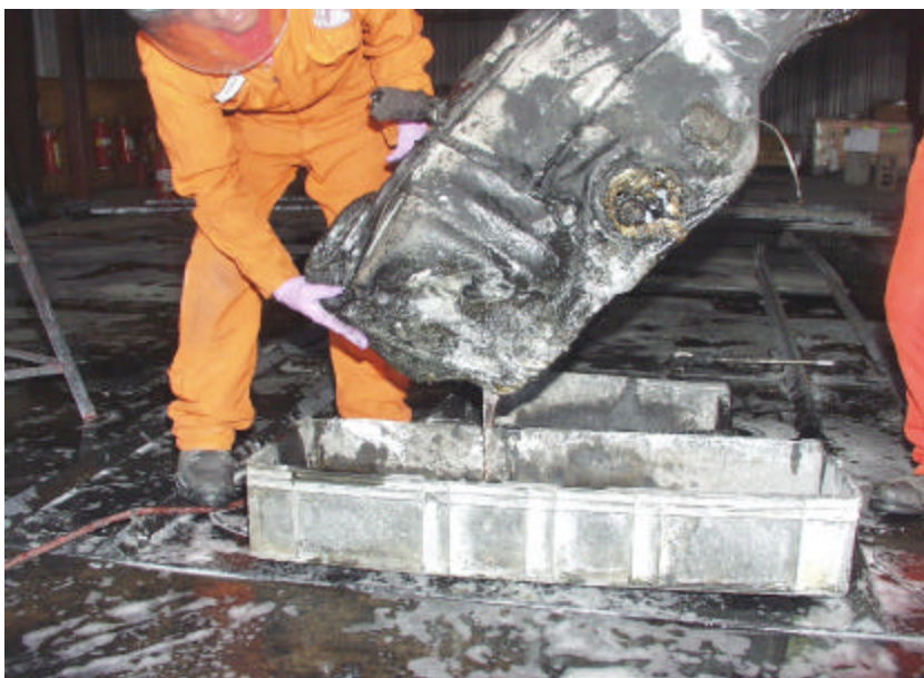
Figure A-176. Test No. 7S, Top View of New 1998 Plymouth Grand Voyager Fuel Tank After Fire Exposure With Leak Location at Rear Corner Driver Side of Fuel Tank.
