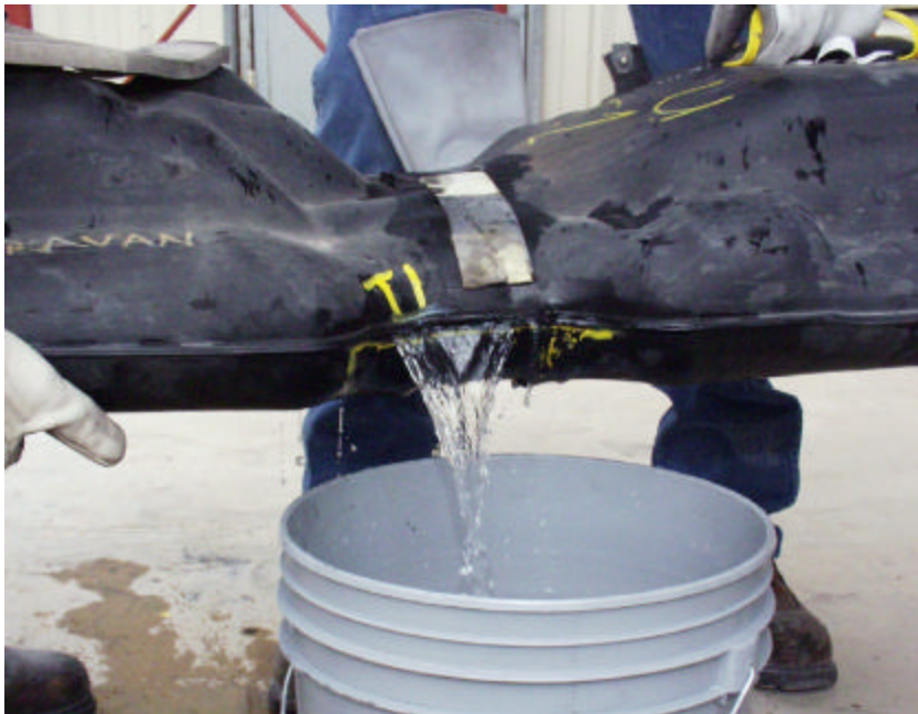
Figure A-30. Leakage of New Plymouth Plastic Fuel Tank After Impact.
