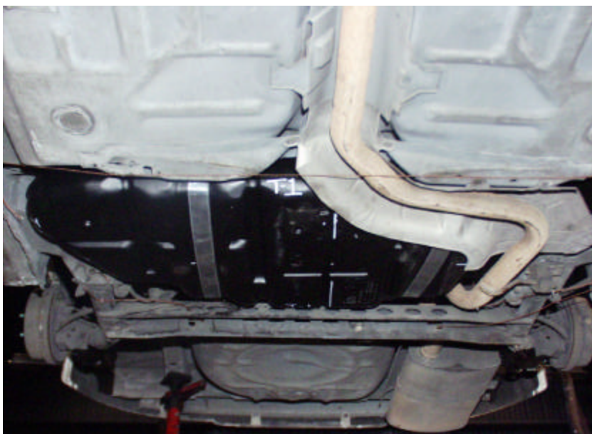
Figure A-187. Test No. 1 (January 21, 2003), New 2000 Chevrolet Cavalier Plastic Fuel Tank Mounted in Test Platform Prior to Testing.
