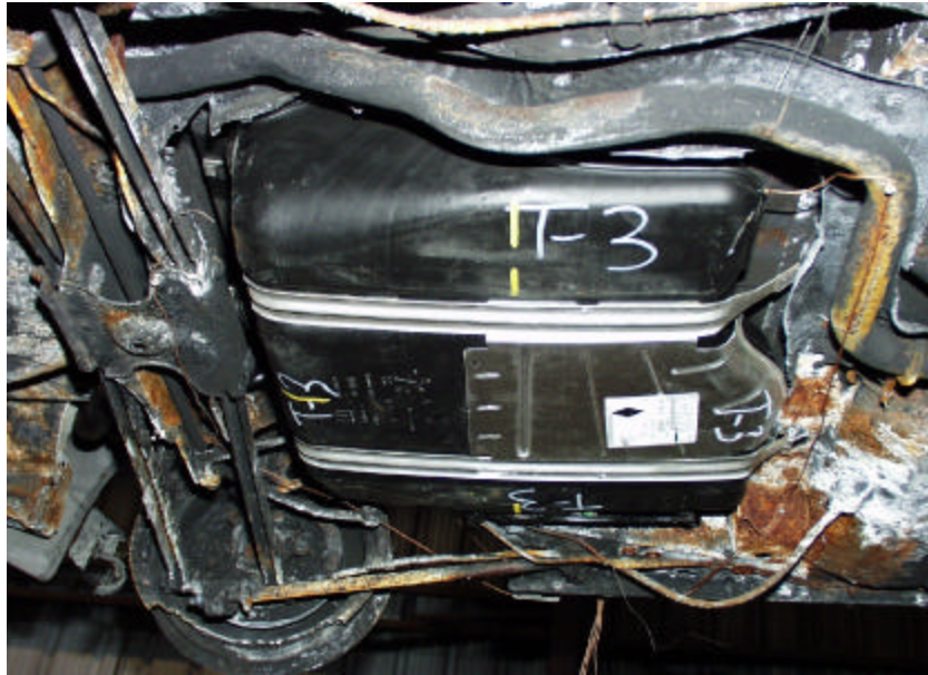
Figure A-81. Test No. 3, Repeatability Evaluation on a New 1998 Saturn Twin Cam 4-Door Fuel Tank Assembly Mounted in Test Platform Prior to Testing.
