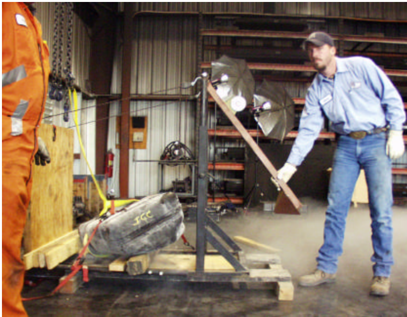
Figure A-27. Impact Resistance Test Setup.
