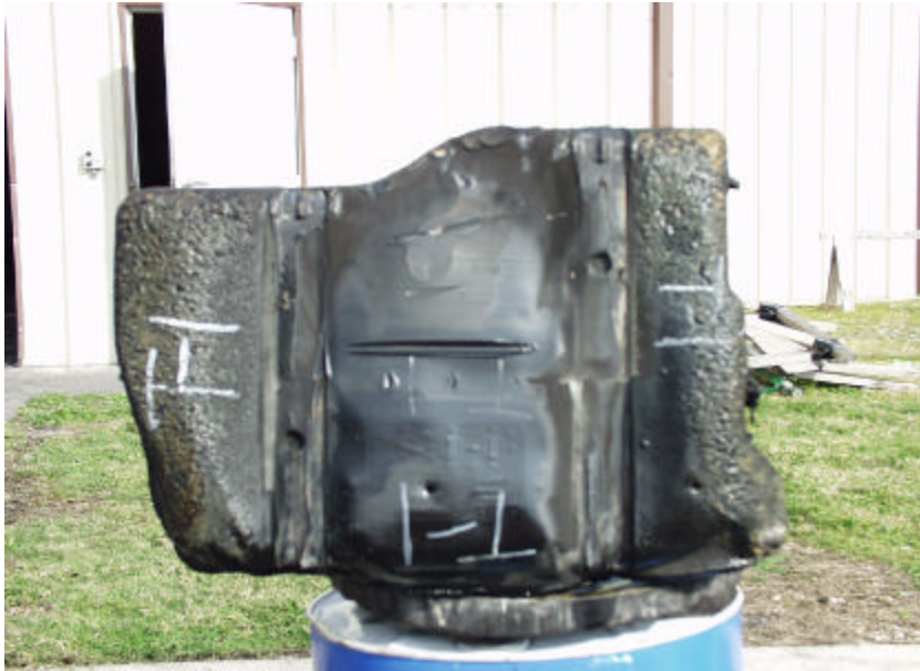
Figure A-50. Test No. 1, Bottom View of Conditioned 1998 Saturn Twin Cam 4-Door Fuel Tank After Fire Exposure.
