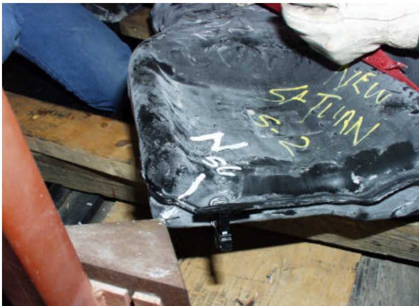
Figure A-209. Front Driver Side of the New 1998 Saturn Twin Cam 4-Door Fuel Tank Prior to Impact.
