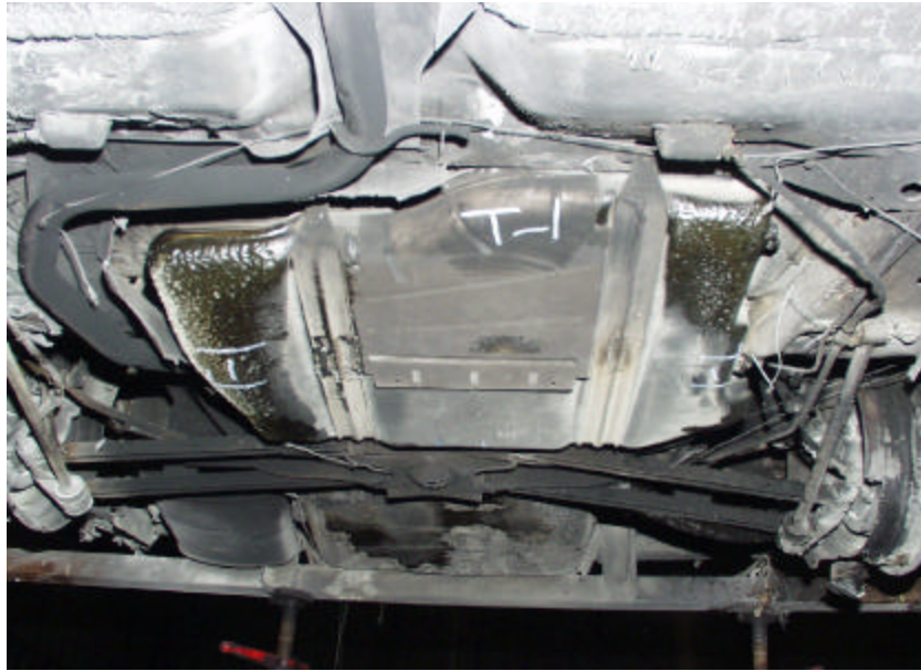
Figure A-65. Test No. 1, Repeatability Evaluation on a New 1998 Saturn Twin Cam 4-Door Fuel Tank with No Leaks; Classified as a Non-Failed Test.
