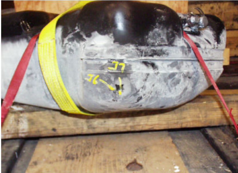
Figure A-214. No Leaks to the Front Driver Side of the Conditioned 1998 Jeep Grand Cherokee Fuel Tank After Two Impacts Ranging Between 43.6 Nm and 147.2 Nm.
