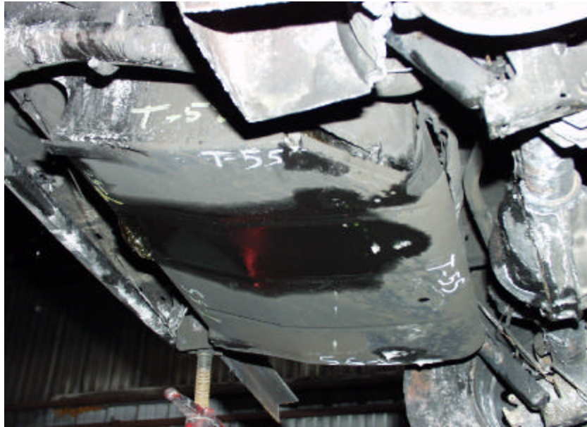
Figure A-119. Test No. 5S, New 1998 Jeep Grand Cherokee Fuel Tank Immediately After Fire Exposure with Heat Shield and Leak Location at Rear of Tank.
