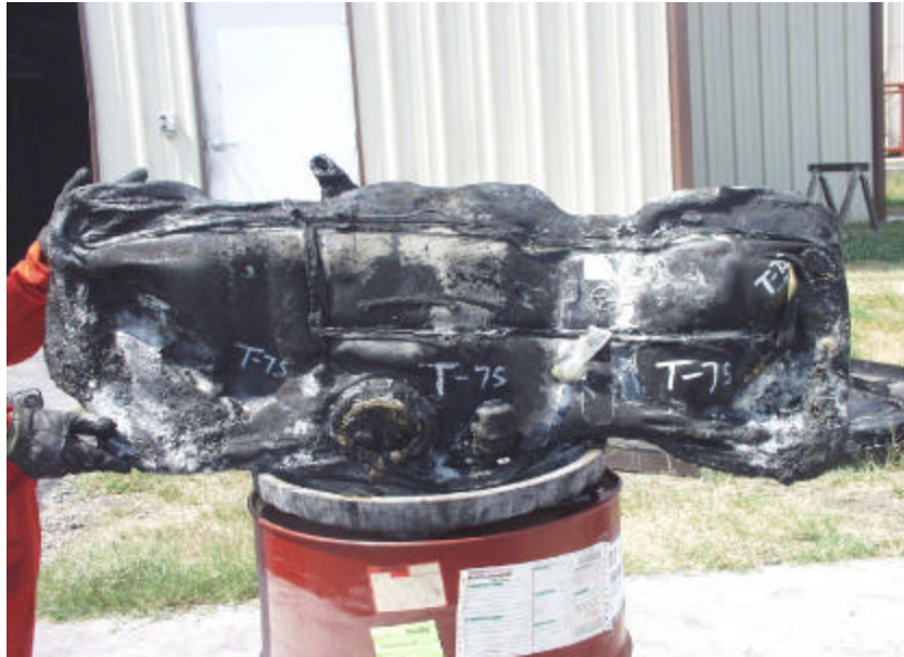
Figure A-177. Test No. 7S, Top Front View of New 1998 Plymouth Grand Voyager Fuel Tank After Fire Exposure.
