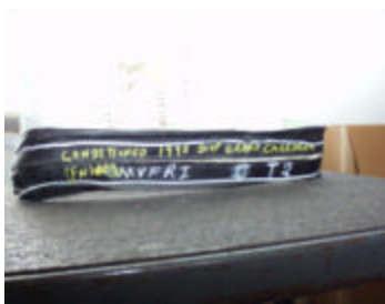
Figure 34. External View of Jeep Tank Pinch-Off Section.
