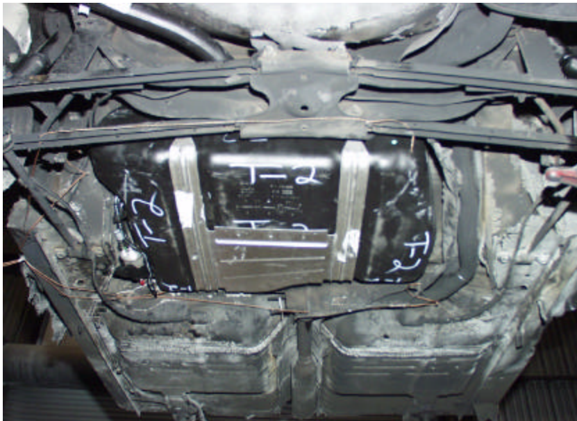
Figure A-55. Test No. 2, New 1998 Saturn Twin Cam 4-Door Fuel Tank Mounted in Test Platform Prior to Testing.
