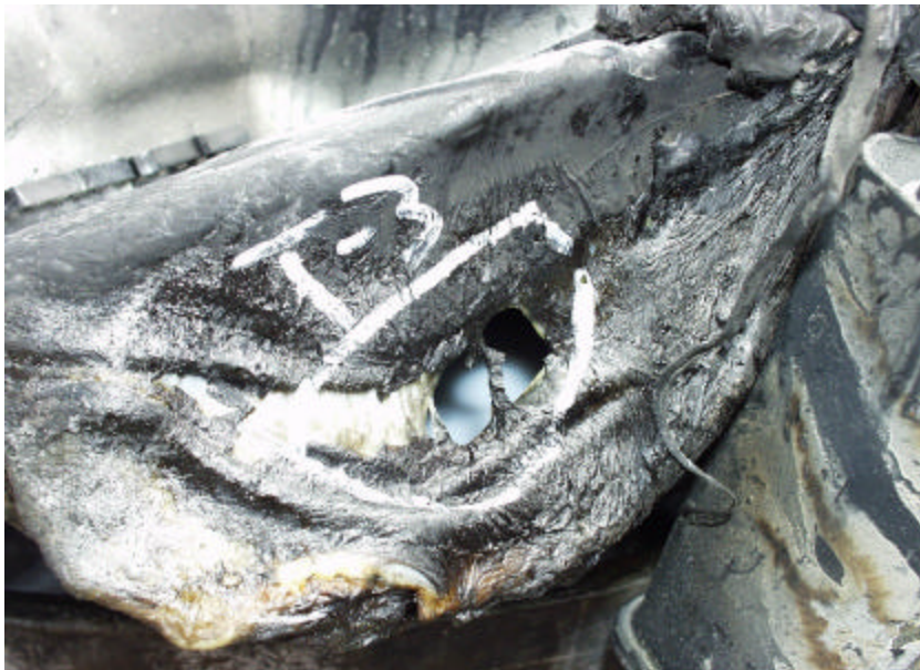
Figure A-88. Test No. 3, Saturn Twin Cam 4-Door Fuel Tank Post-Test Observation at Rear Left Passenger Side of Fuel Tank.
