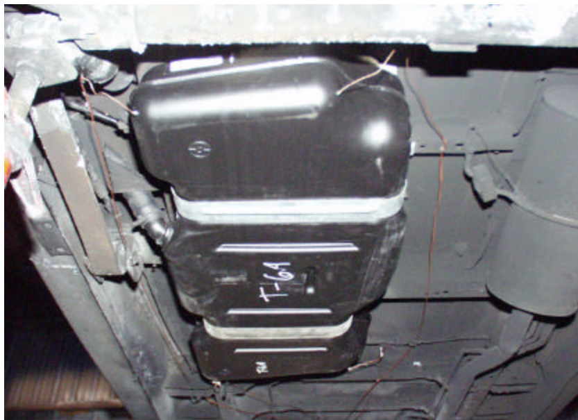
Figure A-146. Test No. 6A, New 1998 Plymouth Grand Voyager Fuel Tank Mounted in Test Platform Prior to Testing.
