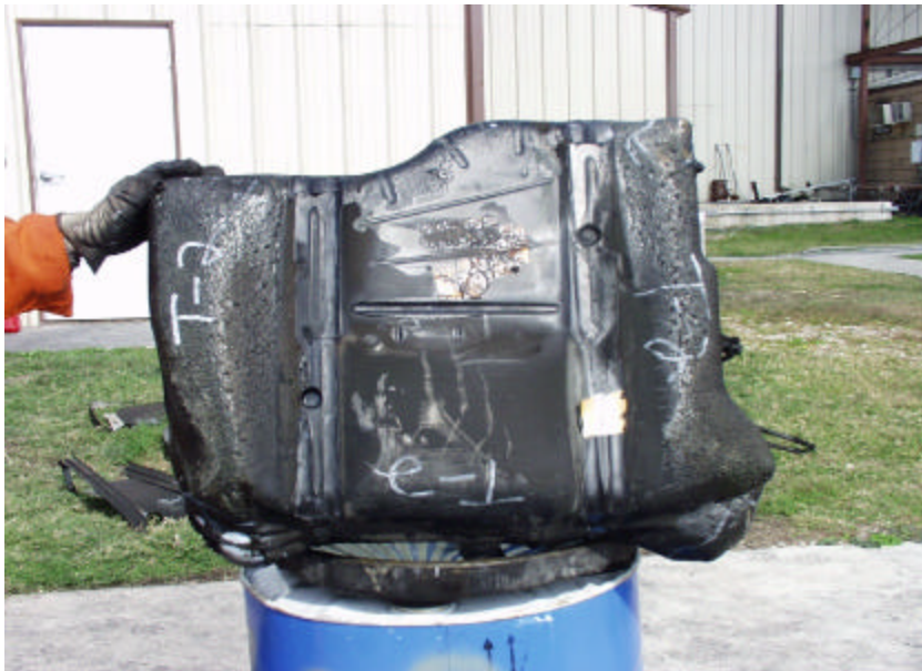
Figure A-59. Test No. 2, Bottom View of New 1998 Saturn Twin Cam 4-Door Fuel Tank After Fire Exposure.
