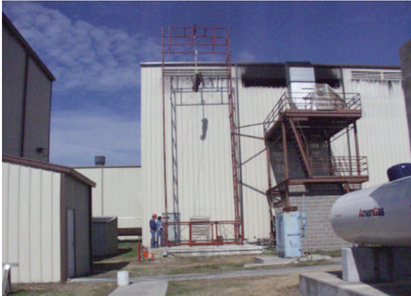
Figure A-235. The New 1998 Plymouth Grand Voyager Fuel Tank at 30-ft Elevation.
