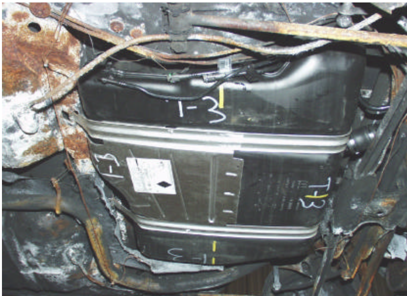
Figure A-80. Test No. 3, Repeatability Evaluation on a New 1998 Saturn Twin Cam 4-Door Fuel Tank Assembly Mounted in the Test Platform Prior to Testing.
