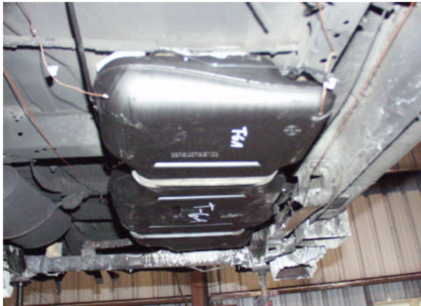
Figure A-145. Test No. 6A, New 1998 Plymouth Grand Voyager Fuel Tank Mounted in Test Platform Prior to Testing.
