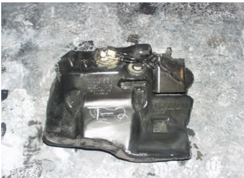
Figure A-76. Test No. 2, Repeatability Evaluation on a New 1998 Saturn Twin Cam 4-Door Fuel Tank After Fire Exposure, Top View.
