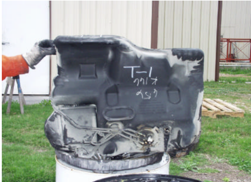
Figure A-67. Test No. 1, Repeatability Evaluation on a New 1998 Saturn Twin Cam 4-Door Fuel Tank with No Leaks, Top View; Classified as a Non-Failed Test.
