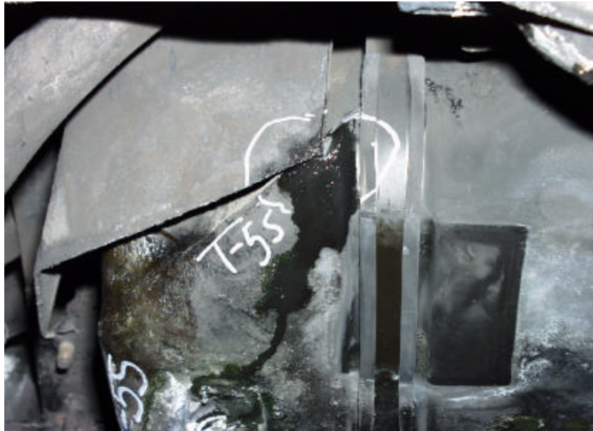
Figure A-125. Test No. 5S, New 1998 Jeep Grand Cherokee Fuel Tank Immediately After Fire Exposure with Leak Location at Front Right Corner of Tank due to Exhaust Shield.
