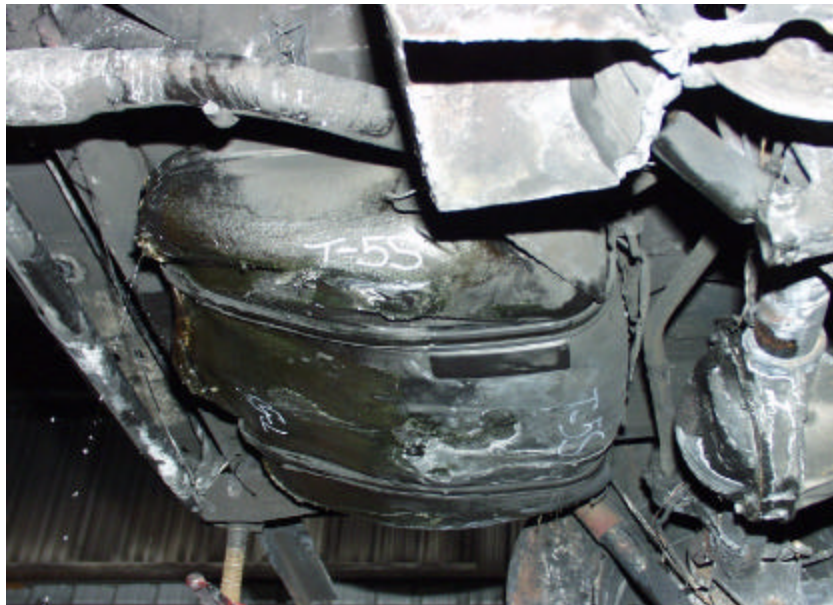
Figure A-122. Test No. 5S, New 1998 Jeep Grand Cherokee Fuel Tank Immediately After Fire Exposure with Heat Shield Removed and Leak Location at Rear Left Corner and Rear Middle of Tank.
