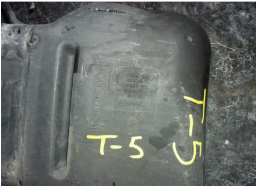
Figure A-134. DaimlerChrysler Manufacturer Imprint on Bottom Side of Conditioned 1998 Plymouth Grand Voyager Fuel Tank.
