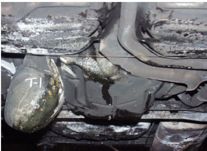
Figure A-189. Test No. 1 (January 21, 2003), New 2000 Chevrolet Cavalier Plastic Fuel Tank Immediately After Fire Exposure with Passenger Side Fuel Tank Sagging.
