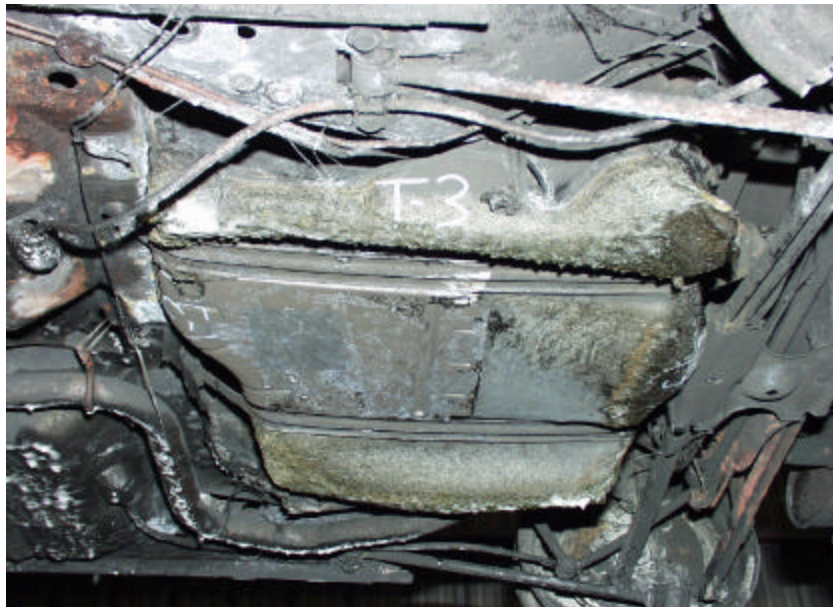
Figure A-82. Test No. 3, Repeatability Evaluation on a New 1998 Saturn Twin Cam 4-Door Fuel Tank Immediately After Fire Exposure with a Leak at Front Left Passenger Side Bottom Corner.
