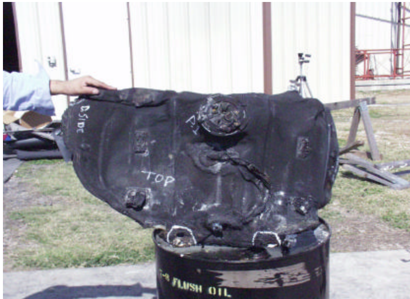
Figure A-190. Test No. 1 (January 21, 2003), Top View of New 2000 Chevrolet Cavalier Plastic Fuel Tank After Fire Exposure.
