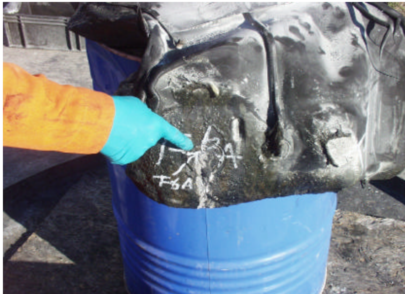
Figure A-154. Test No. 6A, Top Front View of New 1998 Plymouth Grand Voyager Fuel Tank After Fire Exposure at Leak Location.
