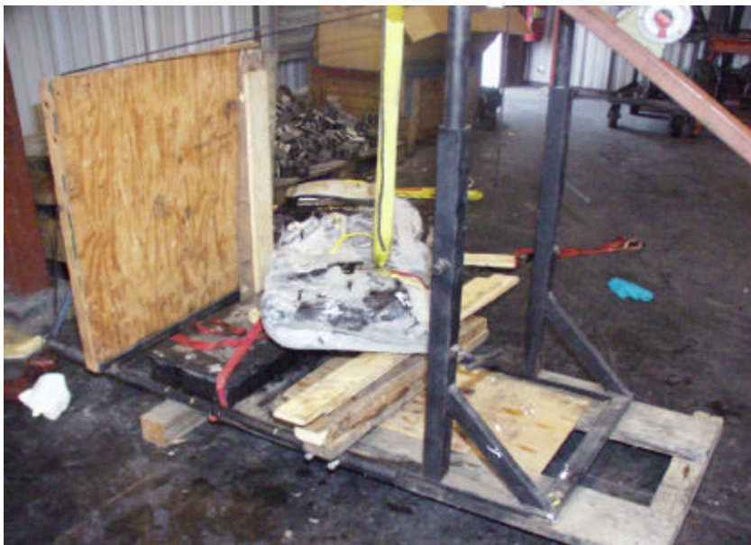
Figure A-223. Front Driver Side of Conditioned 1998 Plymouth Grand Voyager Fuel Tank Prior to Impact.
