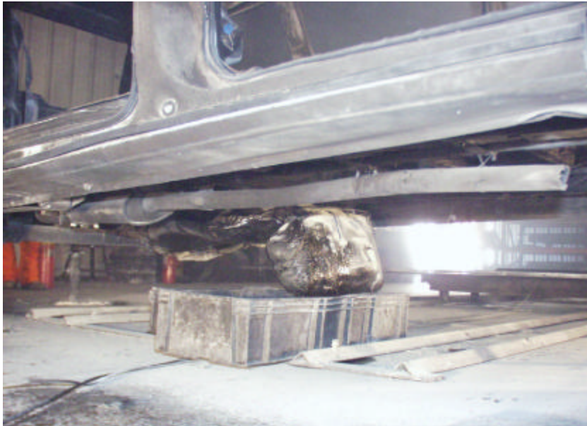
Figure A-147. Test No. 6A, New 1998 Plymouth Grand Voyager Fuel Tank Immediately After Fire Exposure with Leak at Front Strap and Front Top Side of Fuel Tank.
