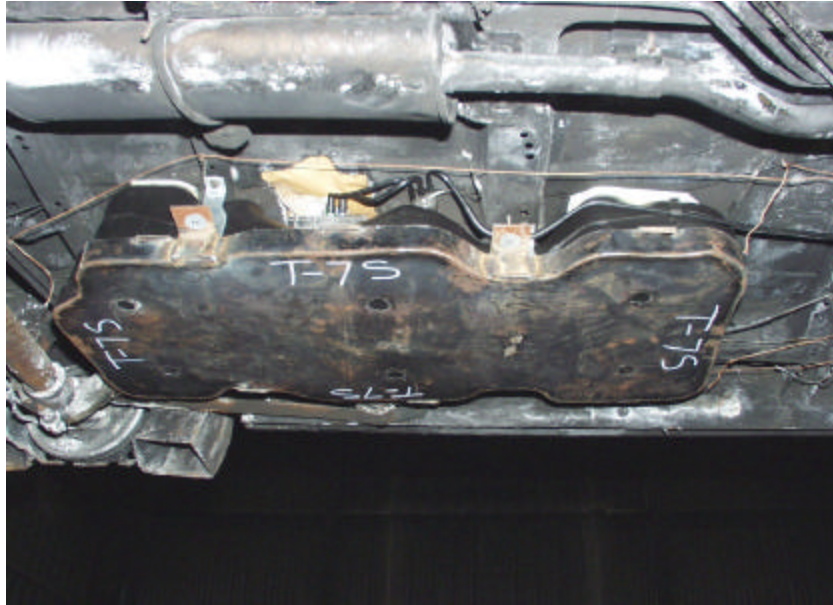
Figure A-163. Test No. 7S, Bottom Side of New 1998 Plymouth Grand Voyager Fuel Tank Assembly With Bottom Heat Shield, Prior to Test.
