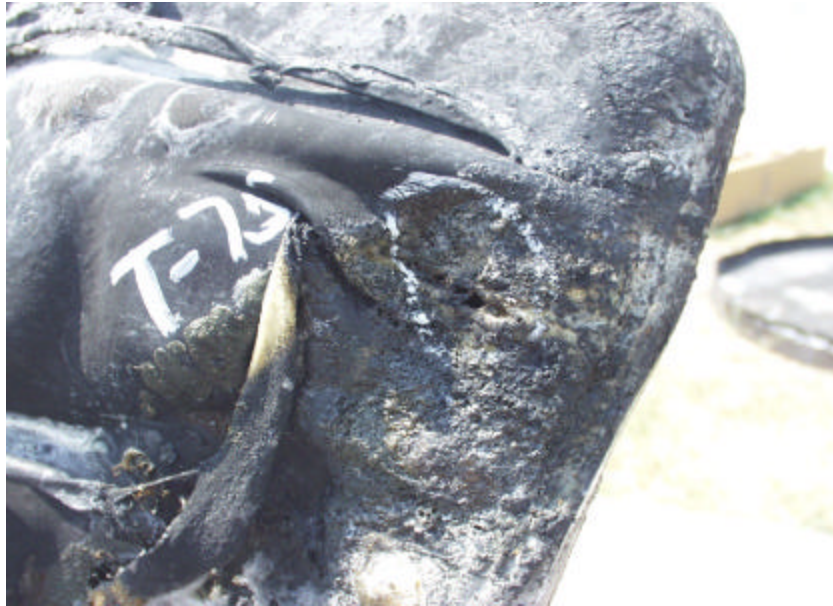
Figure A-181. Test No. 7S, Top View of New 1998 Plymouth Grand Voyager Fuel Tank After Fire Exposure With Leak Location at Top Driver Side of Fuel Tank.
