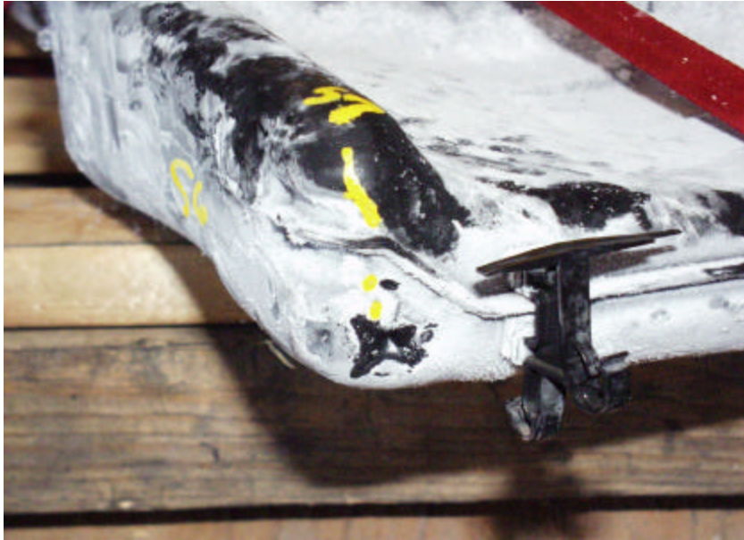
Figure A-206. No Leaks to the Front Driver Side of the Conditioned 1999 Saturn Twin Cam 4-Door Fuel Tank After Two Impacts Ranging Between 43.6 Nm and 147.2 Nm.
