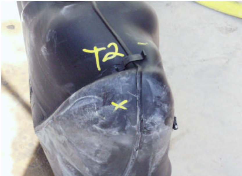
Figure A-236. No Leaks on Front Passenger Side Corner of the New 1998 Plymouth Grand Voyager Fuel Tank After the 30-ft Drop Test.
