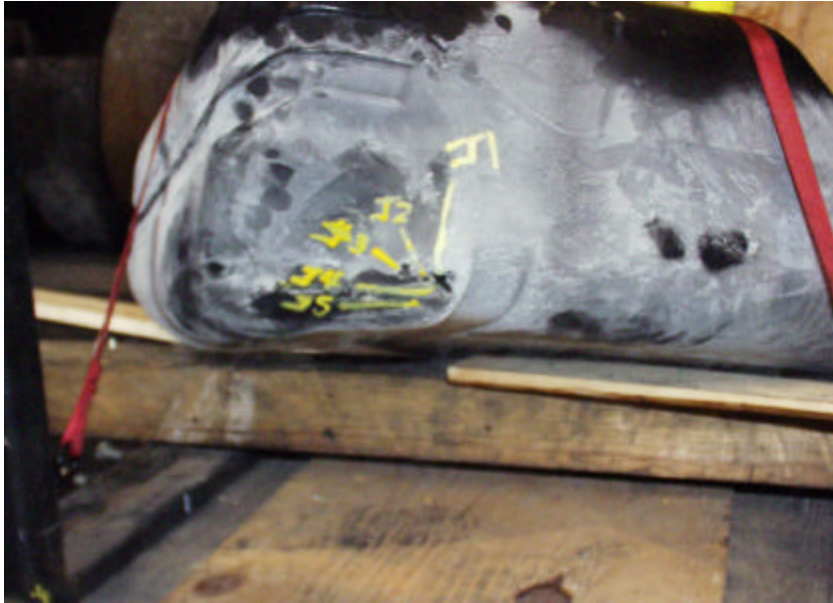
Figure A-212. No Leaks to the Front Passenger Side of the Conditioned 1998 Jeep Grand Cherokee Fuel Tank After Five Impacts Ranging Between 30.1 Nm to 43.6 Nm.
