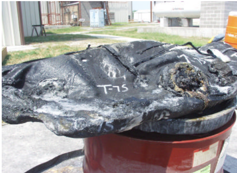
Figure A-182. Test No. 7S, Top View of New 1998 Plymouth Grand Voyager Fuel Tank After Fire Exposure With Leak Location at Rear Corner Passenger Side of Fuel Tank.
