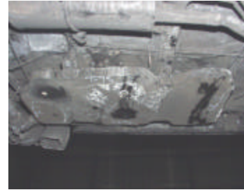
Figure 24. Test PNP2(S) After Exposure Without Shield.
