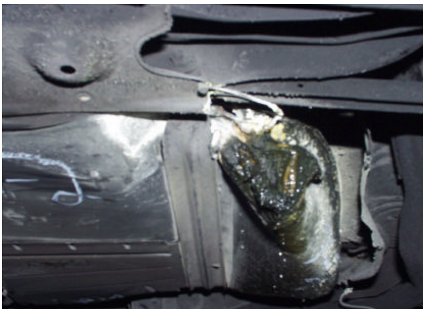
Figure A-74. Test No. 2, Repeatability Evaluation on a New 1998 Saturn Twin Cam 4-Door Fuel Tank Immediately After Fire Exposure with Leak on Rear Passenger Side Corner of Fuel Tank.
