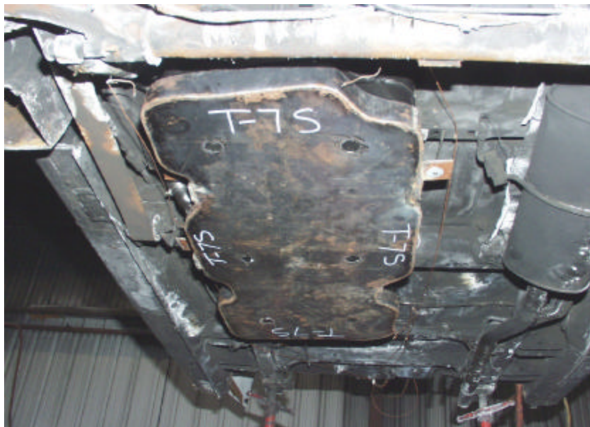
Figure A-162. Test No. 7S, Bottom Side of New 1998 Plymouth Grand Voyager Fuel Tank Assembly With Bottom Heat Shield, Prior to Test.
