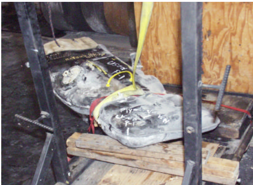
Figure A-218. Front Passenger Side of a 1998 Plymouth Grand Voyager Fuel Tank Prior to Impact.
