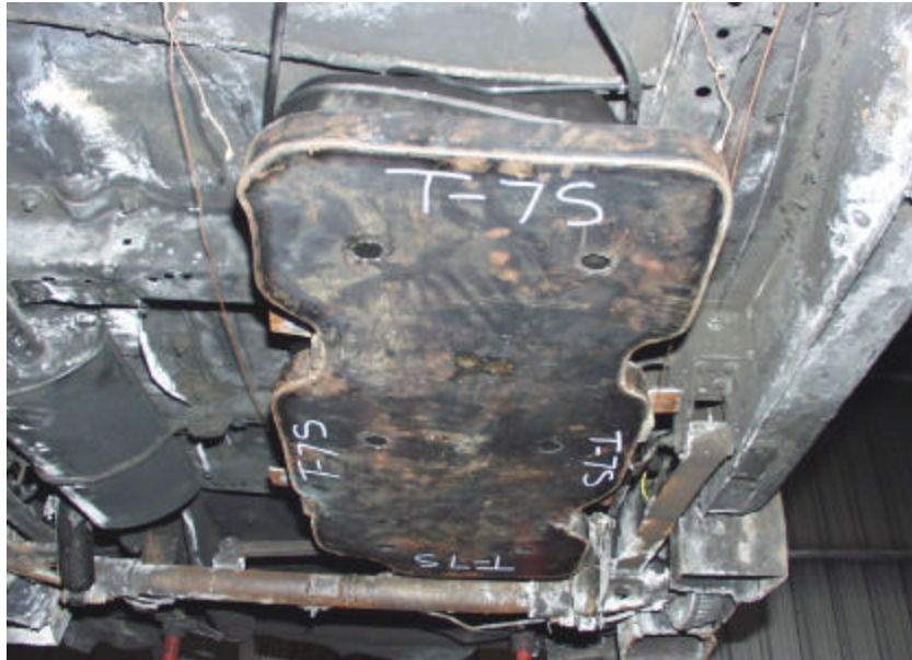
Figure A-161. Test No. 7S, Bottom Side of New 1998 Plymouth Grand Voyager Fuel Tank Assembly With Bottom Heat Shield, Prior to Test.
