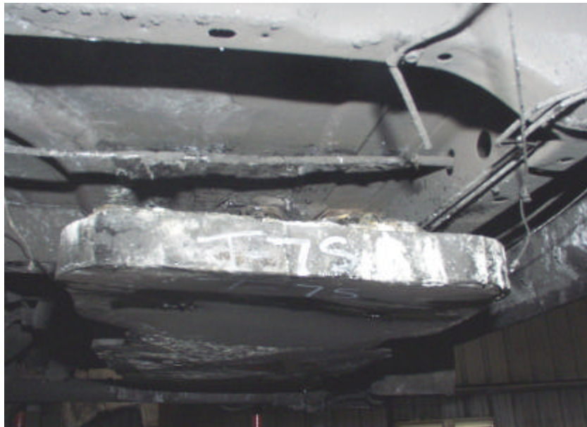
Figure A-168. Test No. 7S, Bottom View Indicating How New 1998 Plymouth Grand Voyager Plastic Fuel Tank Melted Down Into the Heat Shield After Fire Exposure.
