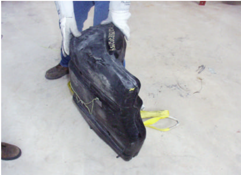
Figure A-227. No Leaks on the Front Passenger Side of the Conditioned 2001 Saturn Fuel Tank After the 30-ft Drop Test.
