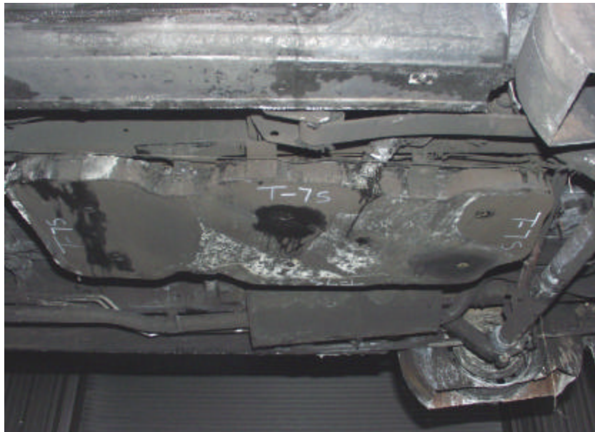
Figure A-166. Test No. 7S, Bottom View of New 1998 Plymouth Grand Voyager Fuel Tank With Heat Shield After Fire Exposure With Leak Location at Front Side and Middle Drain Holes.
