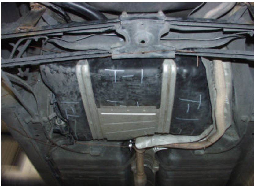
Figure A-46. Test No. 1, Conditioned 1998 Saturn Twin Cam 4-Door Fuel Tank Mounted in Test Platform Prior to Testing.
