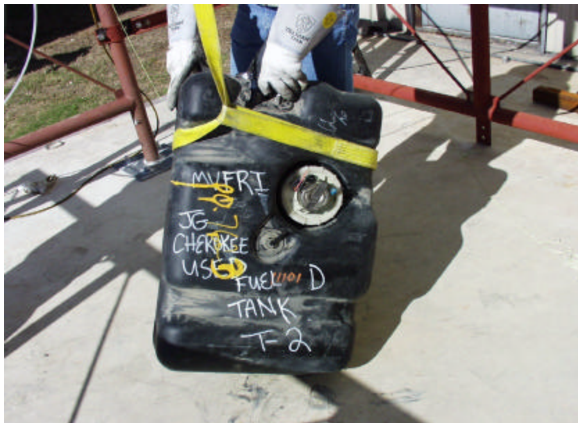
Figure A-240. The Conditioned 1998 Jeep Grand Cherokee Fuel Tank Filled with 17.05 Gallons of Ethylene Glycol Water Mixture (Equal to 23 Gallons of Gasoline) Prior to 30-ft Drop Test on the Front Passenger Side Corner.
