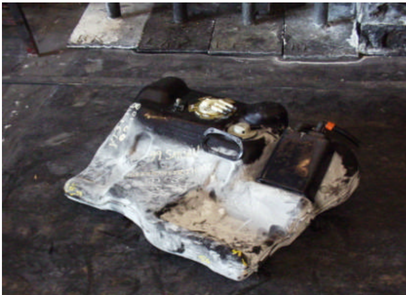
Figure A-203. Impact Resistance Saturn Fuel Tank After Being Conditioned to a -40^{\circ}\text{C} \pm 2^{\circ}\text{C} .
