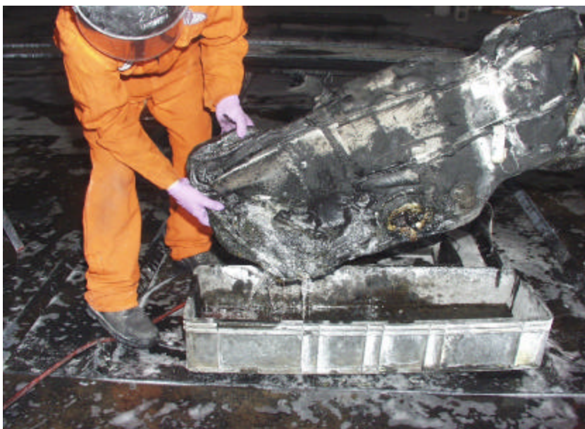
Figure A-175. Test No. 7S, Top View of New 1998 Plymouth Grand Voyager Fuel Tank After Fire Exposure With Leak Location at Rear Corner and Rear Top Driver Side of Fuel Tank.
