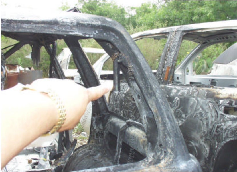
Figure A-131. Test No. 5S, Post-Test Observation of 1998 Jeep Grand Cherokee Lift Gate Strut Support That Vented Loudly During the Test.
