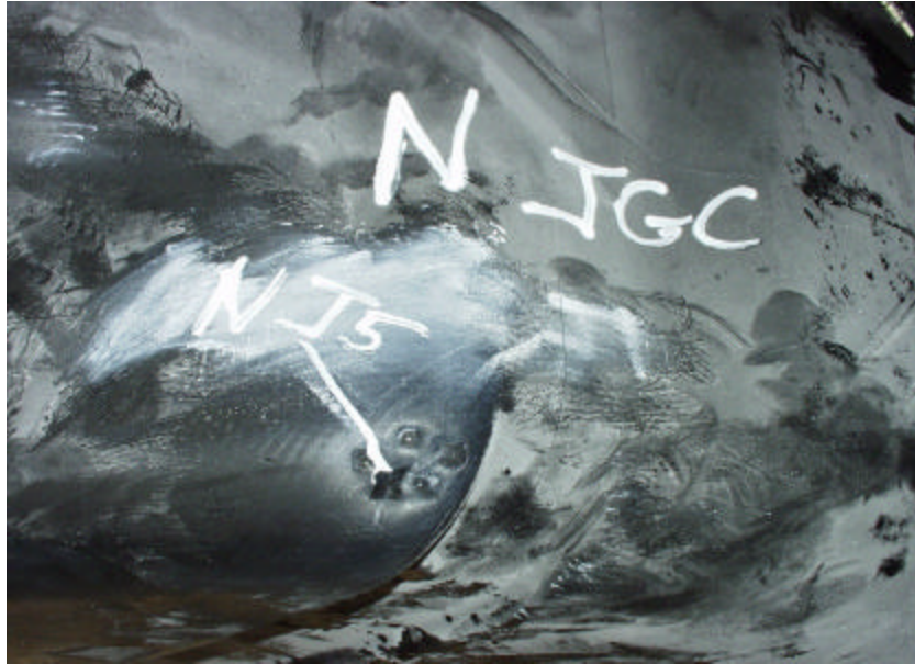
Figure A-216. No Leaks to the Front Passenger Side of the New 1998 Jeep Grand Cherokee Fuel Tank After Five Impacts Ranging Between 30.1 Nm to 43.6 Nm.
