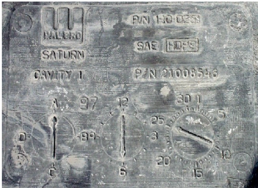
Figure A-43. WALBRO Manufacturer Imprint on Bottom Side of Conditioned 1998 Saturn Twin Cam 4-Door Twin Fuel Tank.
