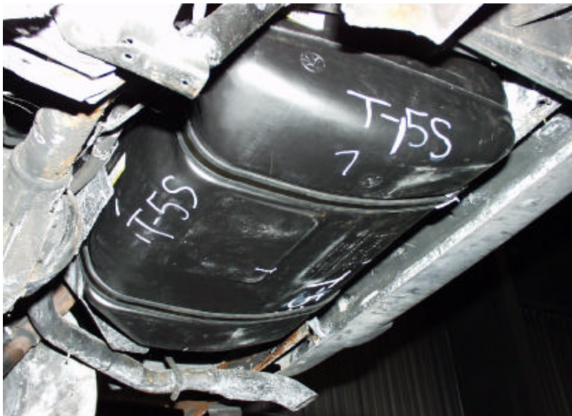
Figure A-114. Test No. 5S, New 1998 Jeep Grand Cherokee Fuel Tank Mounted in Test Platform Prior to Heat Shield and Testing.
