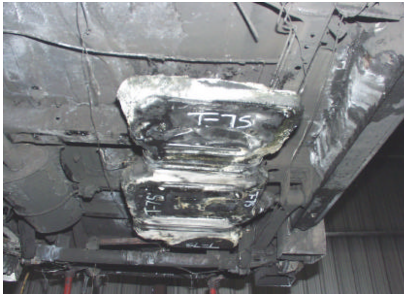
Figure A-169. Test No. 7S, Bottom View of New 1998 Plymouth Grand Voyager Fuel Tank With Heat Shield Removed After Fire Exposure.
