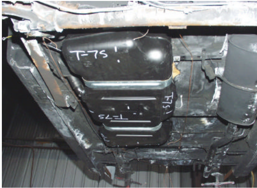
Figure A-159. Test No. 7S, Bottom Side of New 1998 Plymouth Grand Voyager Fuel Tank Assembly Without Bottom Heat Shield, Prior to Test.
