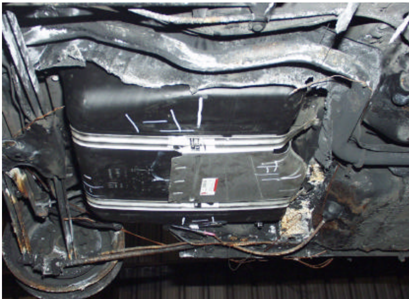
Figure A-63. Test No. 1, Repeatability Evaluation on a New 1998 Saturn Twin Cam 4-Door Fuel Tank Mounted in the Test Platform Prior to Testing.
