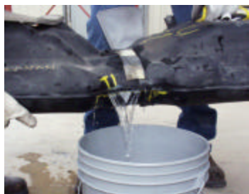
Figure 30. Leakage of Conditioned Plymouth Plastic Fuel Tank After Sever Drop.
