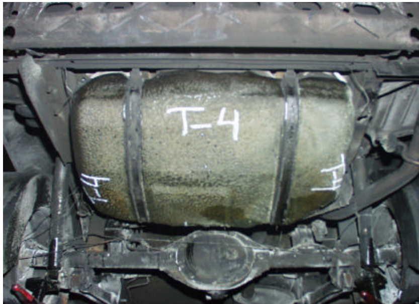
Figure A-105. Test No. 4, New 1998 Jeep Grand Cherokee Fuel Tank Immediately After Fire Exposure with Leak at Front Right Side Bottom of Fuel Tank.
