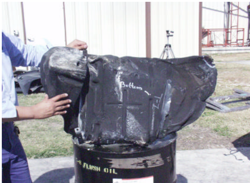
Figure A-191. Test No. 1 (January 21, 2003), Bottom View of New 2000 Chevrolet Cavalier Plastic Fuel Tank After Fire Exposure.
