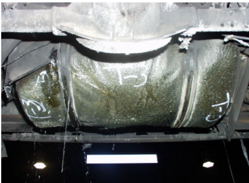
Figure A-94. Test No. 3, Conditioned 1998 Jeep Grand Cherokee Fuel Tank Immediately After Fire Exposure with Leak at Front Right Side Along Outboard Side of Strap.
