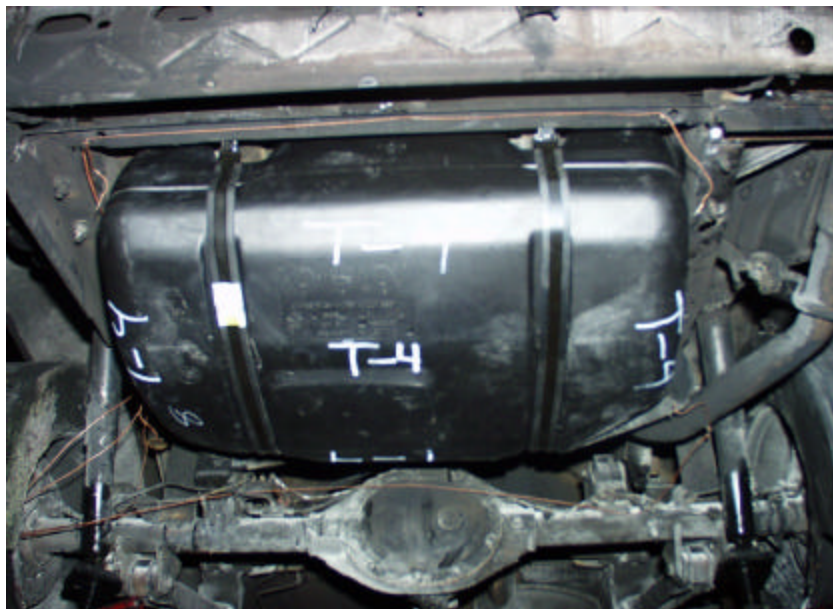
Figure A-104. Test No. 4, New 198 Jeep Grand Cherokee Fuel Tank Mounted in Test Platform Prior to Testing.
