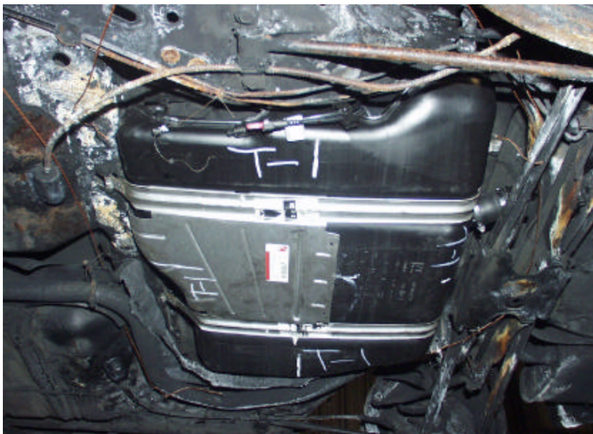
Figure A-64. Test No. 1, Repeatability Evaluation on a New 1998 Saturn Twin Cam 4-Door Fuel Tank Mounted in Test Platform Prior to Testing.
