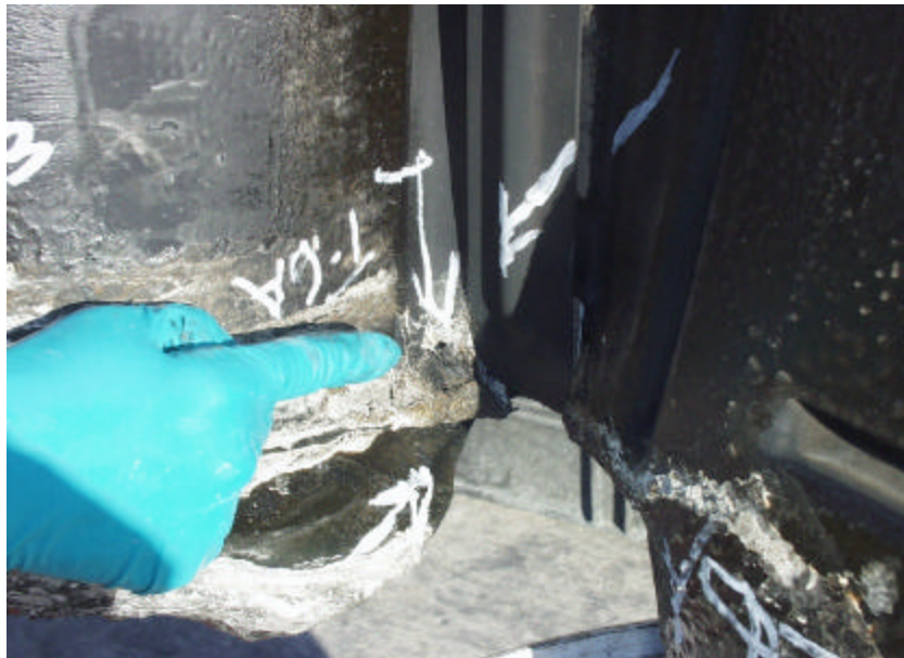
Figure A-152. Test No. 6A, Bottom View of New 1998 Plymouth Grand Voyager Fuel Tank After Fire Exposure at Front Strap Leak Location.
