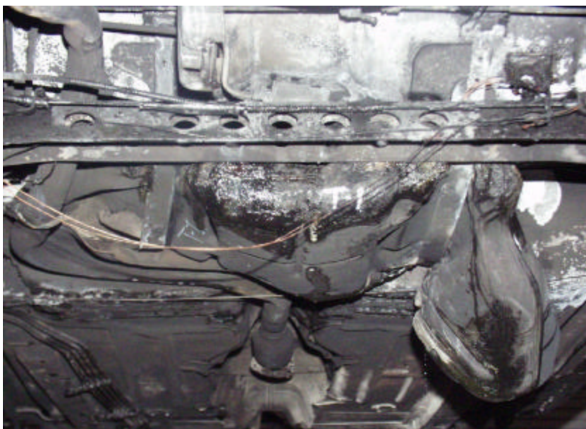
Figure A-188. Test No. 1 (January 21, 2003), New 2000 Chevrolet Cavalier Plastic Fuel Tank Immediately After Fire Exposure with Passenger Side of Fuel Tank Sagging.
