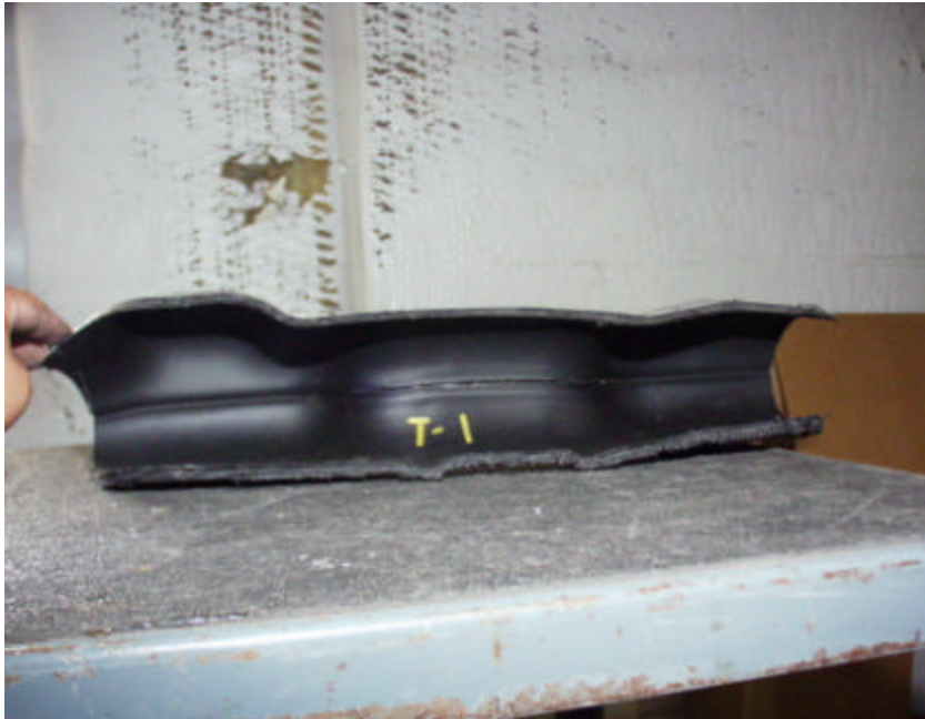
Figure A-33. Internal View of Plymouth Tank Pinch-Off Section.
