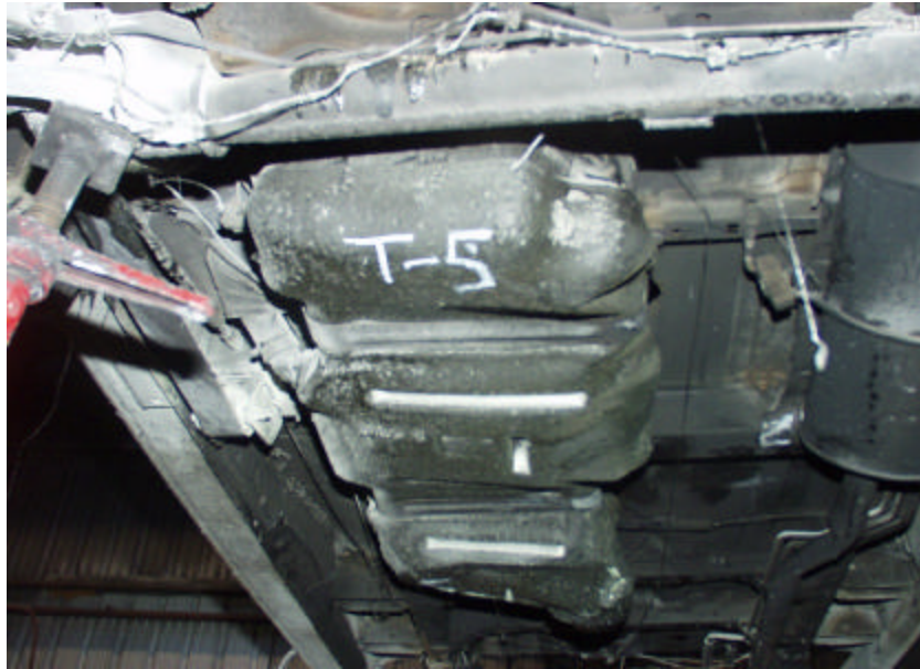
Figure A-139. Test No. 5 Conditioned 1998 Plymouth Grand Voyager Fuel Tank Immediately After Fire Exposure with Leak at Front Right Bottom Corner of Fuel Tank.
