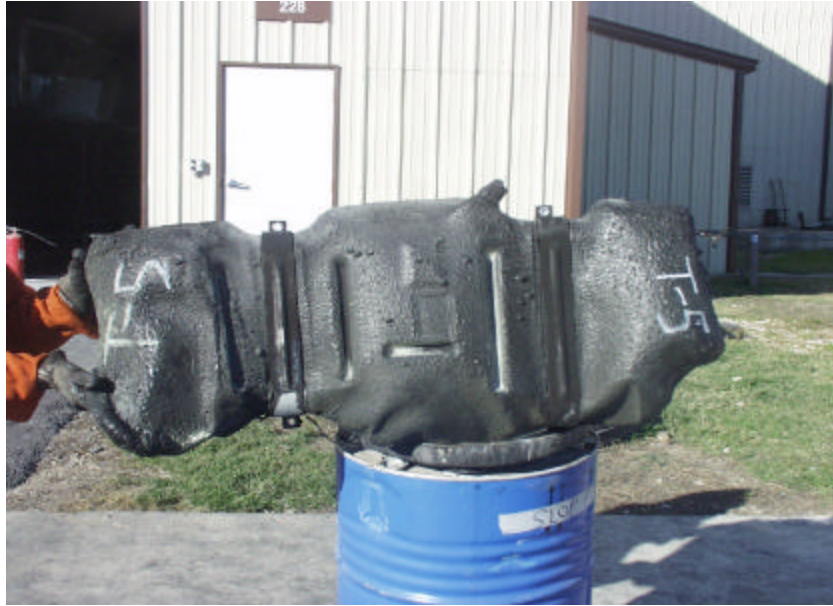
Figure A-141. Test No. 5, Bottom View of Conditioned 1998 Plymouth Grand Voyager Fuel Tank After Fire Exposure.
