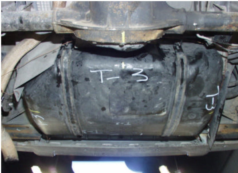
Figure A-92. Test No. 3, Conditioned 1998 Jeep Grand Cherokee Fuel Tank Mounted in Test Platform Prior to Testing.
