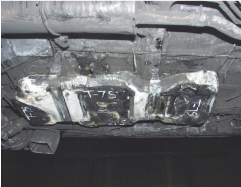
Figure A-23. Test PNP2(S) After Exposure With Tank Shield.
