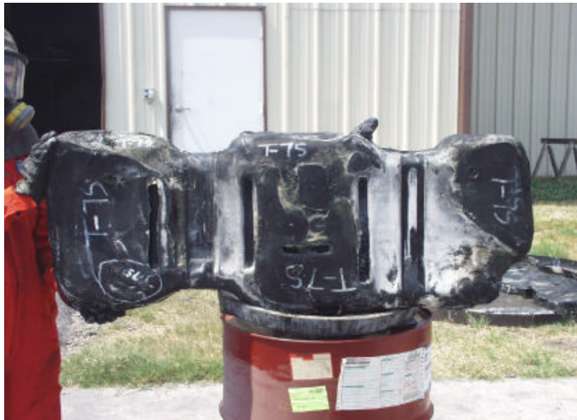
Figure A-178. Test No. 7S, Bottom View of New 1998 Plymouth Grand Voyager Fuel Tank After Fire Exposure With Leak Location at Front Bottom Passenger Side of Fuel Tank.
