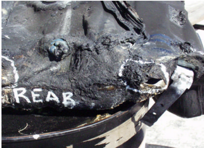
Figure A-194. Test No. 1 (January 21, 2003), Passenger Side Fire Exposure Hole, Rear Topside of New 2000 Chevrolet Cavalier Plastic Fuel Tank.
