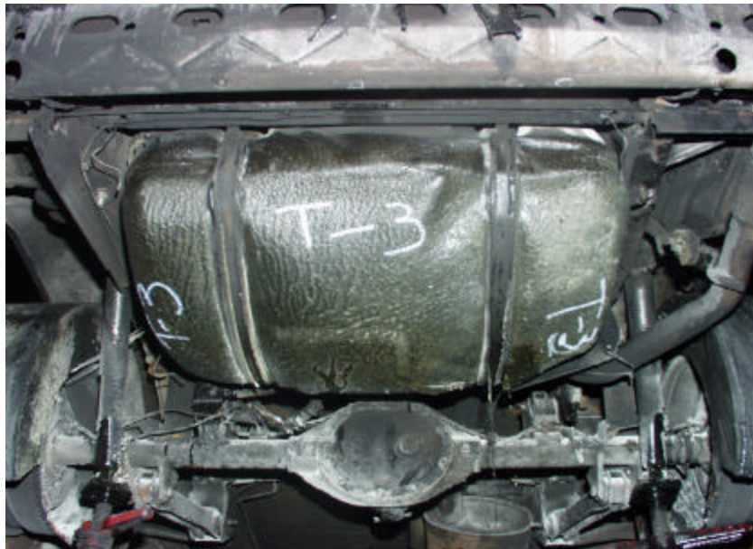
Figure A-96. Test No. 3, Conditioned 1998 Jeep Grand Cherokee Fuel Tank Immediately After Fire Exposure with Leak at Front Right Side Along Outboard Side of Strap.
