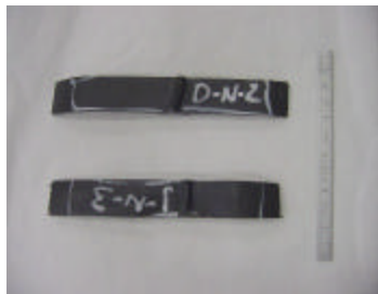
Figure 37. Typical Tensile Test Specimen Coupon.
