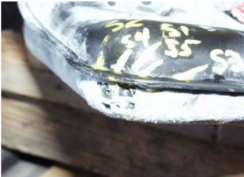
Figure A-205. No Leaks to the Front Passenger Side of the Conditioned 1999 Saturn Twin Cam 4-Door Fuel Tank After Five Impacts Ranging Between 30.1 Nm to 43.6 Nm.
