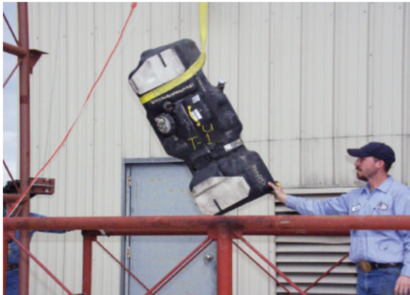
Figure A-231. The Conditioned 2000 Plymouth Grand Voyager Fuel Tank Filled with 14.83 Gallons of Ethylene Glycol Water Mixture (Equal to 20 Gallons of Gasoline) Prior to 30-ft Drop Test of the Front Passenger Side Corner.
