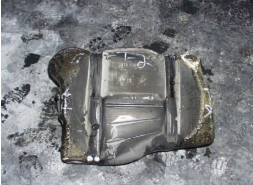
Figure A-77. Test No. 2, Repeatability Evaluation on a New 1998 Saturn Twin Cam 4-Door Fuel Tank After Fire Exposure, Bottom View.
