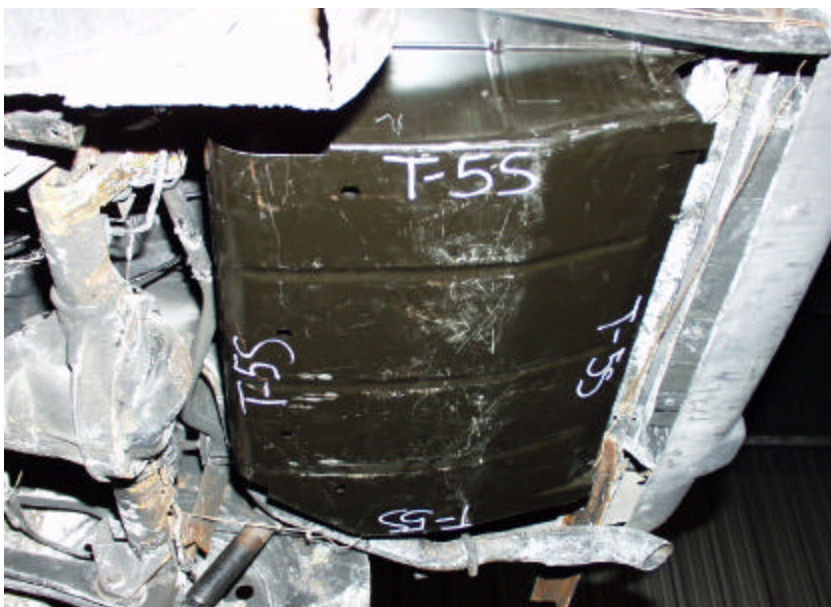
Figure A-116. Test No. 5S, New 1998 Jeep Grand Cherokee Fuel Tank Mounted in Test Platform with Heat Shield, Prior to Testing.
