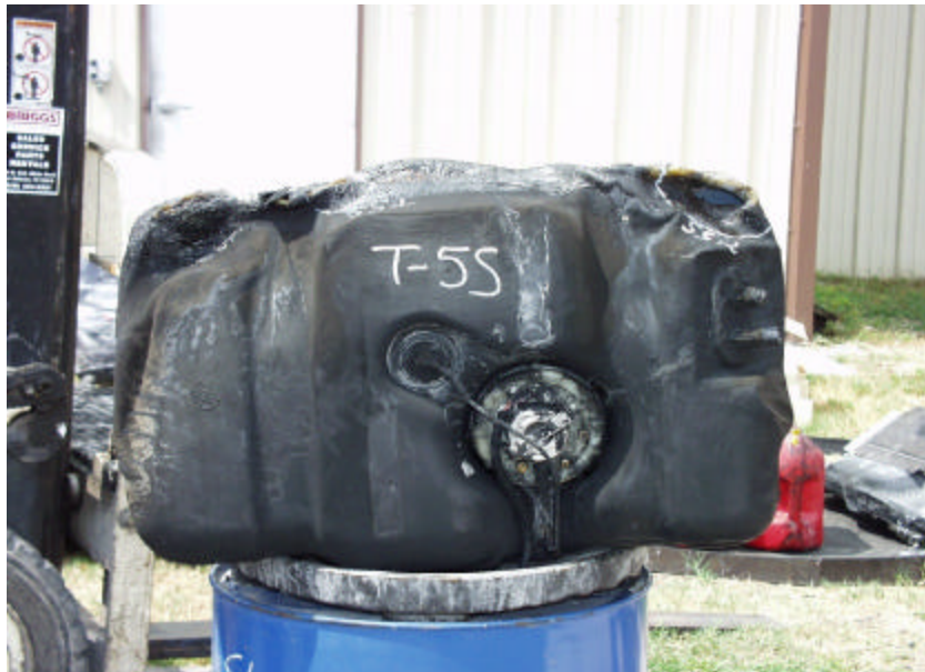
Figure A-126. Test No. 5S, Top View of New 1998 Jeep Grand Cherokee Fuel Tank After Fire Exposure.
