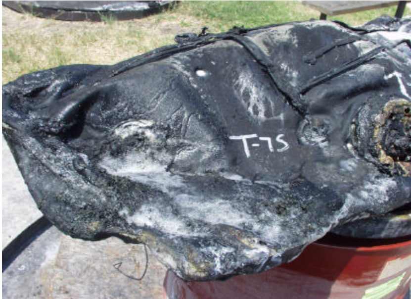
Figure A-183. Test No. 7S, Top View of New 1998 Plymouth Grand Voyager Fuel Tank After Fire Exposure With Leak Location at Rear Corner Passenger Side of Fuel Tank.
