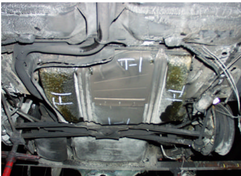
Figure A-47. Test No. 1, Conditioned 1998 Saturn Twin Cam 4-Door Fuel Tank Immediately After Fire Exposure.
