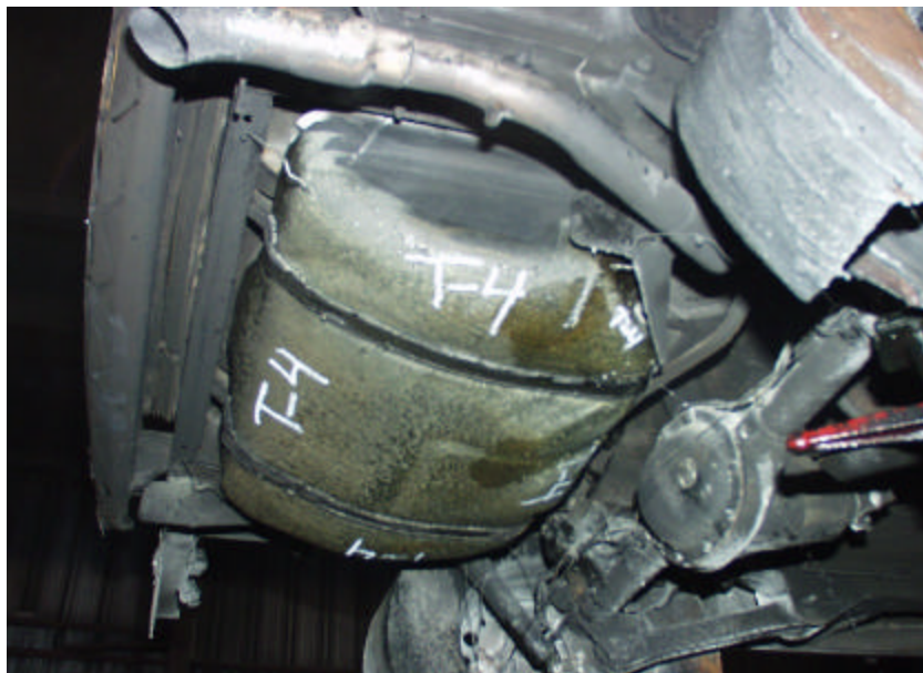
Figure A-106. Test No. 4, New 1998 Jeep Grand Cherokee Fuel Tank Immediately After Fire Exposure with Leak at Front Right Side Bottom of Fuel Tank.
