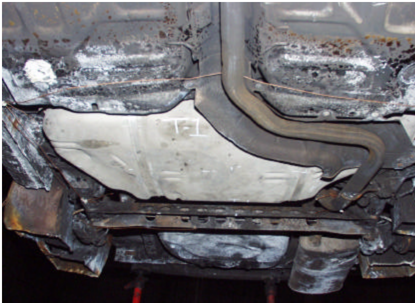
Figure A-196. Test No. 1 (February 18, 2003), Conditioned 1999 Chevrolet Cavalier Metal Fuel Tank Assembly Mounted in Test Platform Prior to Testing.
