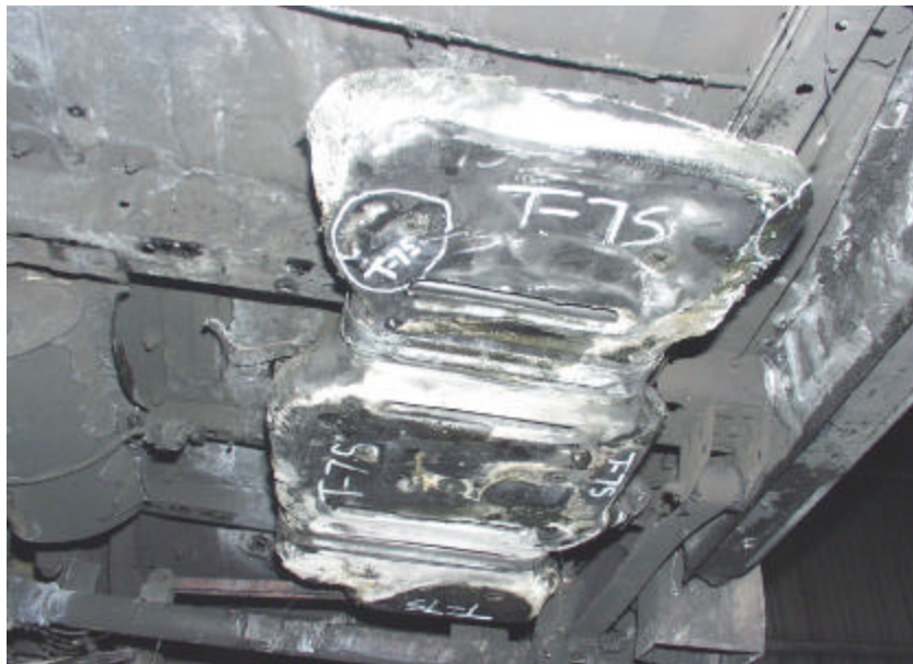
Figure A-174. Test No. 7S, Bottom View of New 1998 Plymouth Grand Voyager Fuel Tank With Heat Shield Removed After Fire Exposure With Leak Location at Front Bottom Passenger Side of Fuel Tank.
