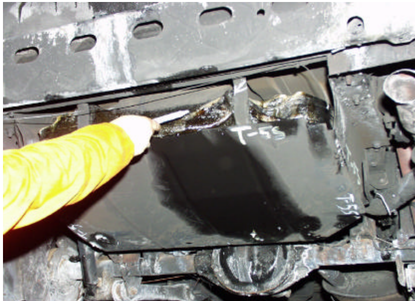
Figure A-120. Test No. 5S, New 1998 Jeep Grand Cherokee Fuel Tank Immediately After Fire Exposure with Heat Shield and Leak Location at Rear Middle of Tank.
