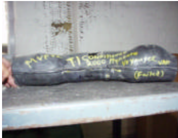
Figure 32. External View of Plymouth Tank Pinch-Off Section
