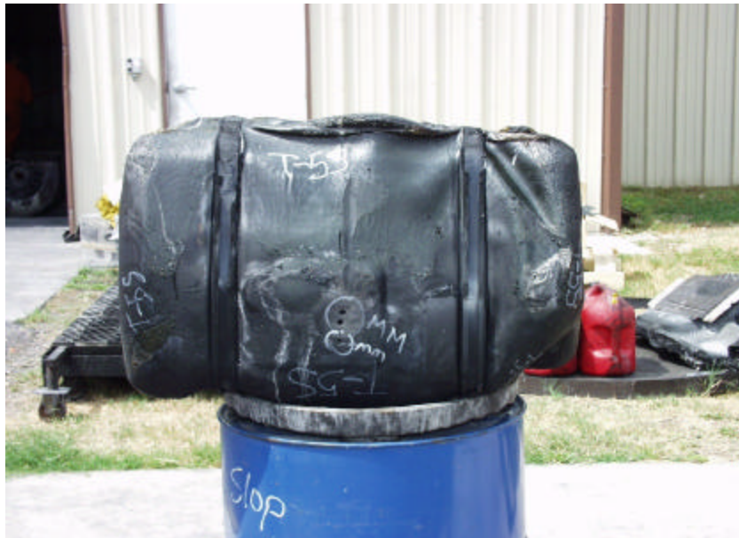
Figure A-127. Test No. 5S, Bottom View of New 1998 Jeep Grand Cherokee Fuel Tank After Fire Exposure.
