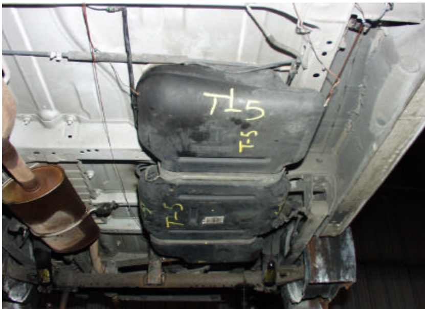
Figure A-136. Test No. 5, Conditioned 1998 Plymouth Grand Voyager Fuel Tank Mounted in Test Platform Prior to Testing.
