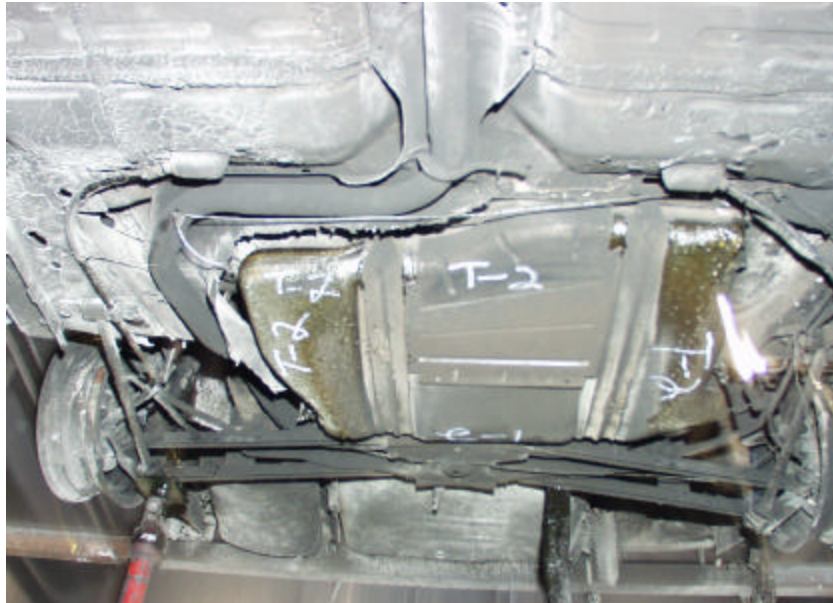
Figure A-56. Test No. 2, New 1998 Saturn Twin Cam 4-Door Fuel Tank Immediately After Fire Exposure.
