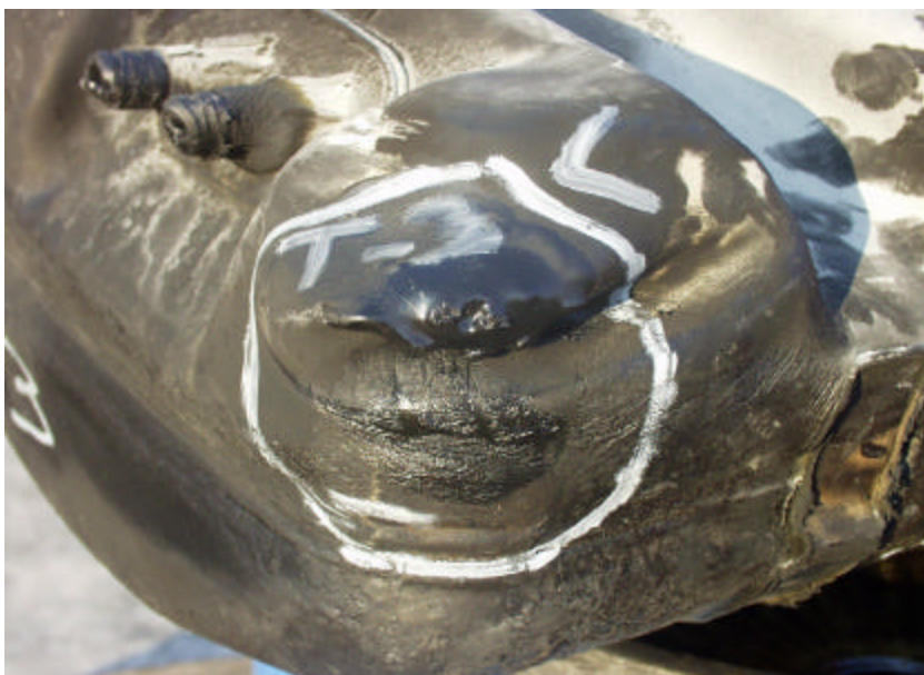
Figure A-100. Test No. 3, Fire Exposure Hole at Front Right Side Top Corner of Conditioned 1998 Jeep Grand Cherokee Fuel Tank.
