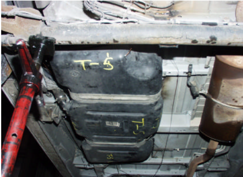
Figure A-137. Test No. 5, Conditioned 1998 Plymouth Grand Voyager Fuel Tank Mounted in Test Platform Prior to Testing.
