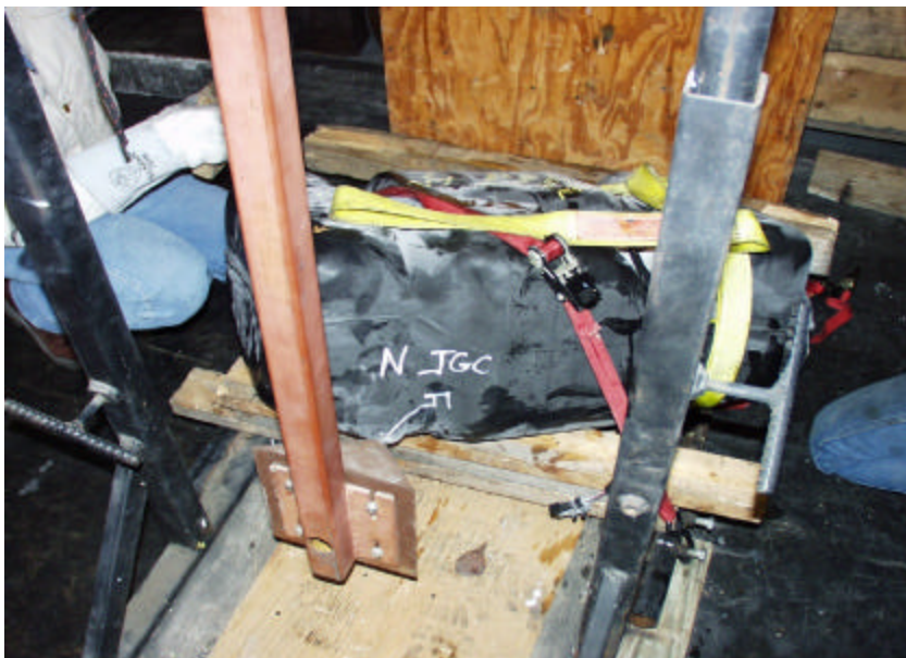
Figure A-215. Front Passenger Side of the New 1998 Jeep Grand Cherokee Fuel Tank Prior to Impact.
