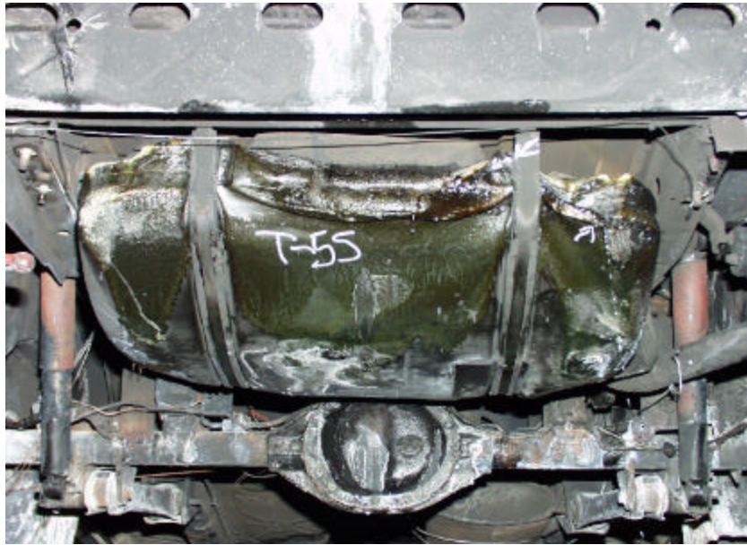
Figure A-123. Test No. 5S, New 1998 Jeep Grand Cherokee Fuel Tank Immediately After Fire Exposure with Heat Shield Removed and Leak Location at Rear Left Corner and Rear Middle of Tank.
