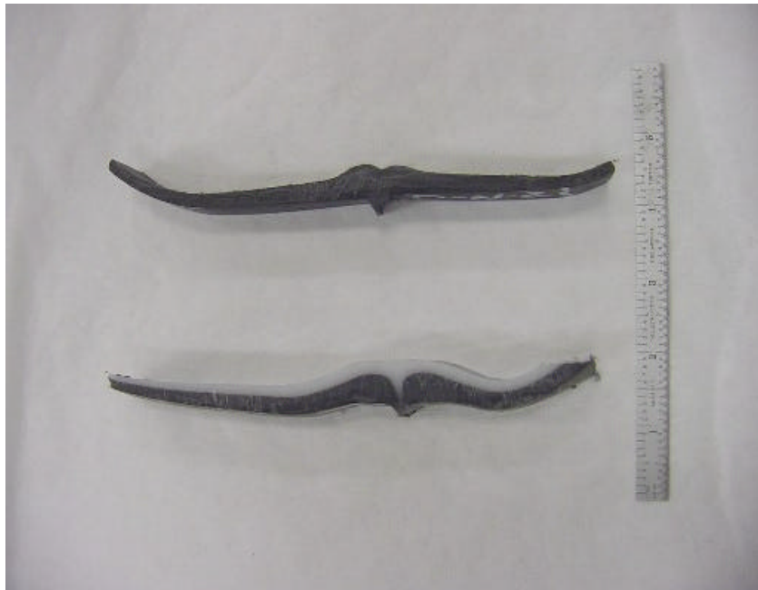
Figure A-38. Thickest Region at Pinch-Off Location.
