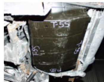
Figure 16. Test JNP2(S) Before Exposure With Skid-Plate.
