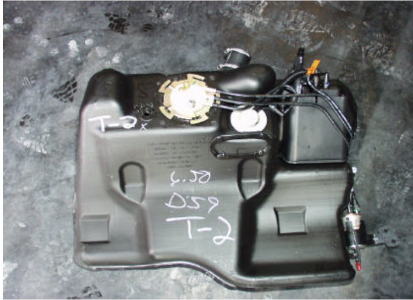
Figure A-52. New 1998 Saturn Twin Cam 4-Door Fuel Tank Assembly.
