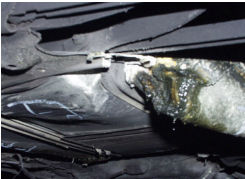
Figure A-75. Test No. 2, Repeatability Evaluation on a New 1998 Saturn Twin Cam 4-Door Fuel Tank Immediately After Fire Exposure with Leak on Rear Passenger Side Corner of Fuel Tank.
