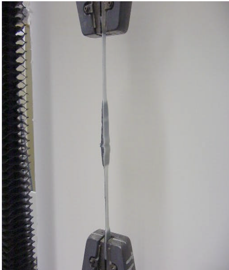
Figure A-40. Elongation of Parent Material.
