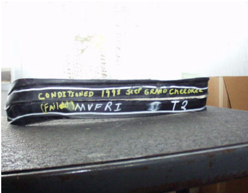
Figure A-34. External View of Jeep Tank Pinch-Off Section.
