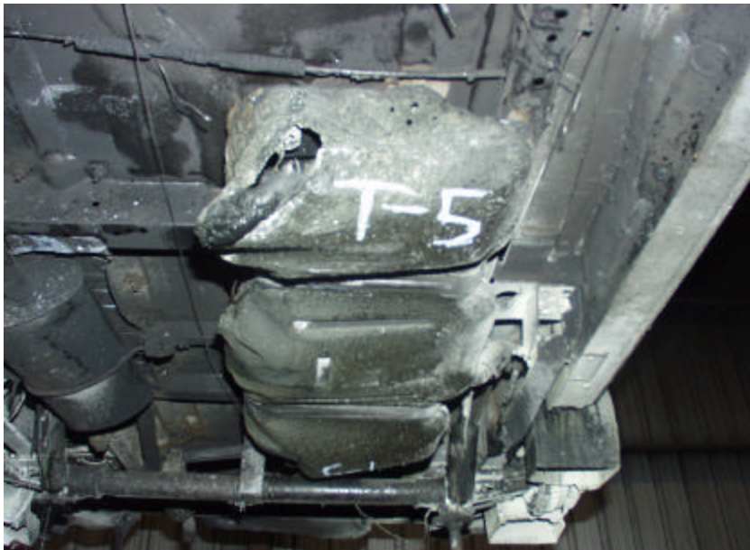
Figure A-138. Test No. 5, Conditioned 1998 Plymouth Grand Voyager Fuel Tank Immediately After Fire Exposure with Leak at Front Right Bottom Corner of Fuel Tank.
