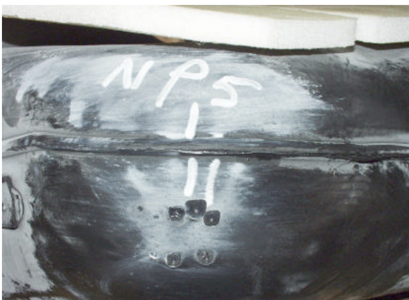
Figure A-219. No Leaks to the Front Passenger Side of the New 1998 Plymouth Grand Voyager Fuel Tank After Five Impacts Ranging Between 30.1 Nm to 43.6 Nm.
