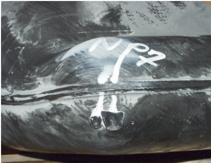
Figure A-28. New Plymouth Plastic Fuel Tank After Impact.
