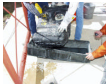
Figure 31. Leakage of Conditioned Jeep Grand Cherokee Fuel Tank After Sever Drop.
