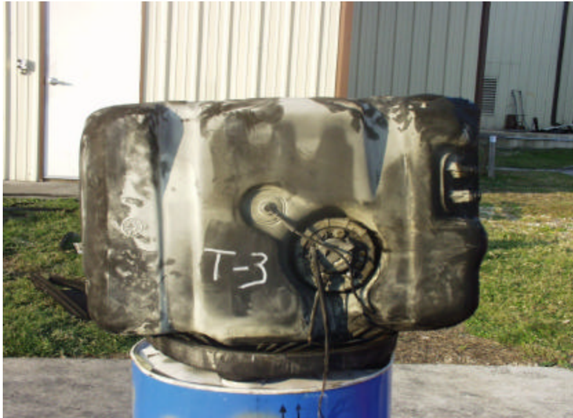
Figure A-97. Test No. 3, Top View of Conditioned 1998 Jeep Grand Cherokee Fuel Tank After Fire Exposure.
