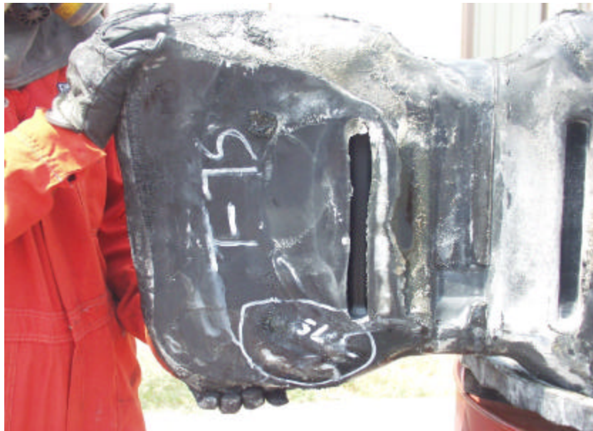
Figure A-179. Test No. 7S, Bottom View of New 1998 Plymouth Grand Voyager Fuel Tank After Fire Exposure With Leak Location at Front Bottom Passenger Side of Fuel Tank.
