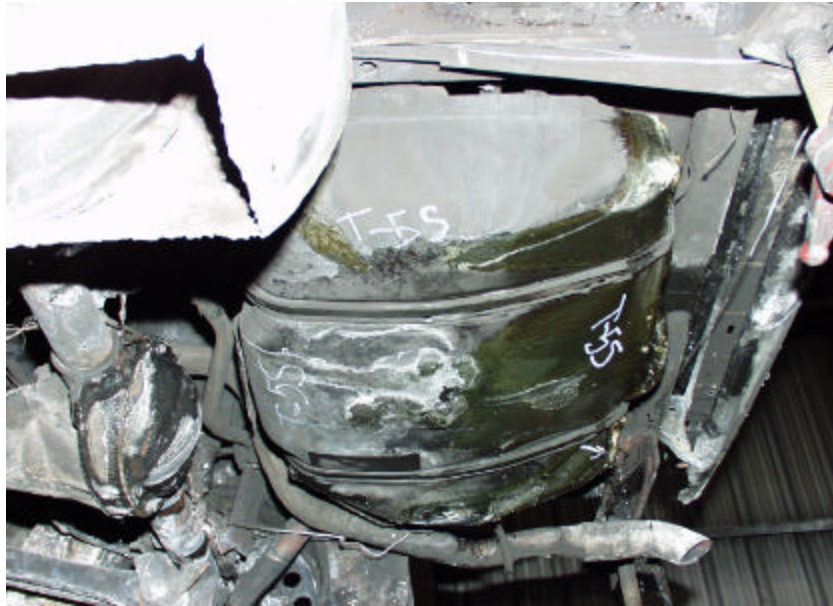
Figure A-121. Test No. 5S, New 1998 Jeep Grand Cherokee Fuel Tank Immediately After Fire Exposure with Heat Shield Removed and Leak Location at Rear Left Corner and Rear Middle of Tank.
