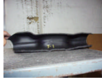
Figure 33. Internal View of Plymouth Tank Pinch-Off Section
