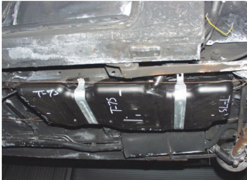
Figure A-160. Test No. 7S, Bottom Side of New 1998 Plymouth Grand Voyager Fuel Tank Assembly Without Bottom Heat Shield, Prior to Test.
