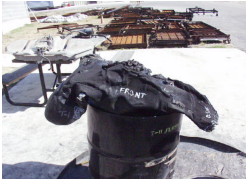
Figure A-192. Test No. 1 (January 21, 2003), Front Side View of New 2000 Chevrolet Cavalier Plastic Fuel Tank After Fire Exposure.
