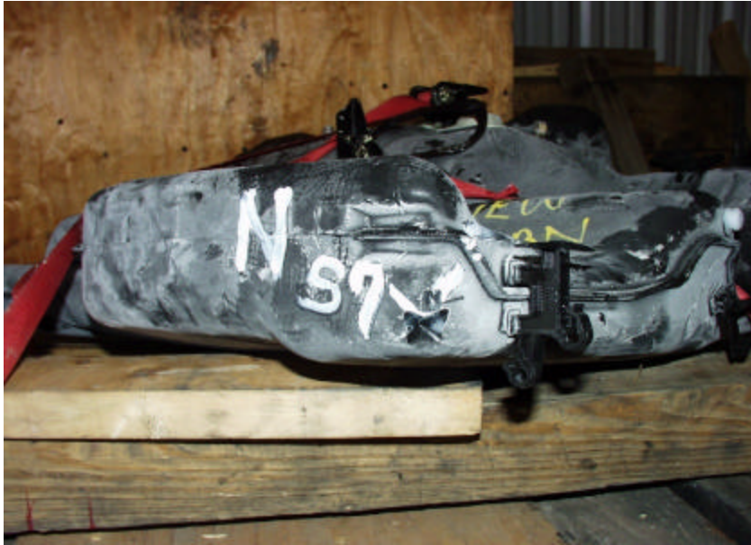
Figure A-210. No Leaks to the Front Driver Side of the New 1998 Saturn Twin Cam 4-Door Fuel Tank After Two Impacts Ranging Between 43.6 Nm and 147.2 Nm.
