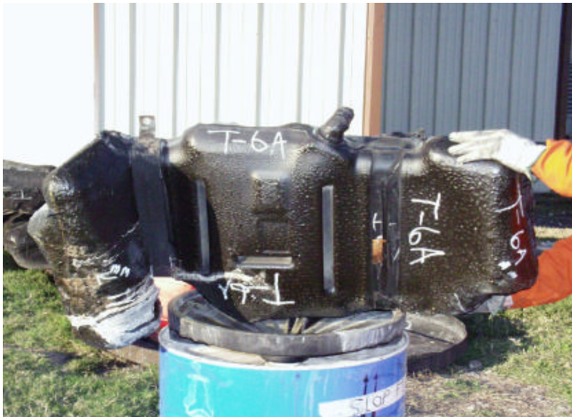
Figure A-150. Test No. 6A, Bottom View of New 1998 Plymouth Grand Voyager Fuel Tank After Fire Exposure.
