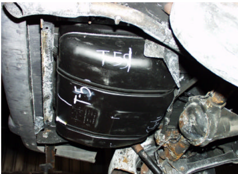
Figure A-115. Test No. 5S, New 1998 Jeep Grand Cherokee Fuel Tank Mounted in Test Platform with Heat Shield, Prior to Testing.
