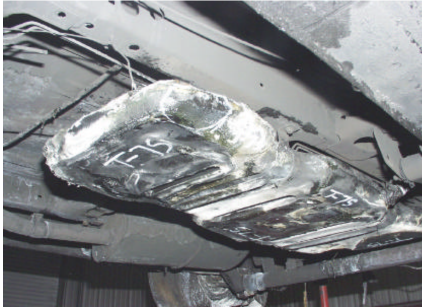
Figure A-173. Test No. 7S, Bottom View of New 1998 Plymouth Grand Voyager Fuel Tank With Heat Shield Removed After Fire Exposure With Leak Location at Front Driver Side Corner of Fuel Tank.
