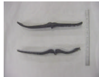
Figure 38. Thickest Region at Pinch-Off Location.
