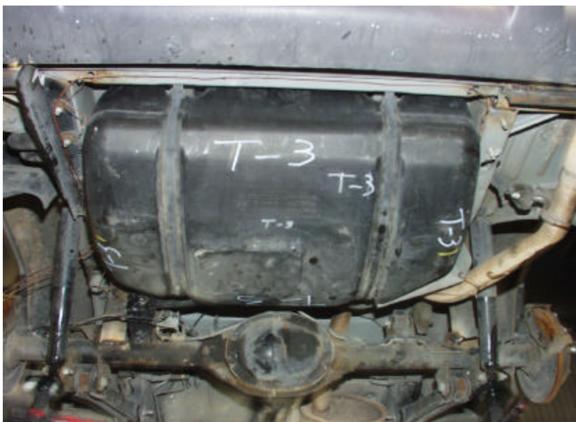
Figure A-93. Test No. 3, Conditioned 1998 Jeep Grand Cherokee Fuel Tank Mounted in Test Platform Prior to Testing.
