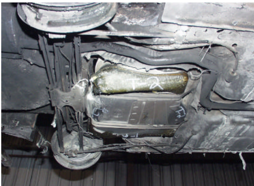
Figure A-73. Test No. 2, Repeatability Evaluation on a New 1998 Saturn Twin Cam 4-Door Fuel Tank Immediately After Fire Exposure with a Leak on Rear Passenger Side Corner of Fuel Tank.
