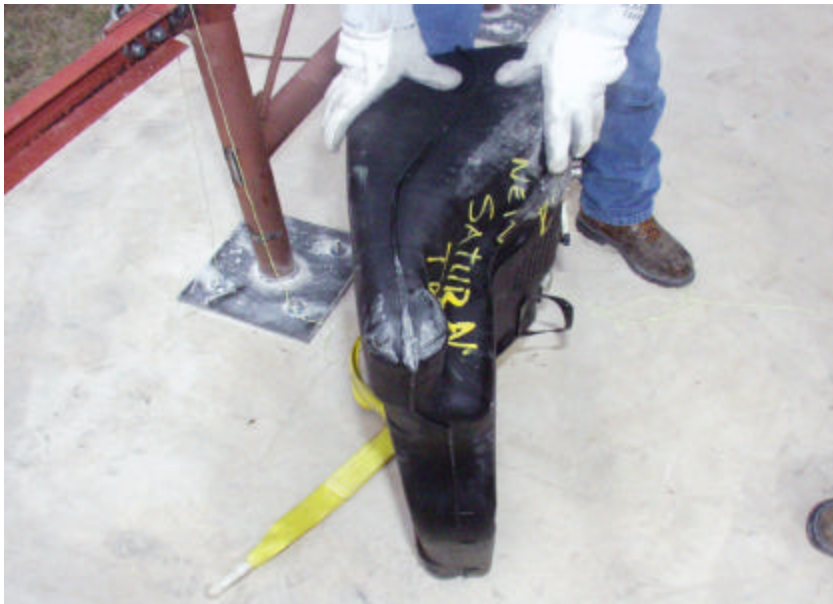
Figure A-230. No Leaks on the Front Passenger Side Corner of the New 1998 Saturn Fuel Tank After the 30-ft Drop Test.
