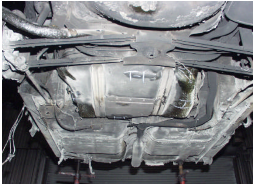
Figure A-66. Test No. 1, Repeatability Evaluation on a New 1998 Saturn Twin Cam 4-Door Fuel Tank with No Leaks; Classified as a Non-Failed Test.
