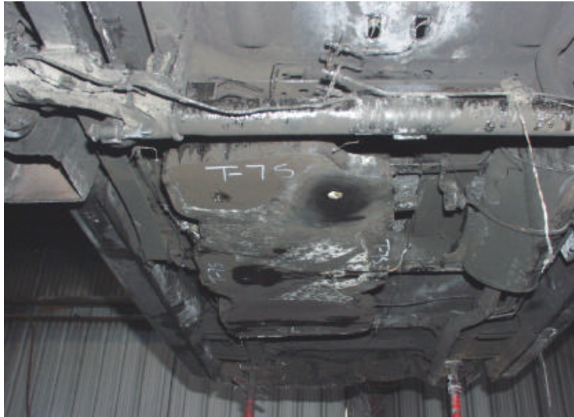
Figure A-165. Test No. 7S, Bottom View of New 1998 Plymouth Grand Voyager Fuel Tank With Heat Shield After Fire Exposure With Leak Location at Front Side and Middle Drain Holes.
