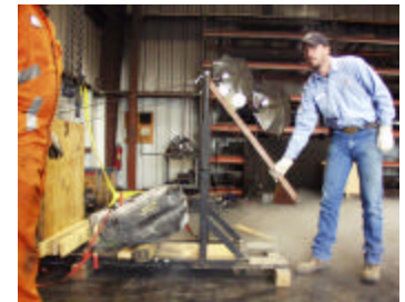
Figure 27. Impact Resistance Test Setup.
