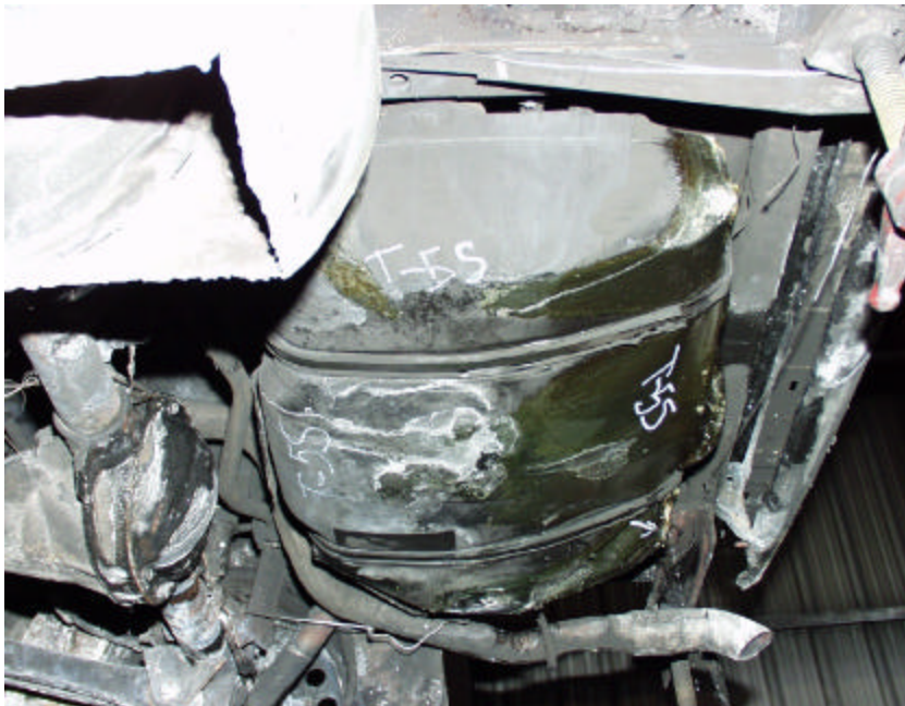
Figure A-18. Test JNP2(S) After Exposure Without Skid-Plate.
