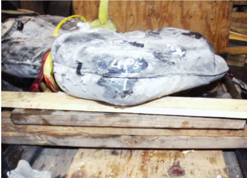
Figure A-222. No Leaks to the Front Passenger Side of the Conditioned 1998 Plymouth Grand Voyager Fuel Tank After Five Impacts Ranging Between 30.1 Nm to 43.6 Nm.
