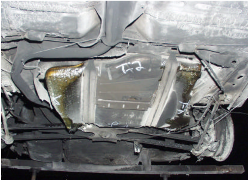
Figure A-71. Test No. 2, Repeatability Evaluation on a New 1998 Saturn Twin Cam 4-Door Fuel Tank Immediately After Fire Exposure with a Leak on Rear Passenger Side Corner of Fuel Tank.
