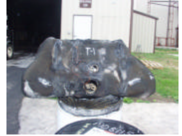
Figure 26. Conditioned Metal Fuel Tank After Exposure.
