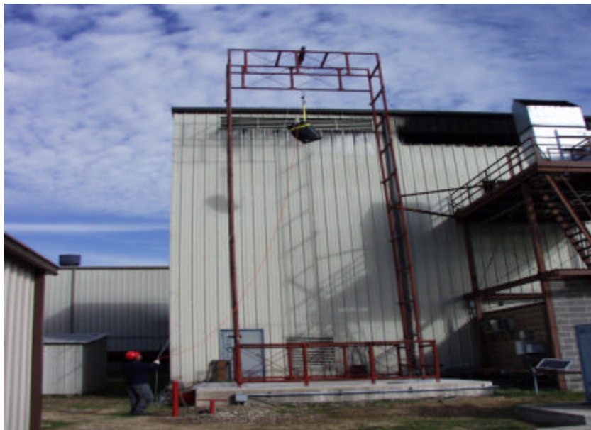
Figure A-238. The New 1998 Jeep Grand Cherokee Fuel Tank at 30-ft Elevation.
