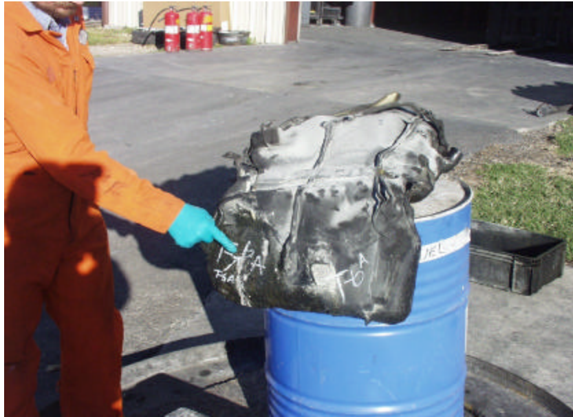
Figure A-153. Test No. 6A, Front Top View of New 1998 Plymouth Grand Voyager Fuel Tank After Fire Exposure at Leak Location.
