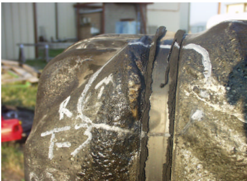
Figure A-99. Test No. 3, Fire Exposure Hole at Front Right Side Along Outside of Strap of Conditioned 1998 Jeep Grand Cherokee Fuel Tank.
