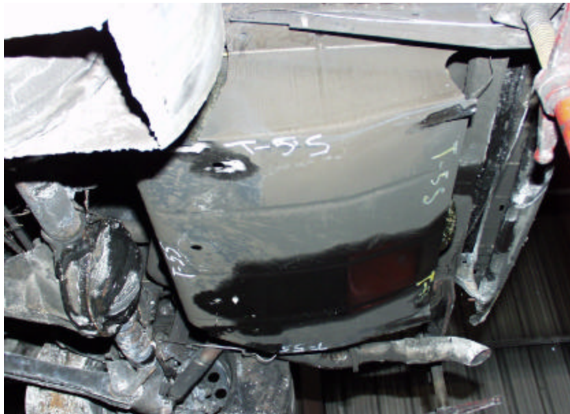
Figure A-118. Test No. 5S, New 1998 Jeep Grand Cherokee Fuel Tank Immediately After Fire Exposure with Heat Shield and Leak Location at Rear of Tank.
