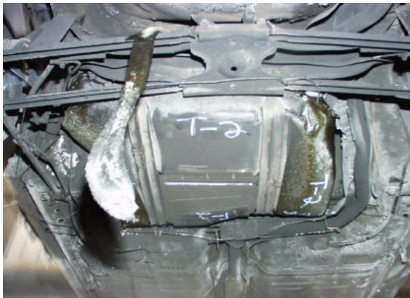
Figure A-57. Test No. 2, New 1998 Saturn Twin Cam 4-Door Fuel Tank Immediately After Fire Exposure.
