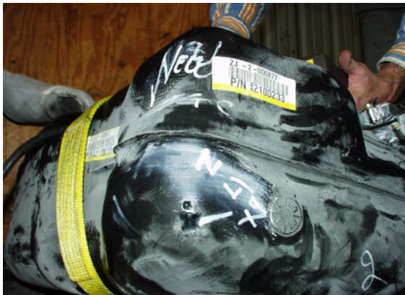
Figure A-217. No Leaks to the Front Driver Side of the New 1998 Jeep Grand Cherokee Fuel Tank After Two Impacts Ranging Between 43.6 Nm and 147.2 Nm.
