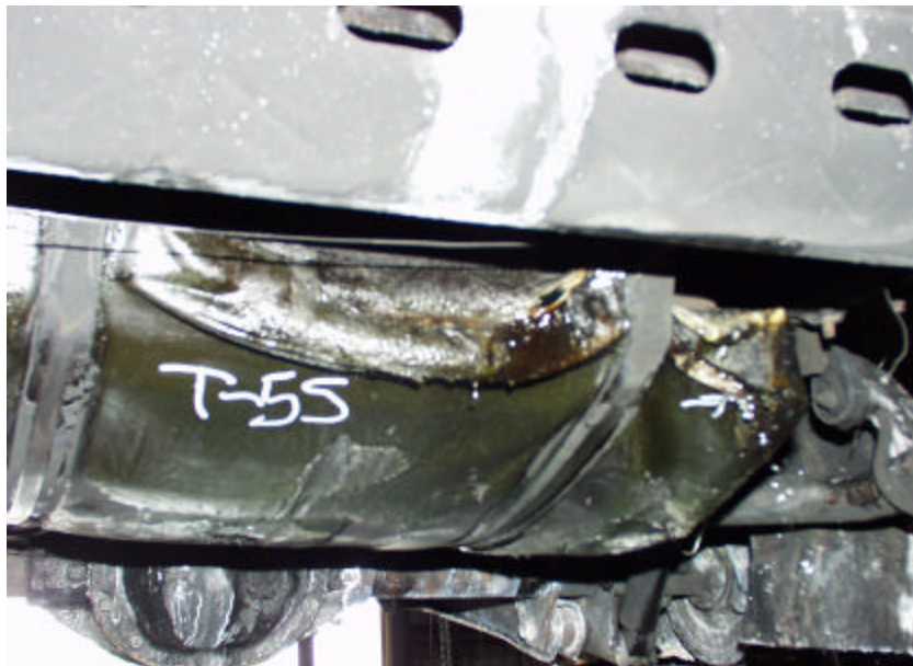
Figure A-124. Test No. 5S, New 1998 Jeep Grand Cherokee Fuel Tank Immediately After Fire Exposure with Heat Shield Removed and Leak Location at Rear of Tank.
