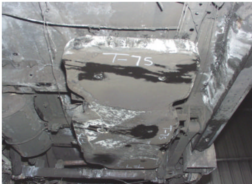
Figure A-164. Test No. 7S, Bottom View of New 1998 Plymouth Grand Voyager Fuel Tank With Heat Shield After Fire Exposure With Leak Location at Front Side and Middle Drain Holes.
