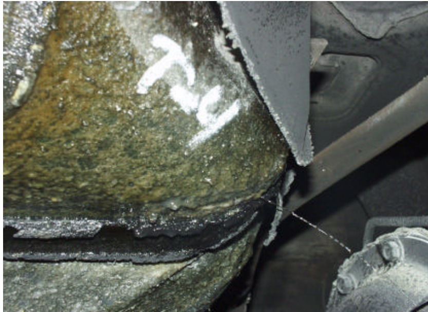
Figure A-107. Test No. 4, New 1998 Jeep Grand Cherokee Fuel Tank Immediately After Fire Exposure with Leak at Front Right Side Bottom of Fuel Tank.
