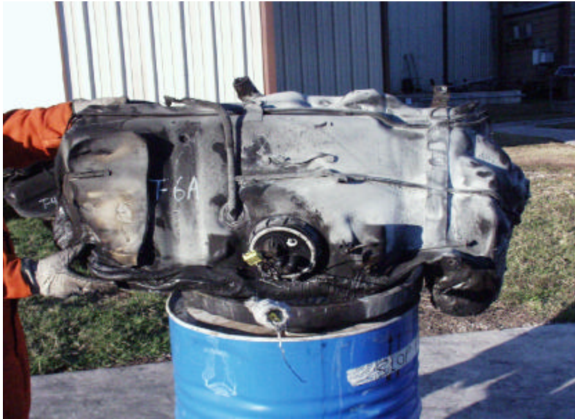
Figure A-149. Test No. 6A, Top View of New 1998 Plymouth Grand Voyager Fuel Tank After Fire Exposure.
