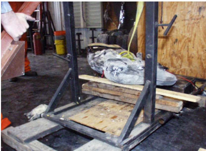
Figure A-221. Front Passenger Side of Conditioned 1998 Plymouth Grand Voyager Fuel Tank Prior to Impact.
