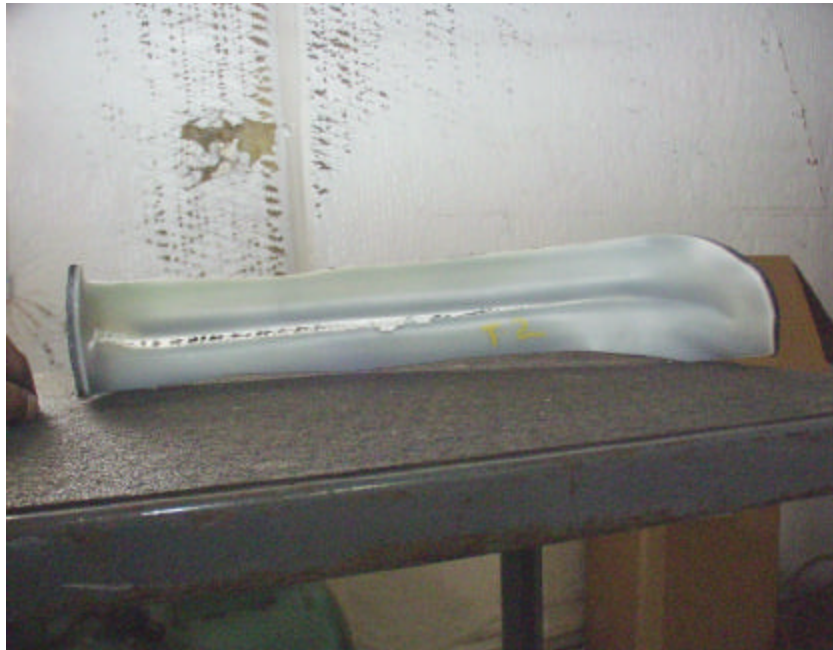
Figure A-35. Internal View of Jeep Tank Pinch-Off Section.
