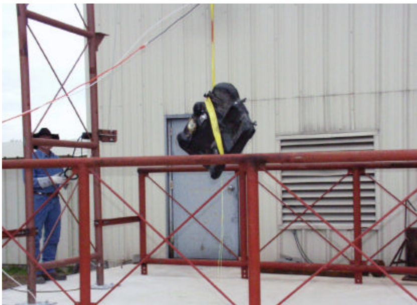
Figure A-225. The Conditioned 2001 Saturn Fuel Tank Filled with 9.05 Gallons of Ethylene Glycol Water Mixture (Equal to 12.2 Gallons of Gasoline) Prior to 30-ft Drop Test on Front Passenger Side Corner.
