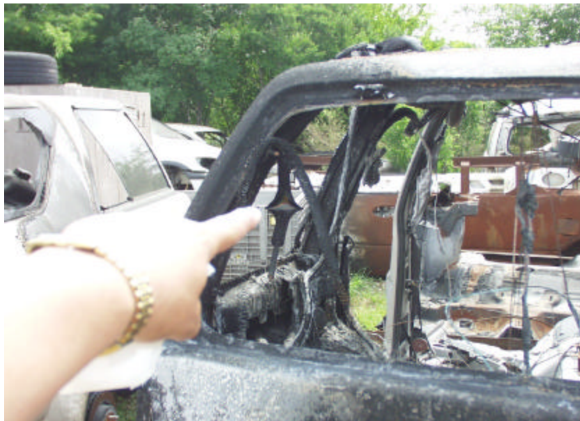
Figure A-130. Test No. 5S, Post-Test Observation of 1998 Jeep Grand Cherokee Lift Gate Strut Support That Vented Loudly During the Test.
