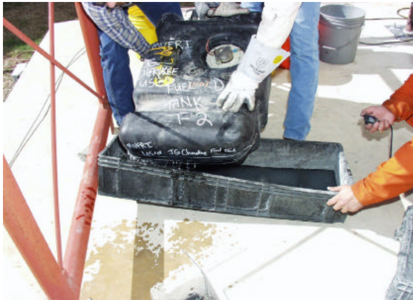
Figure A-243. Leak Rate of 899.49 oz/min of Ethylene-Glycol Water Mixture Due to Pinch-Off Separation at the Front of the Conditioned 1998 Jeep Grand Cherokee Fuel Tank After the 30-ft Drop Test.
