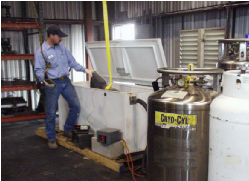
Figure A-202. Impact Resistance -40^{\circ}\text{C} \pm 2^{\circ}\text{C} Conditioning Chamber Connected to 180-lb Bottles of Liquid Nitrogen.
