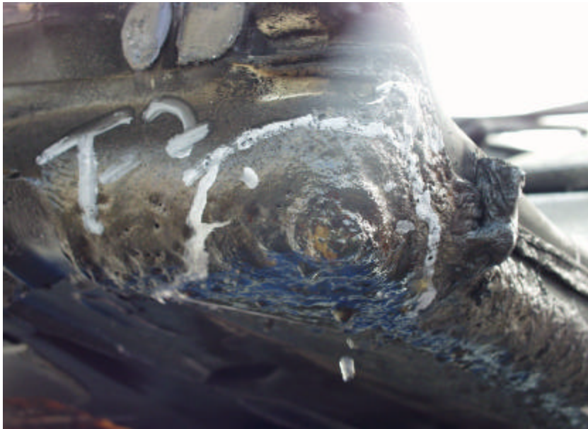
Figure A-60. Test No. 2, Fire Exposure Hole at Front Left Side Bottom Corner of New 1998 Saturn Twin Cam 4-Door Fuel Tank.
