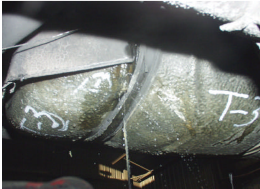
Figure A-95. Test No. 3, Conditioned 1998 Jeep Grand Cherokee Fuel Tank Immediately After Fire Exposure with Leak at Front Right Side Along Outboard Side of Strap.
