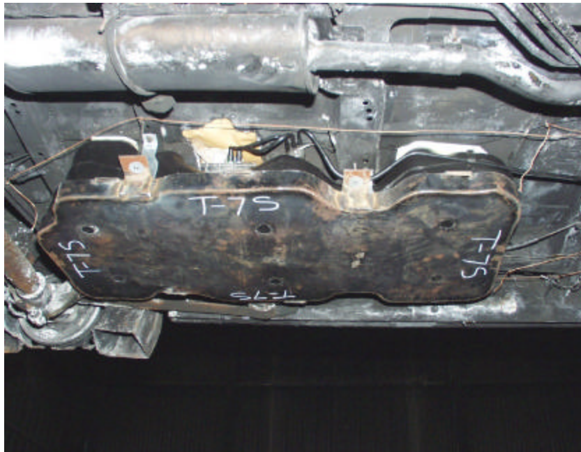
Figure A-22. Test PNP2(S) Before Exposure With Fuel Tank Shield.
