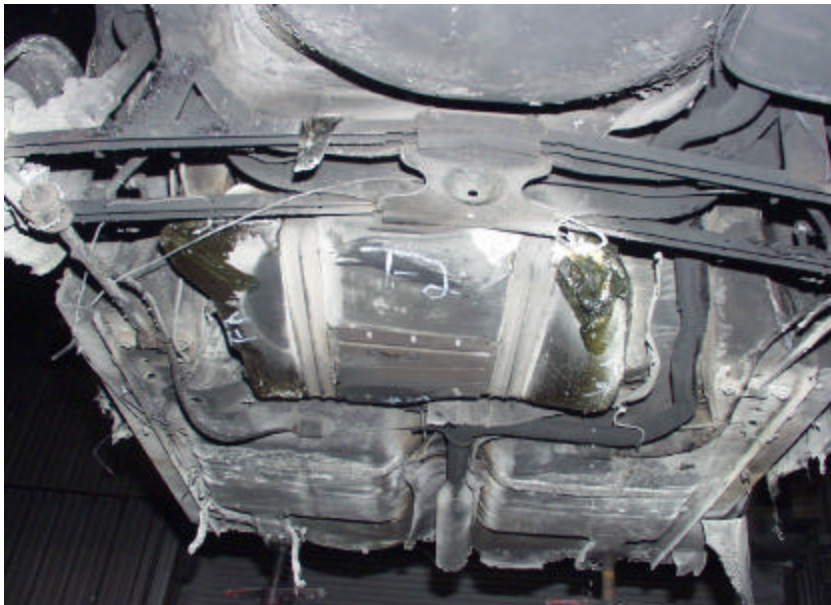
Figure A-72. Test No. 2, Repeatability Evaluation on a New Twin Cam 4-Door Fuel Tank Immediately After Fire Exposure with a Leak on Rear Passenger Side Corner of Fuel Tank.
