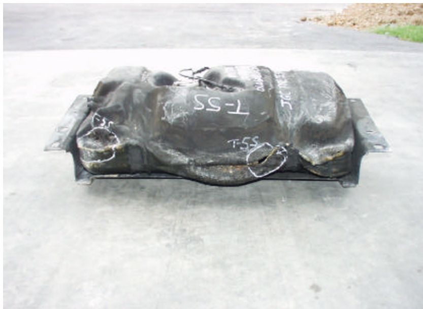
Figure A-128. Test No. 5S, Post-Test Observation of New 1998 Jeep Grand Cherokee Fuel Tank Leak Locations at Rear of Tank.
