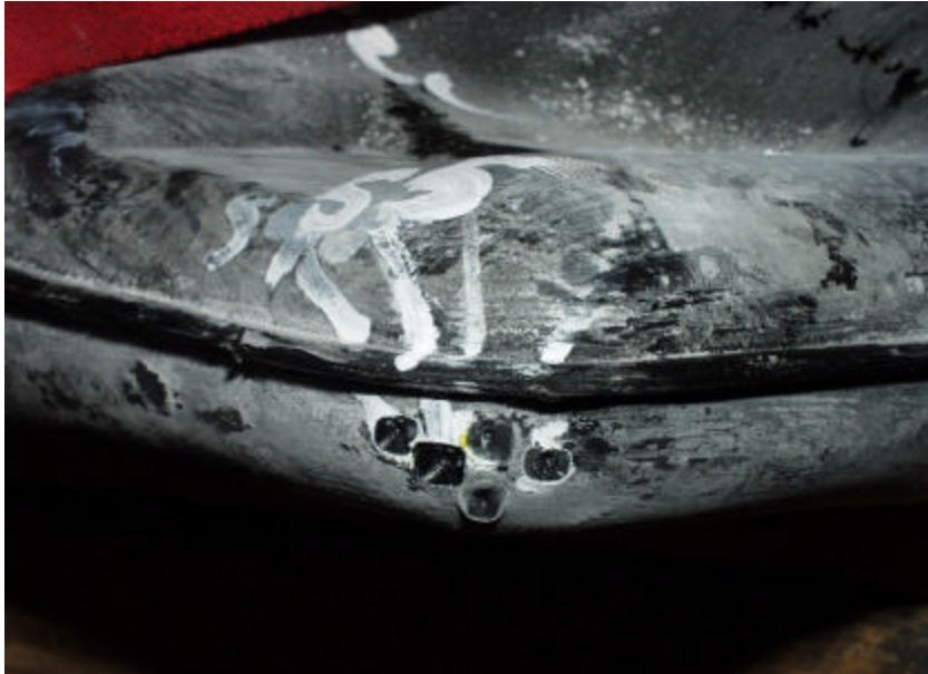
Figure A-208. No Leaks to the Front Passenger Side of the New 1998 Saturn Twin Cam 4-Door Fuel Tank After Five Impacts Ranging Between 30.1 Nm to 43.6 Nm.
