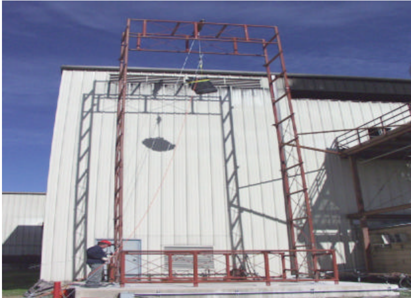
Figure A-241. The Conditioned 1998 Jeep Grand Cherokee Fuel Tank During 30-ft Drop.
