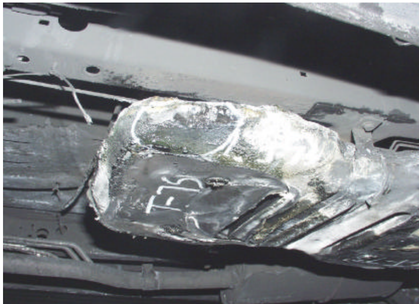
Figure A-172. Test No. 7S, Bottom View of New 1998 Plymouth Grand Voyager Fuel Tank With Heat Shield Removed After Fire Exposure With Leak Location at Front Driver Side Corner of Fuel Tank.
