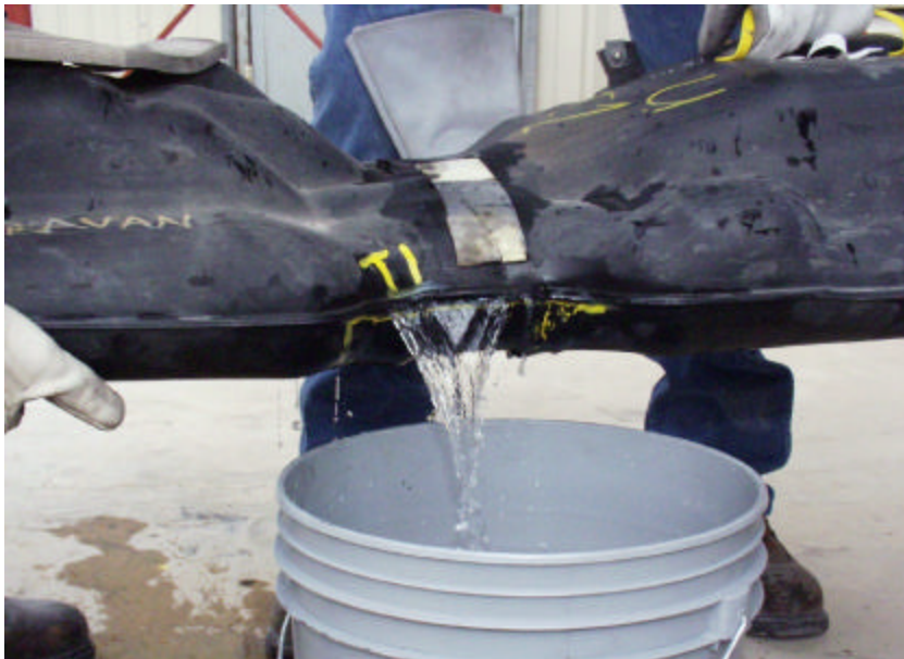
Figure A-233. Leak Rate of 149.98 oz/min of Ethylene -Glycol Water Mixture Due to Pinch-Off Separation at Front Strap Location of the 2000 Plymouth Grand Voyager Fuel Tank After the 30-ft Drop Test.
