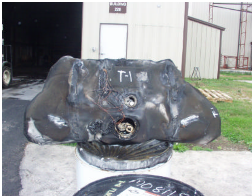
Figure A-26. Conditioned Metal Fuel Tank After Exposure.
