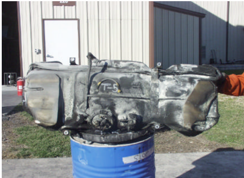
Figure A-140. Test No. 5, Top View of Conditioned 1998 Plymouth Grand Voyager Fuel Tank After Fire Exposure.
