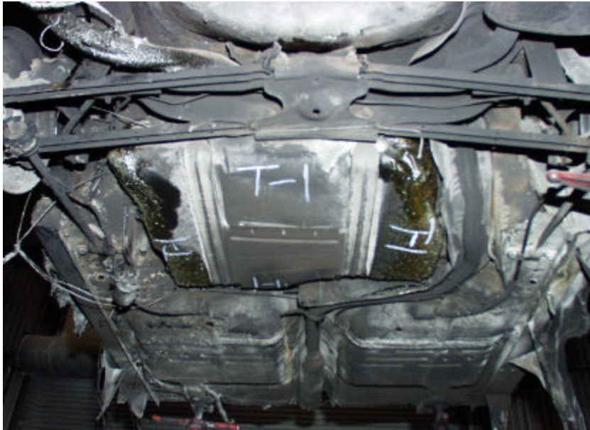
Figure A-48. Test No. 1, Conditioned 1998 Saturn Twin Cam 4-Door Fuel Tank Immediately After Fire Exposure.
