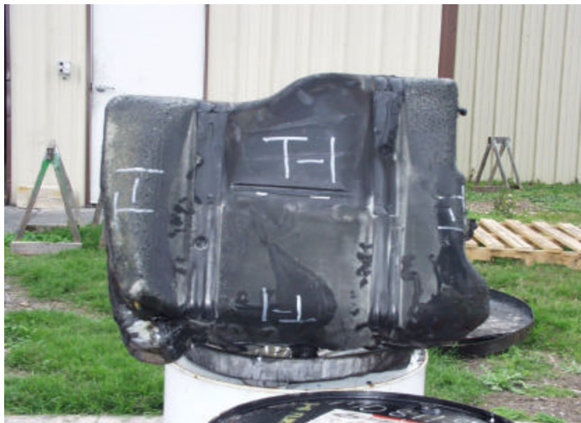
Figure A-68. Test No. 1, Repeatability Evaluation on a New 1998 Saturn Twin Cam 4-Door Fuel Tank with No Leaks, Bottom View; Classified as a Non-Failed Test.
