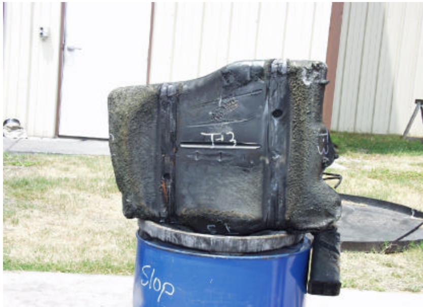
Figure A-85. Test No. 3, Repeatability Evaluation on a New 1998 Saturn Twin Cam 4-Door Fuel Tank After Fire Exposure, Bottom View.
