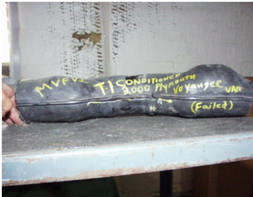
Figure A-32. External View of Plymouth Tank Pinch-Off Section.
