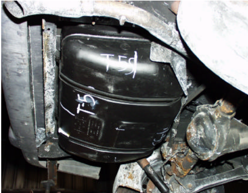
Figure A-15. Test JNP2(S) Before Exposure Without Skid-Plate.
