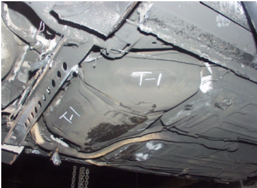
Figure A-199. Test No. 1 (February 18, 2003), Conditioned 1999 Chevrolet Cavalier Metal Fuel Tank Immediately After Fire Exposure.
