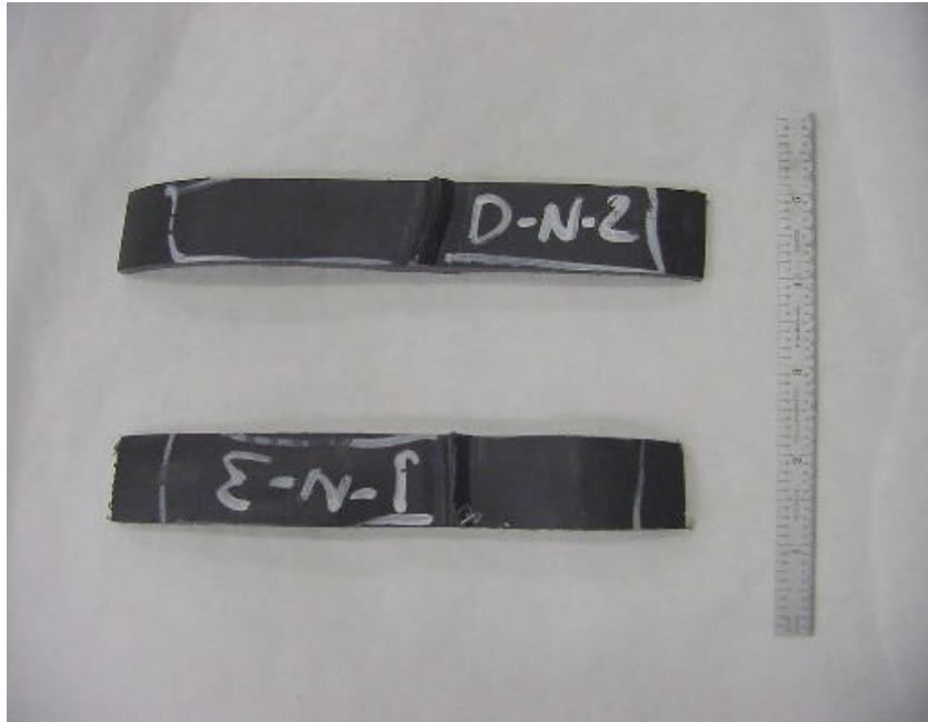
Figure A-37. Typical Tensile Test Specimen Coupon.
