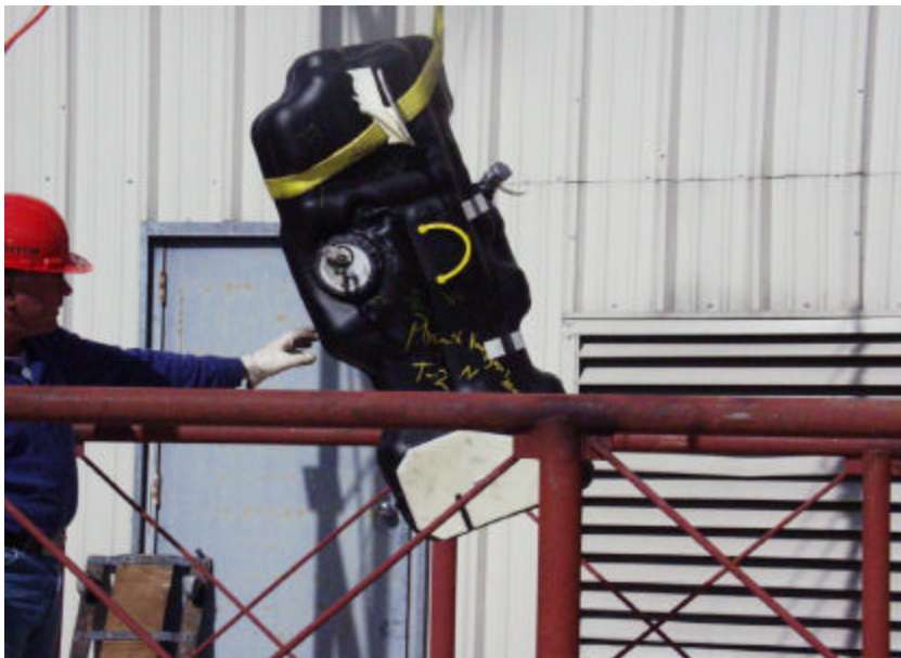
Figure A-234. The New 1998 Plymouth Grand Voyager Fuel Tank Filled with 14.83 Gallons of Ethylene Glycol Water Mixture (Equal to 20 Gallons of Gasoline) Prior to 30-ft Drop Test on the Front Passenger Side Corner.
