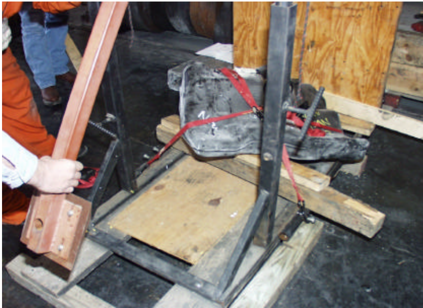
Figure A-204. Front Passenger Side of the Conditioned 1998 Saturn Twin Cam 4-Door Fuel Tank Prior to Impact.
