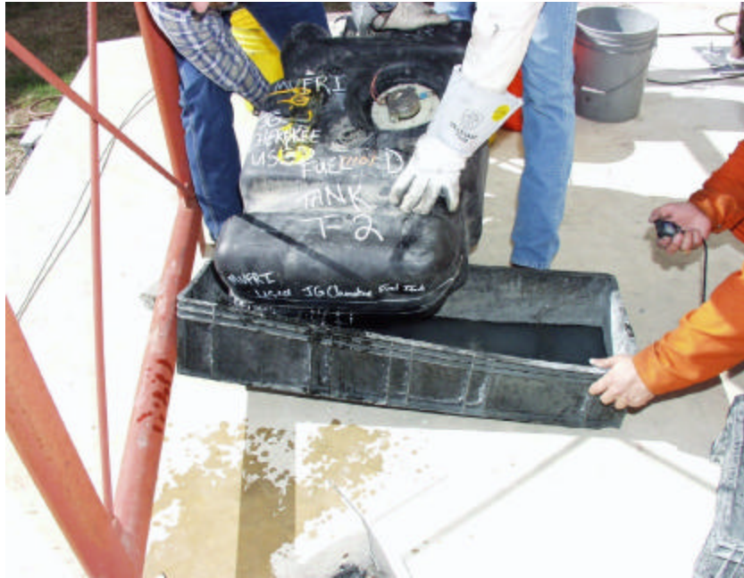
Figure A-31. Leakage of Conditioned Plymouth Plastic Fuel Tank After Impact.
