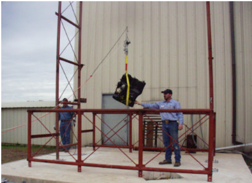
Figure A-228. The New 1998 Saturn Fuel Tank Filled with 9.05 Gallons of Ethylene Glycol Water Mixture (Equal to 12.2 Gallons of Gasoline) Prior to 30-ft Drop Test on Front Passenger Side Corner.
