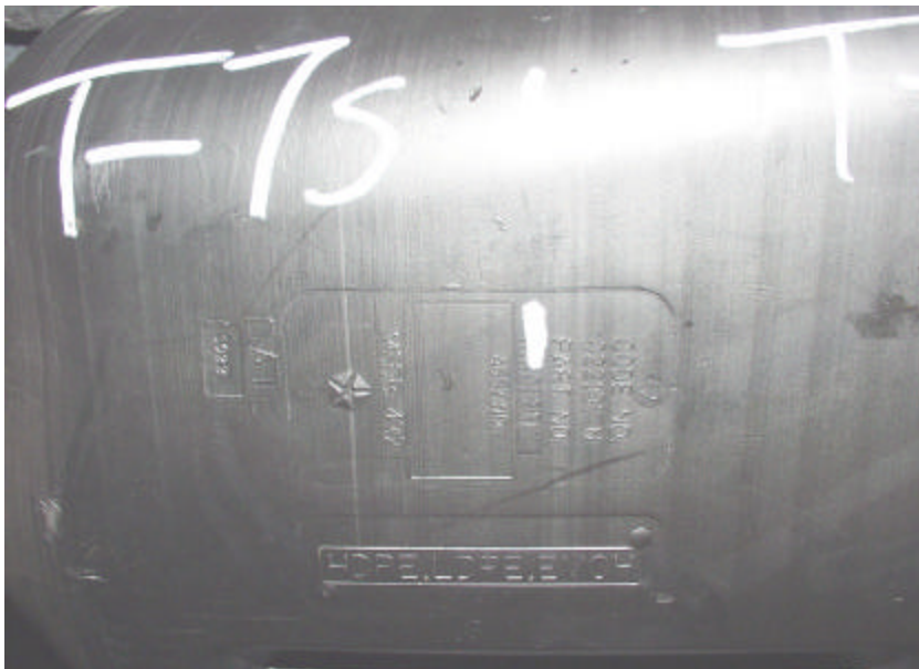
Figure A-156. DaimlerChrysler Manufacturer Imprint on Bottom Side of New 1998 Plymouth Grand Voyager Fuel Tank.
