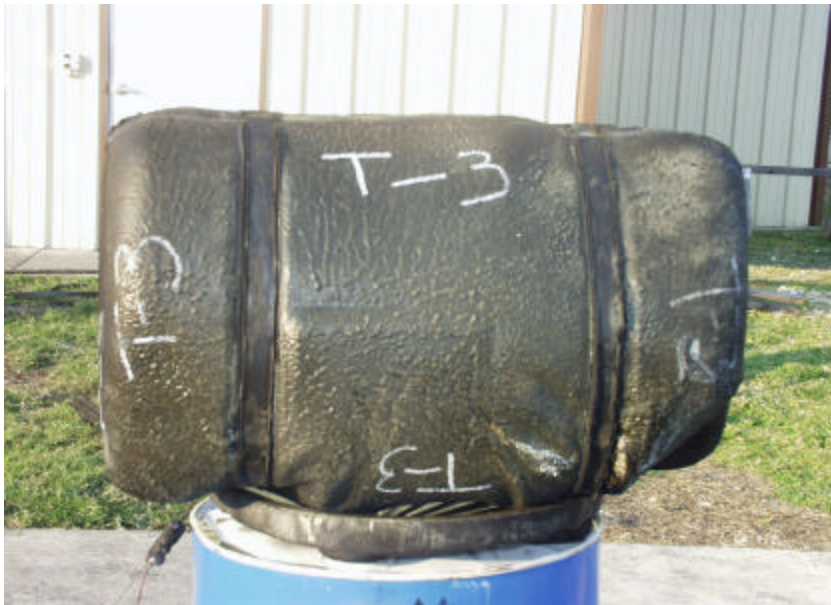
Figure A-98. Test No. 3, Bottom View of Conditioned 1998 Jeep Grand Cherokee Fuel Tank After Fire Exposure.
