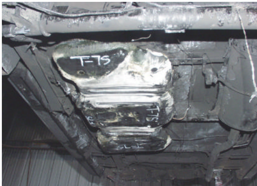
Figure A-170. Test No. 7S, Bottom View of New 1998 Plymouth Grand Voyager Fuel Tank With Heat Shield Removed After Fire Exposure.
