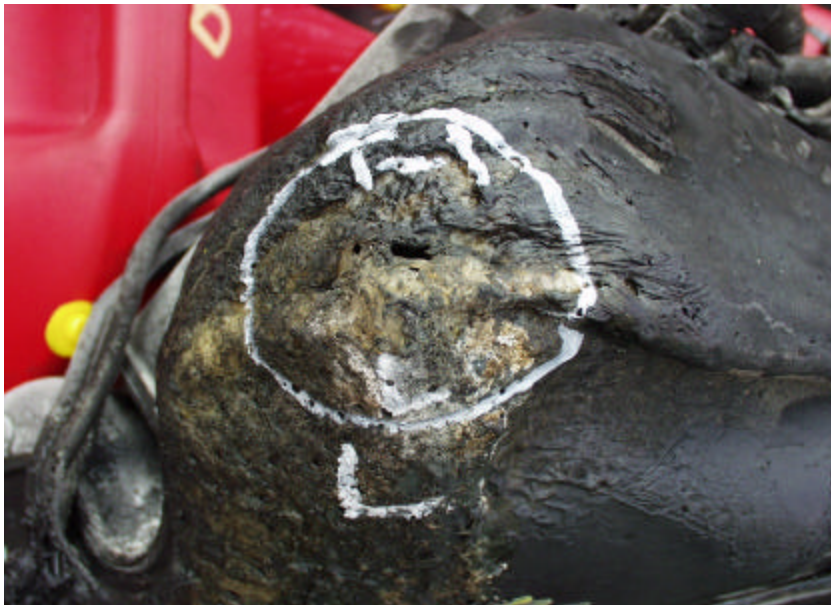
Figure A-51. Test No. 1, Fire Exposure Hole at Rear Left Side Bottom Corner of Conditioned 1998 Saturn Twin Cam 4-Door Fuel Tank.
