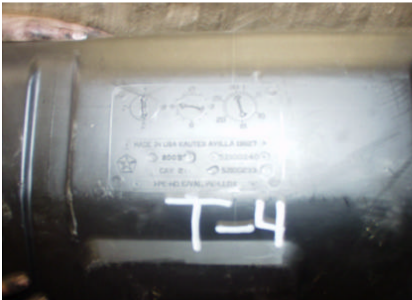
Figure A-102. KAUTEX Manufacturer Imprint on Bottom Side of New 1998 Jeep Grand Cherokee Fuel Tank.
