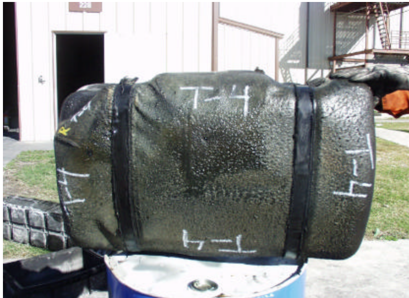
Figure A-109. Test No. 4, Bottom View of New 1998 Jeep Grand Cherokee Fuel Tank After Fire Exposure.
