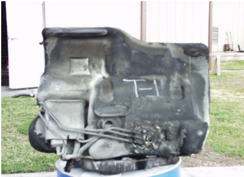
Figure A-49. Test No. 1, Top View of Conditioned 1998 Saturn Twin Cam 4-Door Fuel Tank After Fire Exposure.
