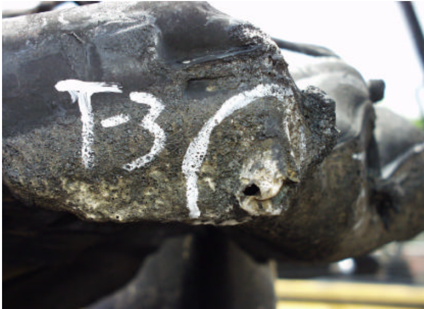
Figure A-87. Test No. 3, New 1998 Saturn Twin Cam 4-Door Fuel Tank Post-Test Observation at Front Left Passenger Side Bottom Corner of Fuel Tank.
