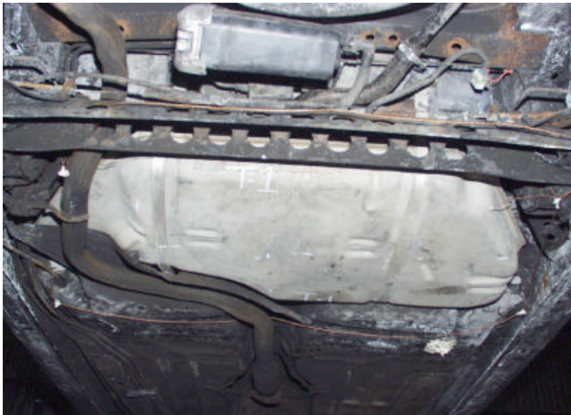
Figure A-197. Test No. 1 (February 18, 2003), Conditioned 1999 Chevrolet Cavalier Metal Fuel Tank Assembly Mounted in Test Platform Prior to Testing.
