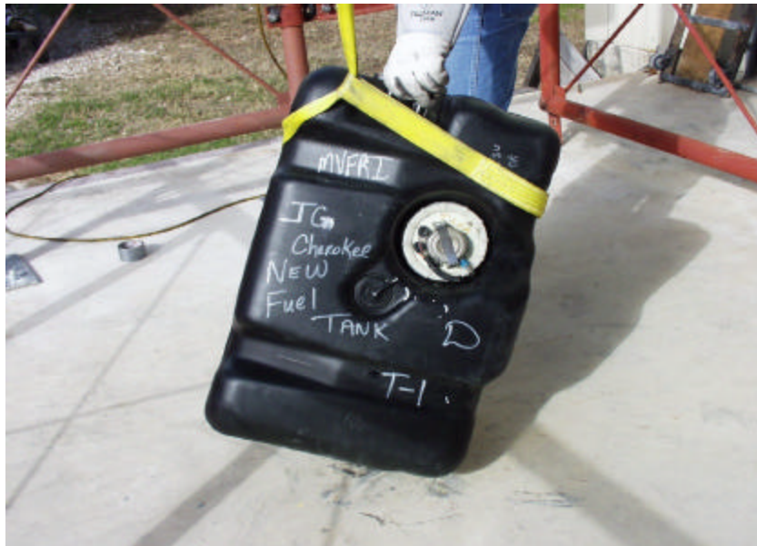
Figure A-237. The New 1998 Jeep Grand Cherokee Fuel Tank Filled with 17.05 Gallons of Ethylene Glycol Water Mixture (Equal to 23 Gallons of Gasoline) Prior to 30-ft Drop Test on the Front Passenger Side Corner.
