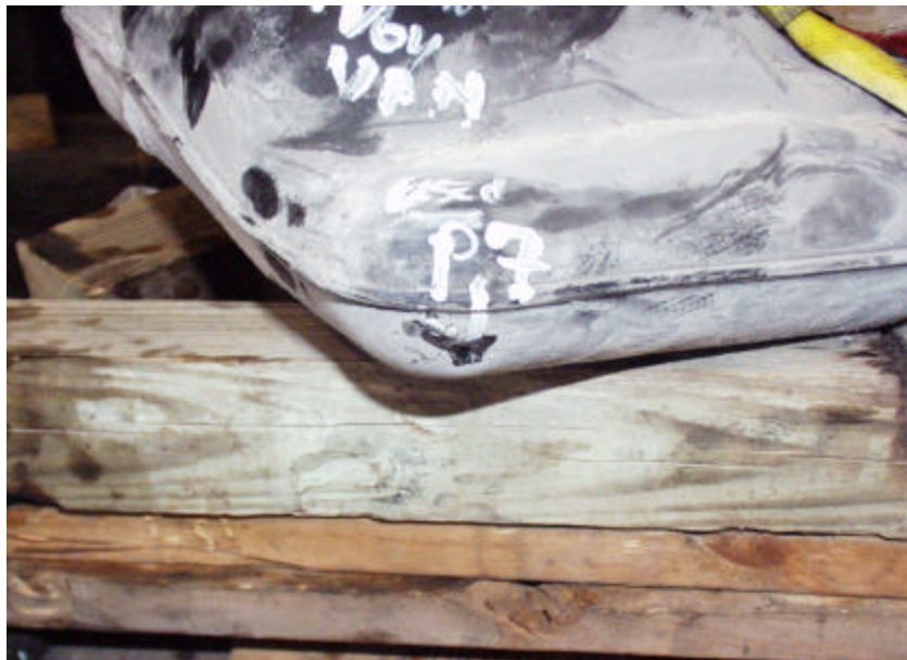
Figure A-224. No Leaks to the Front Driver Side of the Conditioned 1998 Plymouth Grand Voyager Fuel Tank After Two Impacts Ranging Between 43.6 Nm and 147.2 Nm.
