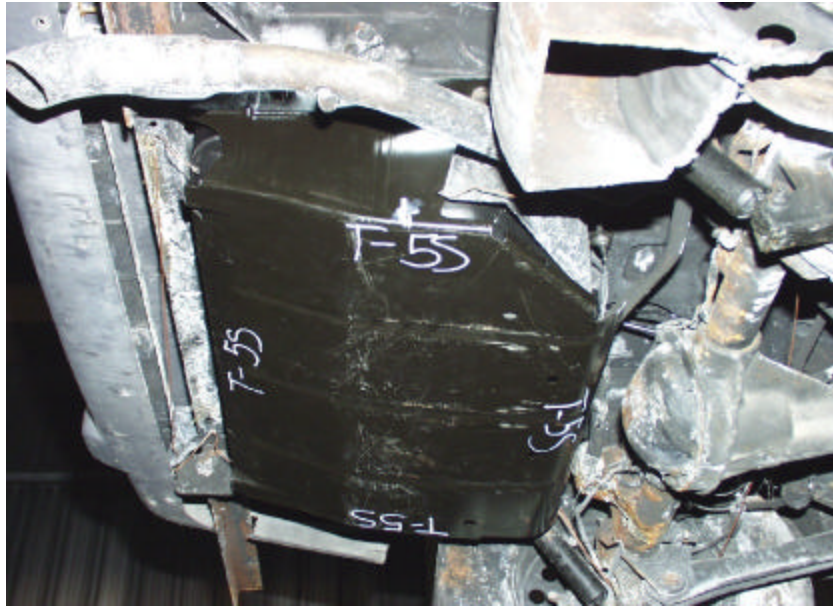
Figure A-117. Test No. 5S, New 1998 Jeep Grand Cherokee Fuel Tank Mounted in Test Platform with Heat Shield, Prior to Testing.
