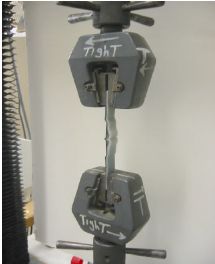
Figure A-39. Typical Tensile Test Setup.
