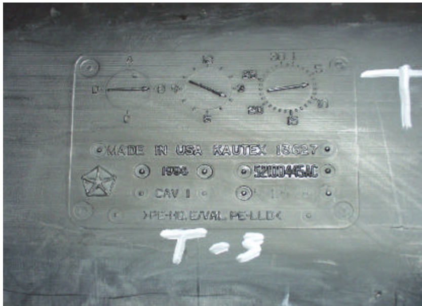
Figure A-90. KAUTEX Manufacturer Imprint on Bottom Side of Conditioned 1998 Jeep Grand Cherokee Fuel Tank.
