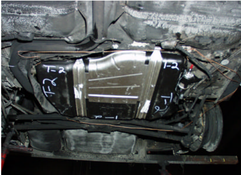
Figure A-54. Test No. 2, New 1998 Saturn Twin Cam 4-Door Fuel Tank Mounted in Test Platform Prior to Testing.
