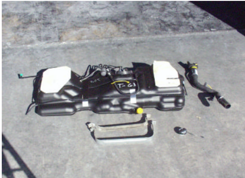
Figure A-142. New 1998 Plymouth Grand Voyager Fuel Tank Assembly.
