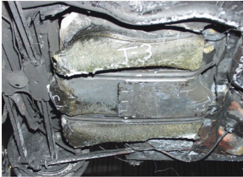
Figure A-83. Test No. 3, Repeatability Evaluation on a New 1998 Saturn Twin Cam 4-Door Fuel Tank Immediately After Fire Exposure with a Leak at Front Left Passenger Side Bottom Corner and Rear Left Passenger Side of Fuel Tank.
