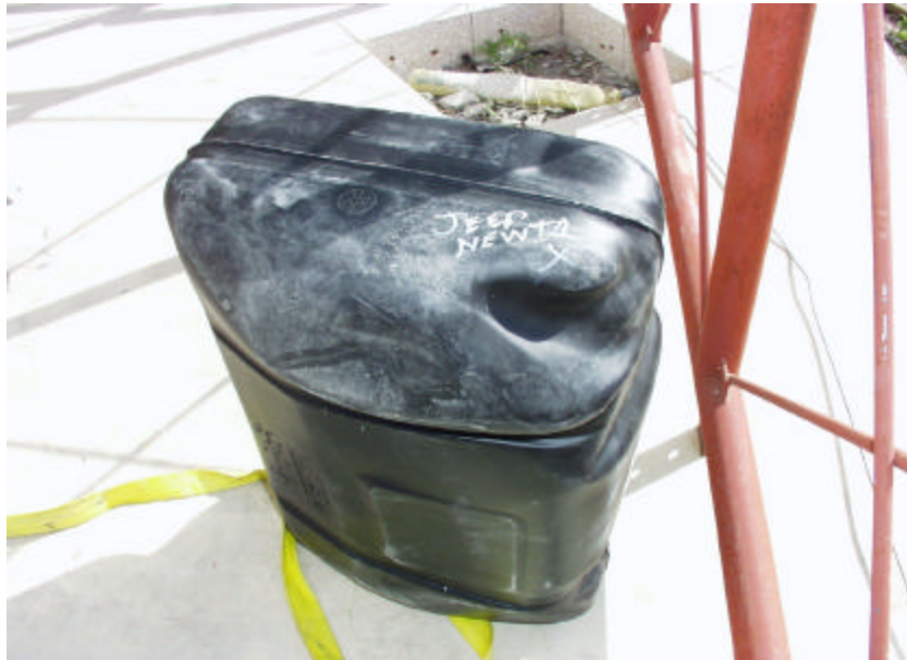
Figure A-239. No Leaks on Front Passenger Side Corner of the New 1998 Jeep Grand Cherokee Fuel Tank After the 30-ft Drop Test.
