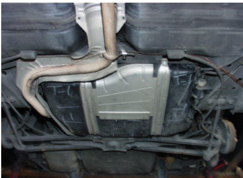
Figure A-45. Test No. 1, Conditioned 1998 Saturn Twin Cam 4-Door Fuel Tank Mounted in Test Platform Prior to Testing.
