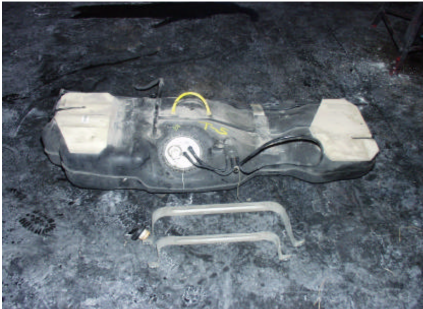
Figure A-132. Conditioned 1998 Plymouth Grand Voyager Fuel Tank Assembly.
