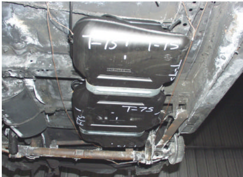
Figure A-158. Test No. 7S, Bottom Side of New 1998 Plymouth Grand Voyager Fuel Tank Assembly Without Bottom Heat Shield, Prior to Test.
