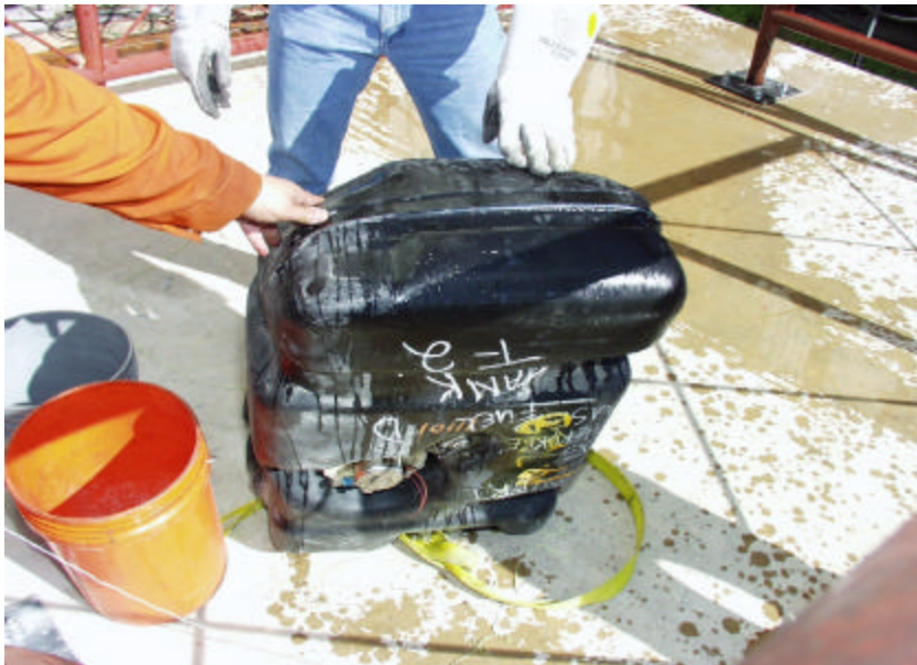
Figure A-242. Leak Due to Pinch-Off Separation of the Conditioned 1998 Jeep Grand Cherokee Fuel Tank After the 30-ft Drop Test.
