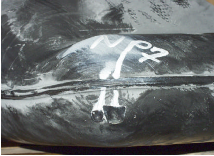
Figure A-220. No Leaks to the Front Driver Side of the New 1998 Plymouth Grand Voyager Fuel Tank After Two Impacts Ranging Between 43.6 Nm and 147.2 Nm.
