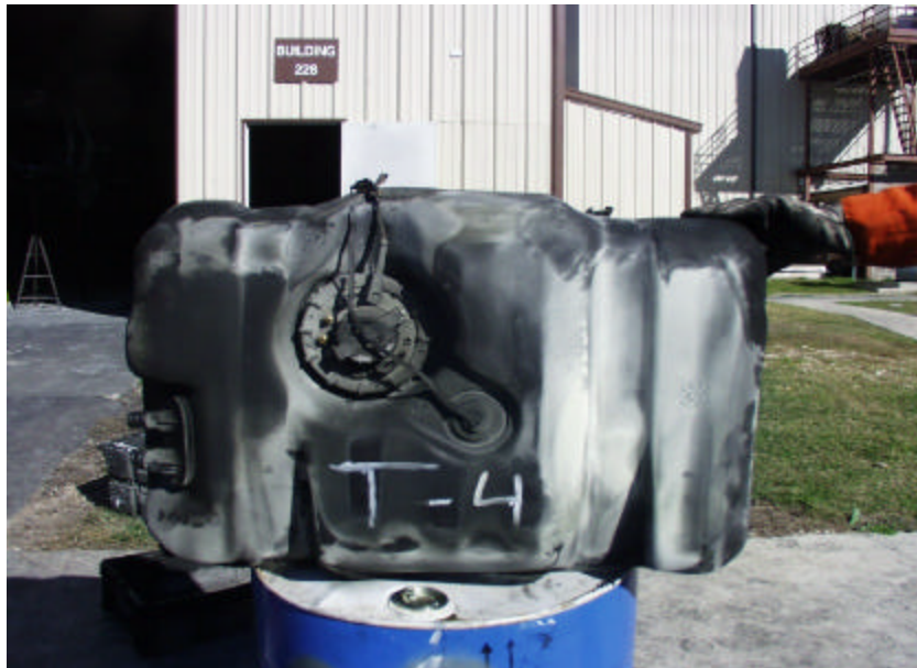
Figure A-108. Test No. 4, Top View of New 1998 Jeep Grand Cherokee Fuel Tank After Fire Exposure.
