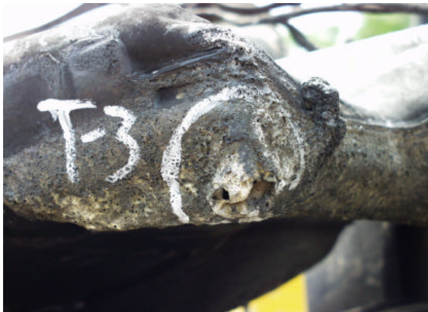
Figure A-86. Test No. 3, New 1998 Saturn Twin Cam 4-Door Fuel Tank Post-Test Observation at Front Left Passenger Side Bottom Corner of Fuel Tank.
