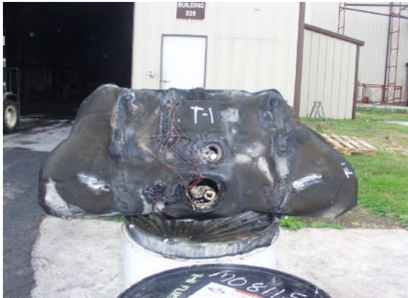
Figure A-200. Test No 1, (February 18, 2003), Top View of Conditioned 1999 Chevrolet Cavalier Metal Fuel Tank After Fire Exposure.
