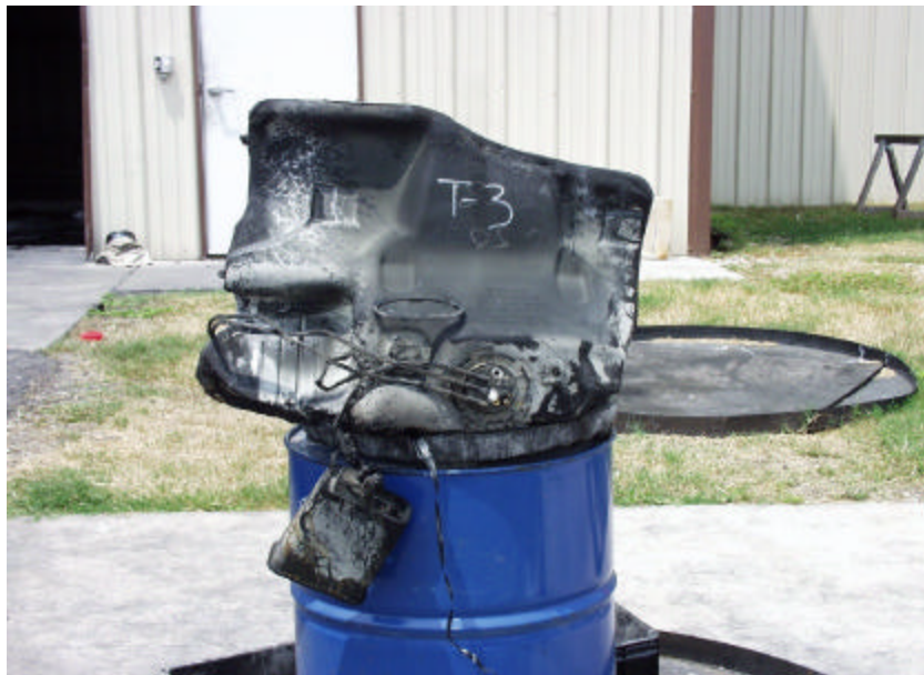
Figure A-84. Test No. 3, Repeatability Evaluation on a New 1998 Saturn Twin Cam 4-Door Fuel Tank After Fire Exposure, Top View.
