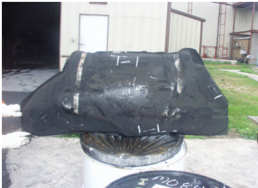
Figure A-201. Test No. 1 ((February 18, 2003), Bottom View of Conditioned 1999 Chevrolet Cavalier Metal Fuel Tank After Fire Exposure.
