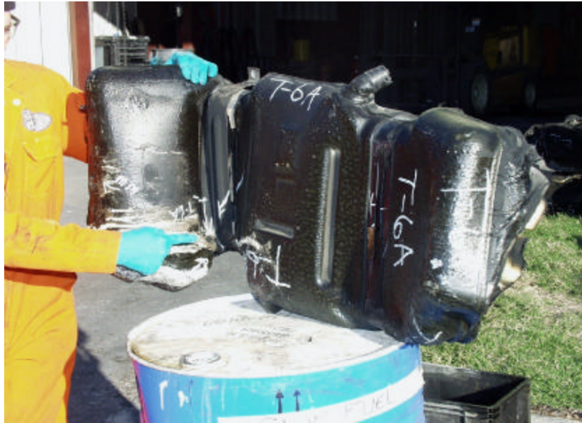
Figure A-151. Test No. 6A, Bottom View of New 1998 Plymouth Grand Voyager Fuel Tank After Fire Exposure at Front Strap Leak Location.
