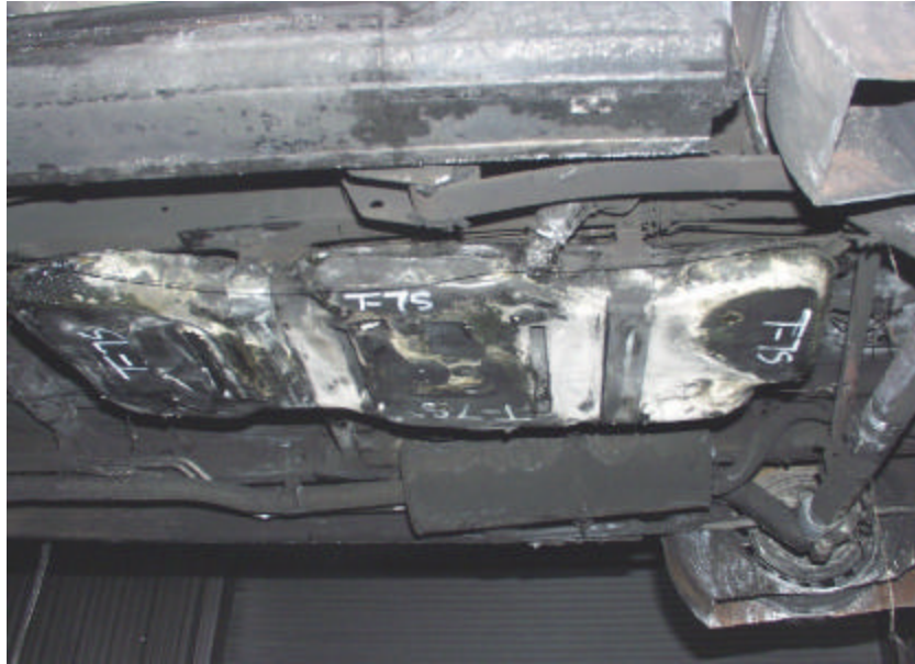
Figure A-171. Test No. 7S, Bottom View of New 1998 Plymouth Grand Voyager Fuel Tank With Heat Shield Removed After Fire Exposure.
