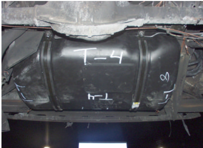
Figure A-103. Test No. 4, New 1998 Jeep Grand Cherokee Fuel Tank Mounted in Test Platform Prior to Testing.
