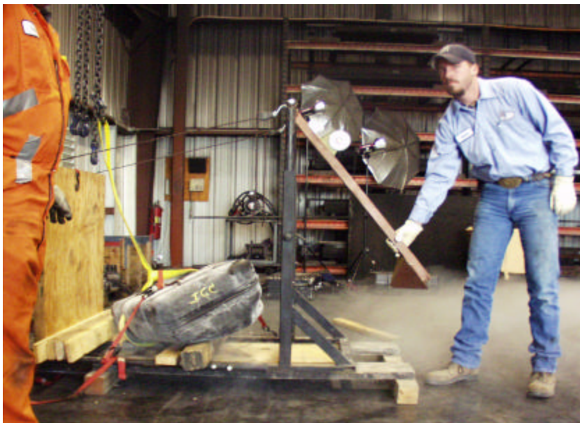
Figure A-211. Front Passenger Side of the Conditioned 1998 Jeep Grand Cherokee Fuel Tank Prior to Impact.
