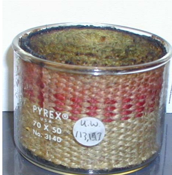
Figure B-1-5. Fluid soaked burlap cloth cylindrical wick inside a Pyrex dish.
