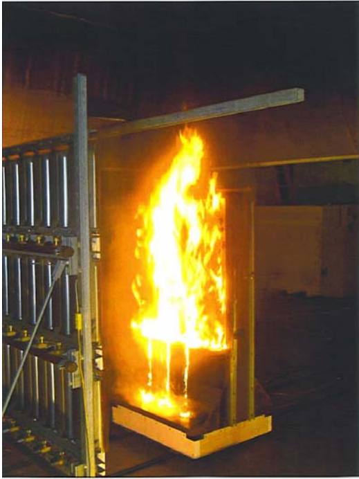
Figure 2-1 Burning of battery cover System in the ASTM E1623 ICAL. Figure is taken from Ref. 1.
