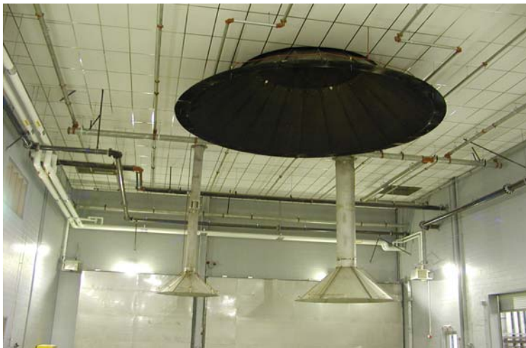
Figure 2-4 The Fire Products Collectors at FM Global. Collector in the back right side was used in the tests. Details are described in Ref. 5.
