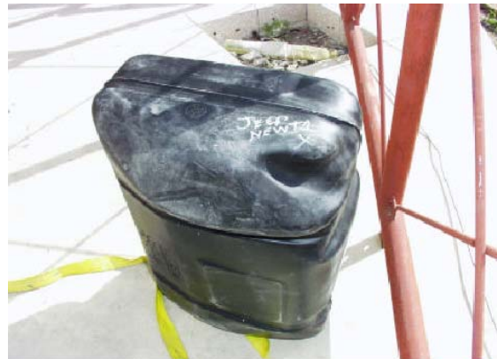
Figure 4 – Jeep Grand Cherokee tank before and after impact
