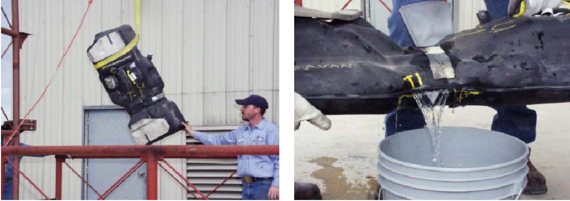
Figure 5 – Plymouth Grand Voyager tank before and after impact
