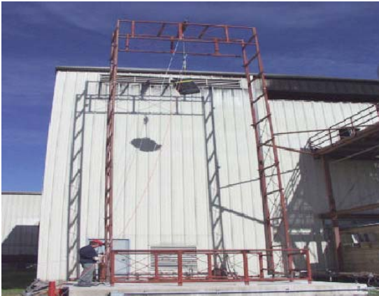
Figure 3 – SwRI Drop Test Setup
