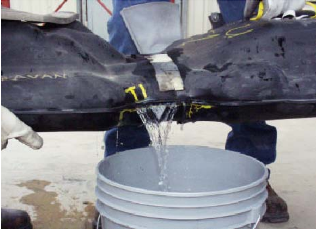
Figure 27 – Failure in the neck area observed in the SwRI Voyager drop test
