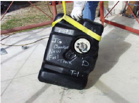
Figure 4 – Jeep Grand Cherokee tank before and after impact
