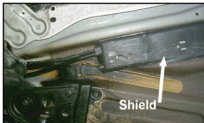
Figure 4 – Partial fuel line shielding
