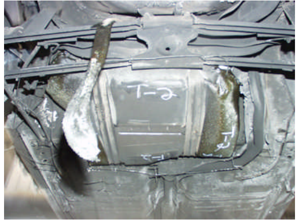
Figure 4. "Pancake" shaped tank post-test.
