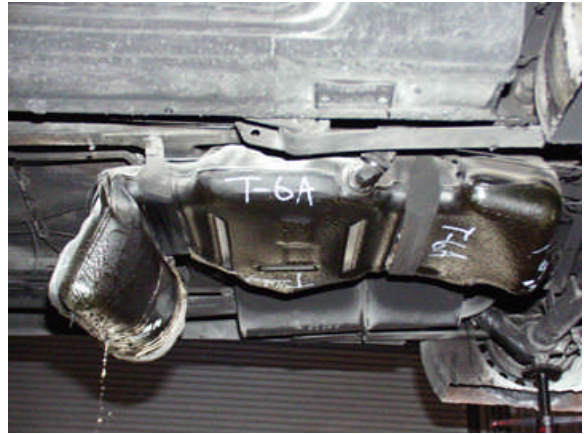
Figure 5. "Long" shaped tank post-test.
