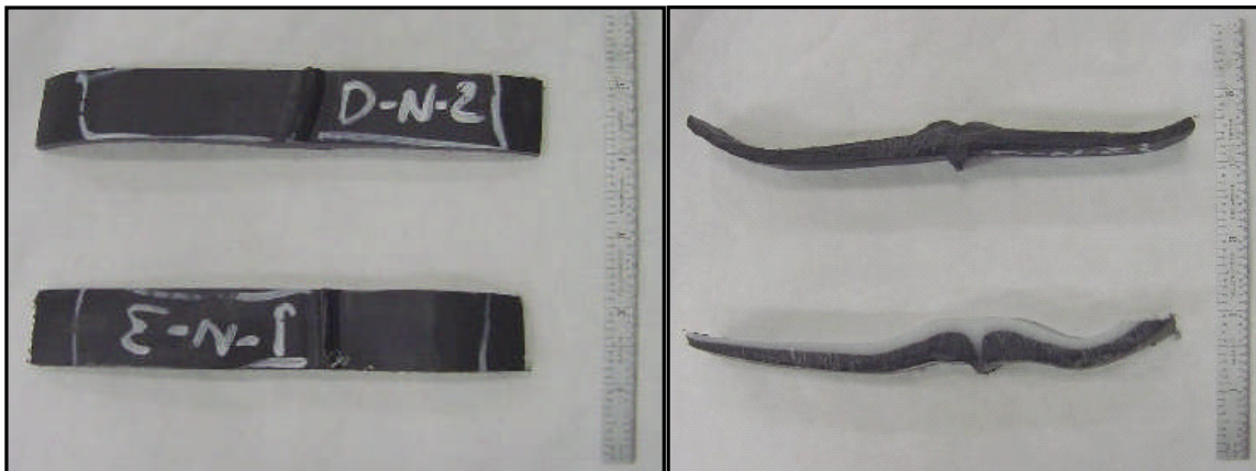
Figure 8 – Material coupons extracted for the tensile testing
