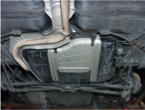
Figure 1. "Pancake" shaped tank pre-test.
