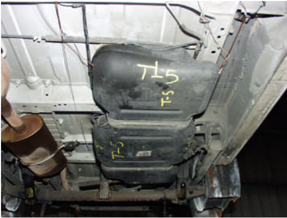
Figure 2. "Long" shaped tank pre-test.
