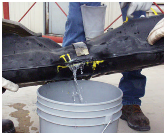
Figure 7. Seasoned “long” tank post drop test
