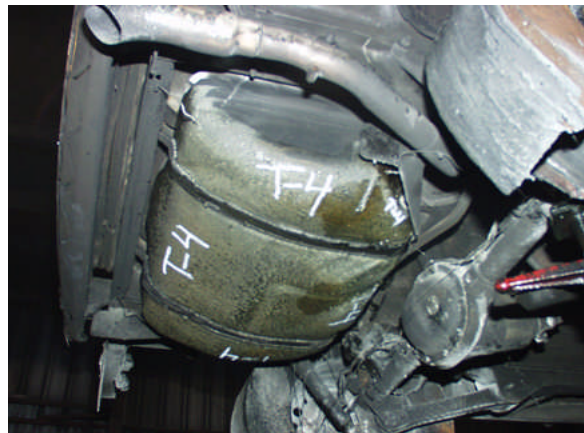
Figure 6. "Square" shaped tank post-test.
