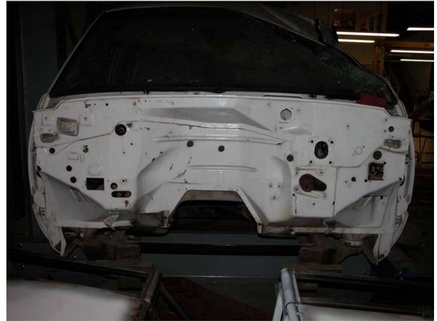
Small Firewall Openings
