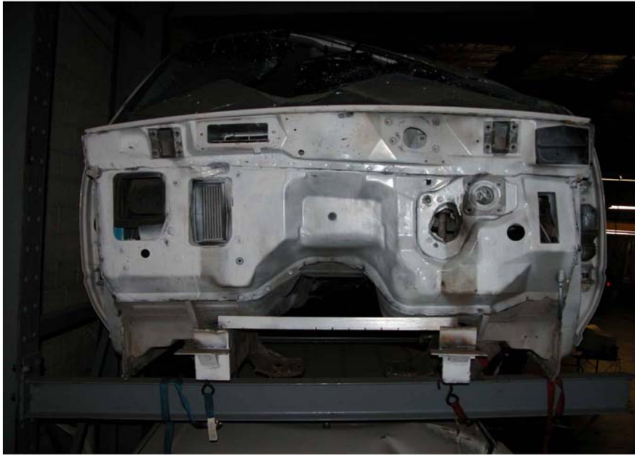
Large Firewall Openings
