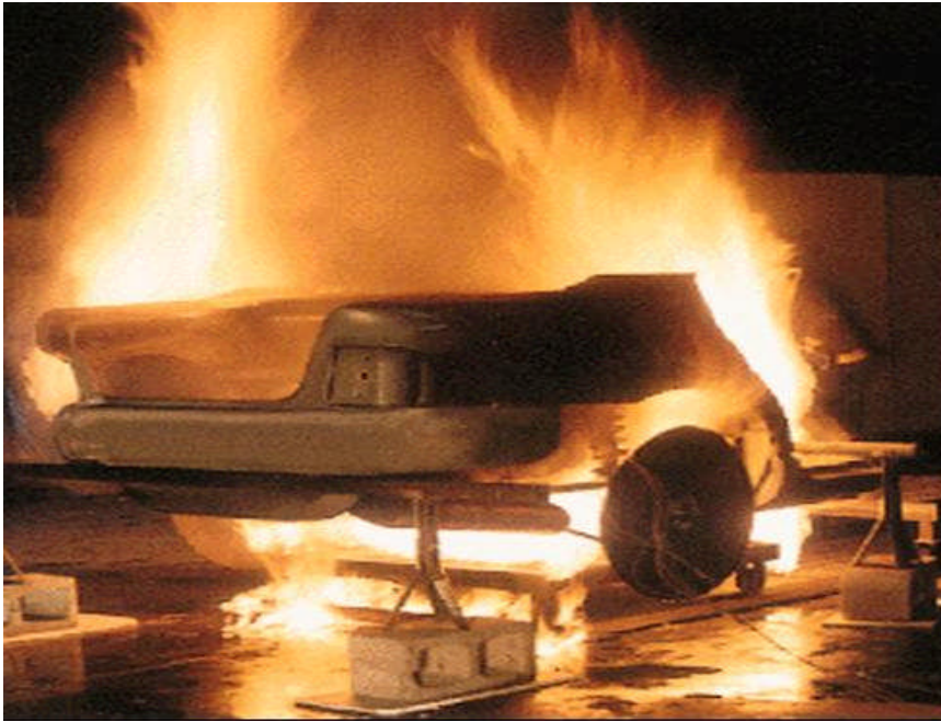
Figure 3. ECE R-34 Bonfire Test
