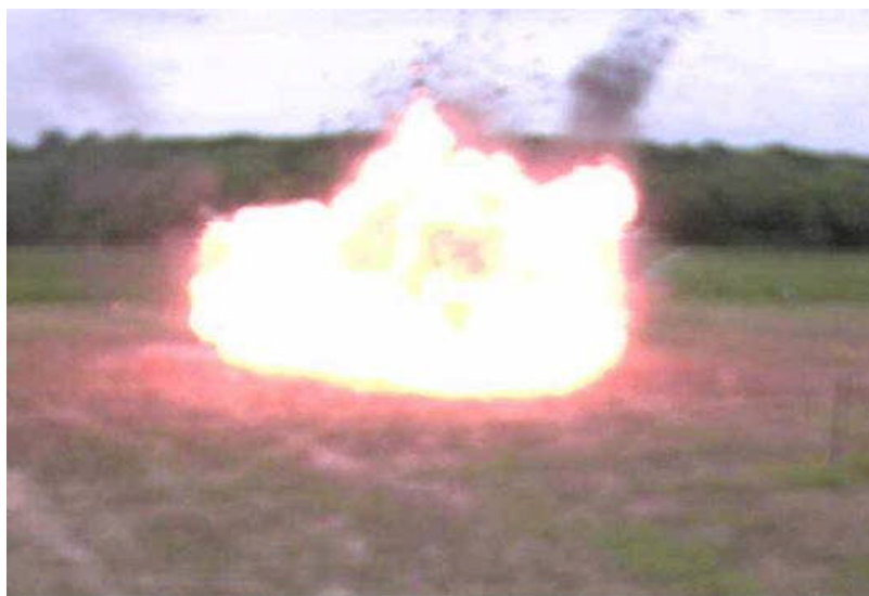
Figure 2. Hydrogen Tank Burst in FMVSS 304-Like Test
