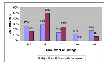
Figure 31. Distribution of Extent of Damage for All Major Fires and Major Fires with Entrapment that Occur in Side Crashes– Vehicles Less than 10 Years Old
