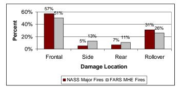
Figure 5. Distribution of Crashes with Fires by Damage Location for Major Fires in NASS/CDS and MHE Fires in FARS 1997- 2005
