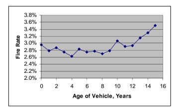
Figure 4. Fire Rate (Fires per Crash Involved Vehicle in FARS) vs. Age of Vehicle – FARS 2000 to 2002
