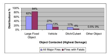
Figure 10. Distribution of 1<sup>st</sup> Object Contacted for All Major Fires and Major Fires with Fatalities that Occur in Frontal Crashes– Vehicles Less than10 Years Old
