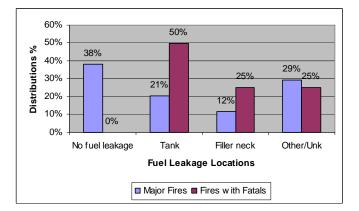
Figure 26. Distribution of Fuel Leakage Location for All Major Fires and Major Fires with Fatalities that Occur in Side Crashes– Vehicles Less than 10 Years Old
