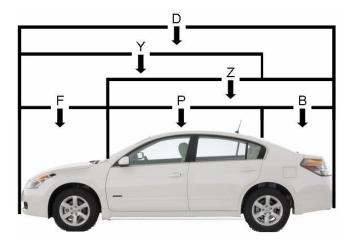
Figure 23. CDC Damage Horizontal Location
