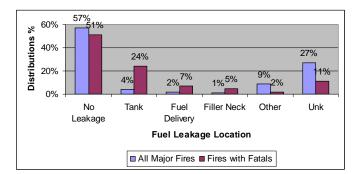
Figure 8. Distribution of Fuel Leakage Location for All Major Fires and Major Fires with Fatalities that Occur in Frontal Crashes– Vehicles Less than 10 Years Old
