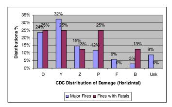
Figure 28. Distribution of Damage Horizontal Location for All Major Fires and Major Fires with Fatalities that Occur in Side Crashes– Vehicles Less than 10 Years Old
