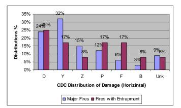
Figure 30. Distribution of Damage Horizontal Location for All Major Fires and Major Fires with Entrapment that Occur in Side Crashes– Vehicles Less than 10 Years Old
