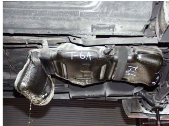
Figure 15. "Long" tank after fire test.
