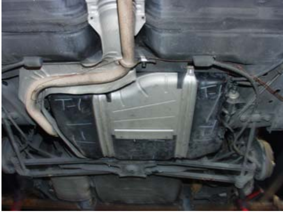
Figure 11. "Pancake" shaped tank pre-test.
