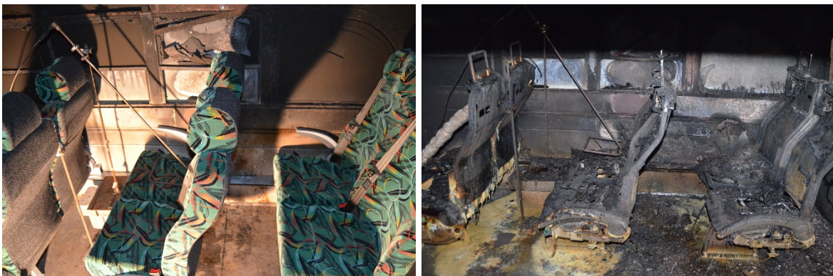
Figure 23. Pre (left) and post (right) test photographs from Test 1 of second series of testing
