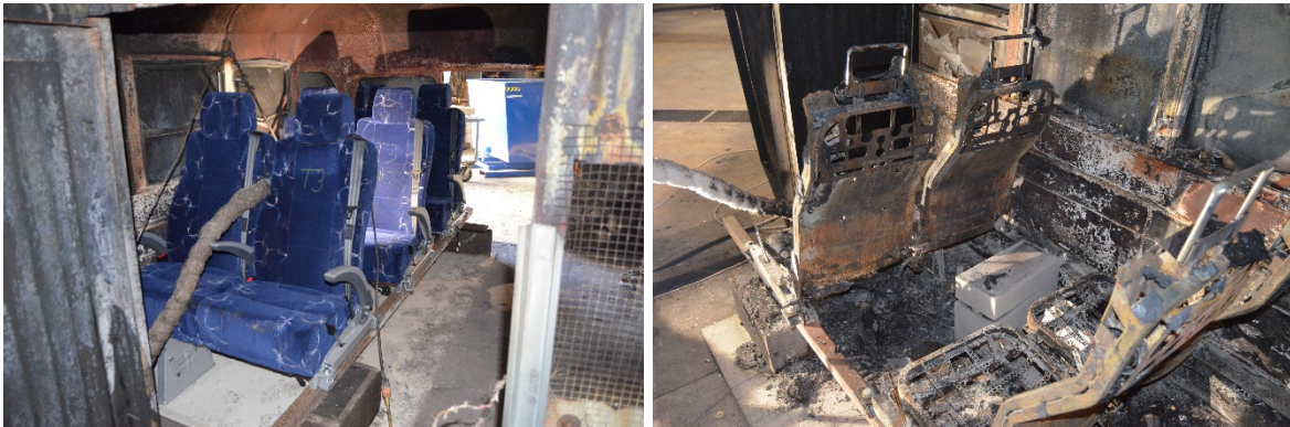
Figure 25. Pre (left) and post (right) test photographs from Test 3 of second series of testing
