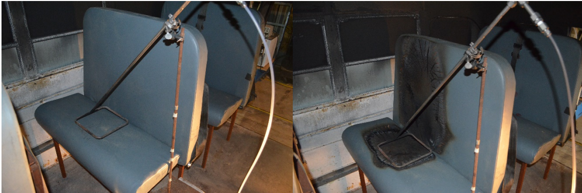
Figure 20. Pre (left) and post (right) test photographs of Bluebird school bus seat
