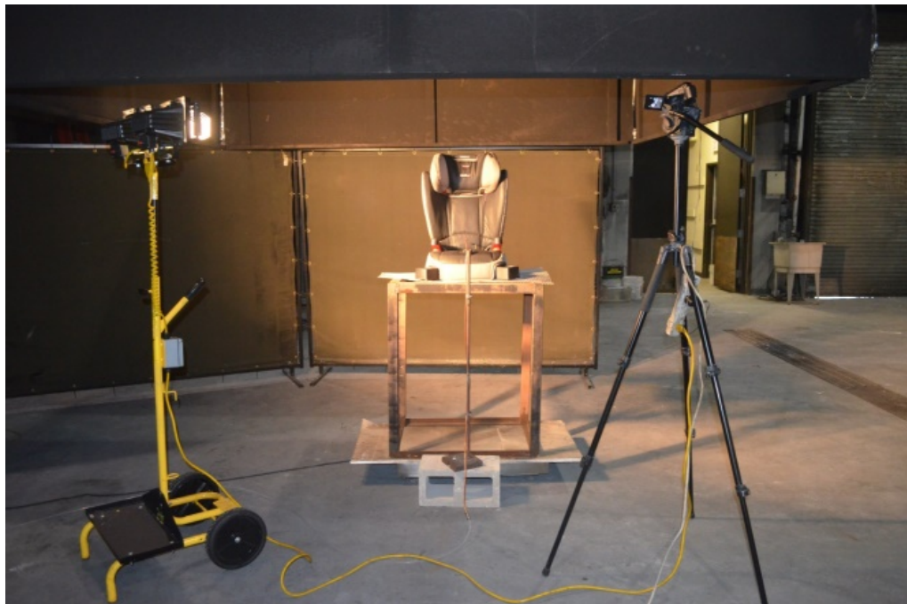
Figure 30. Photograph of CRS test setup (Britax CRS pictured)
