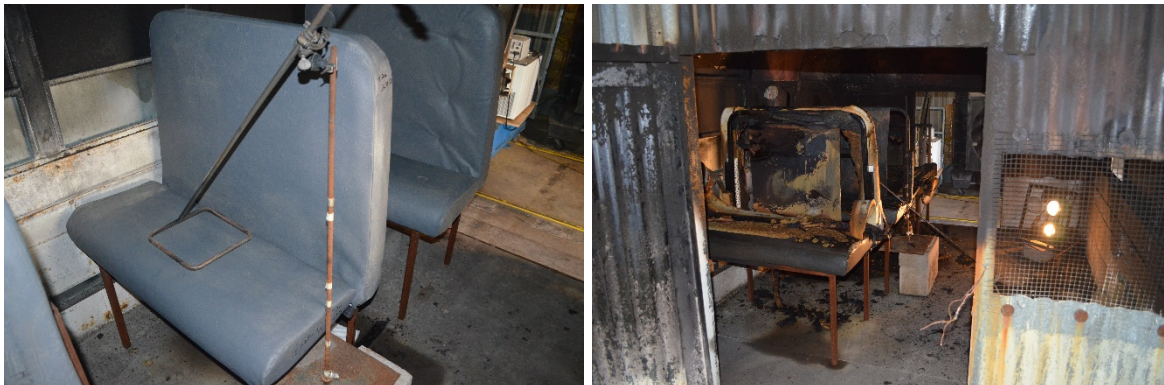
Figure 21. Pre (left) and post (right) test photographs of Trans Tech school bus seat
