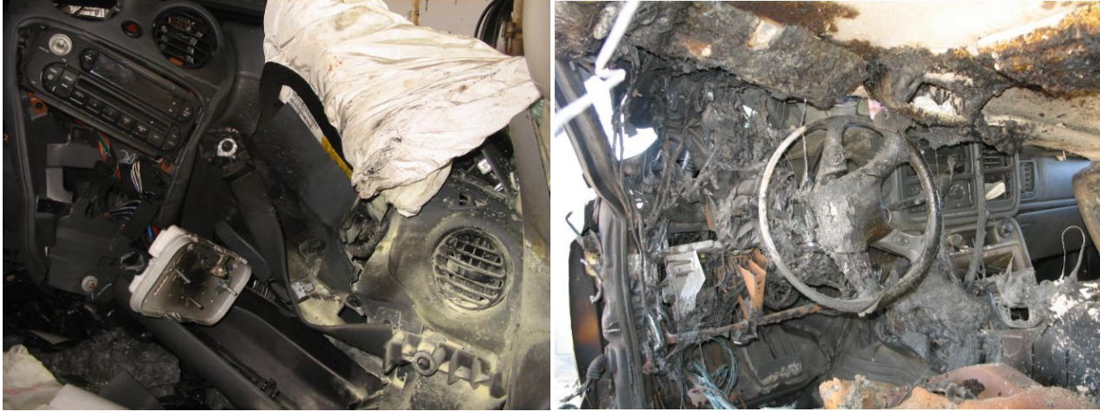
Figure B-59. Example cases with fire ingress through dash/firewall. Left (2009-45-186) right (2011-78-134)
