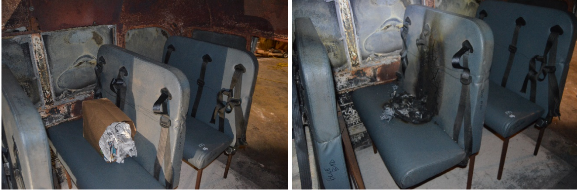
Figure 27. Pre (left) and post (right) test photographs from Test 5 of second series of testing Table 13 provides a summary of the heat release rate parameters.
