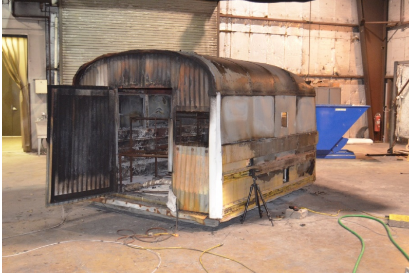
Figure 15. Photograph of SwRI test chamber for ASTM E2574
