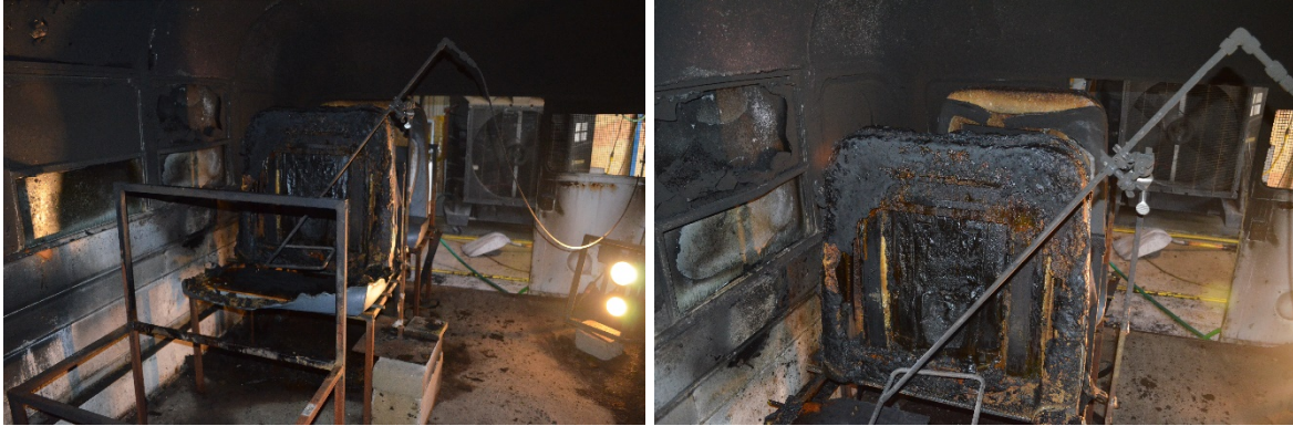
Figure 22. Post-test photographs of Starcraft school bus seats
