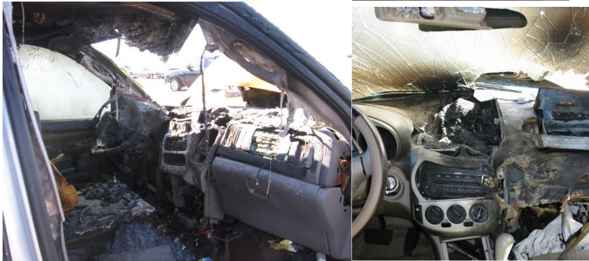
Figure B-57. Example cases with fire ingress through the windshield and over the dash. top left (2004-02-65) top right (2011-09-38) bottom left (2005-50-147) bottom right (2005-43-215)
