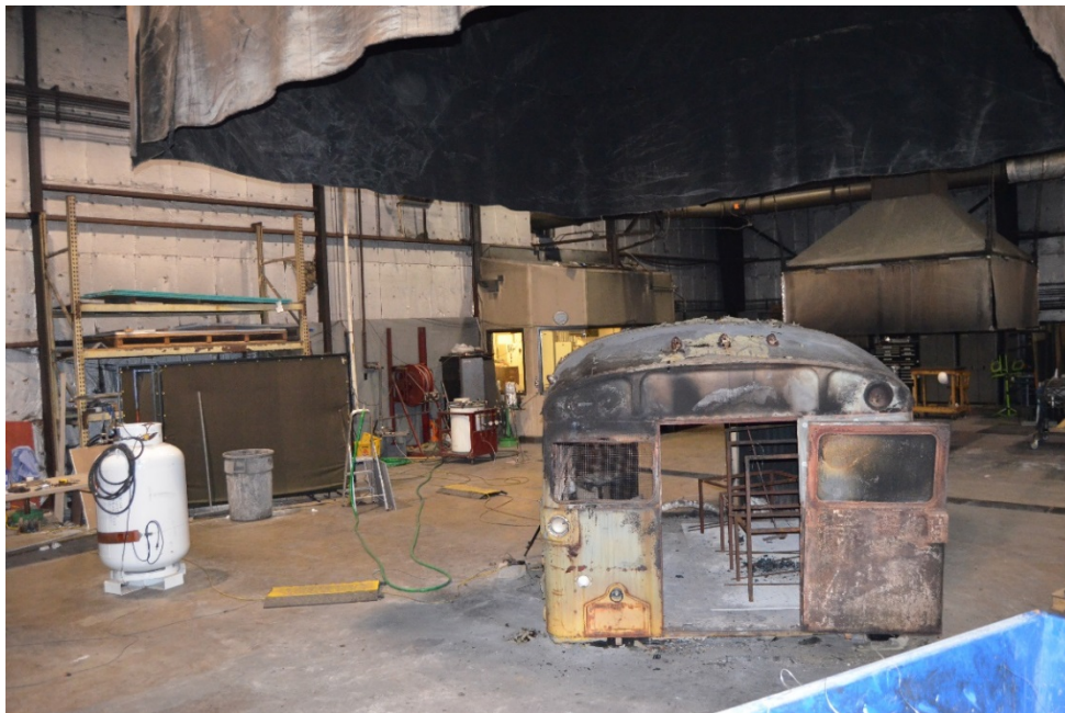
Figure 19. Photograph of SwRI test chamber under large calorimeter
