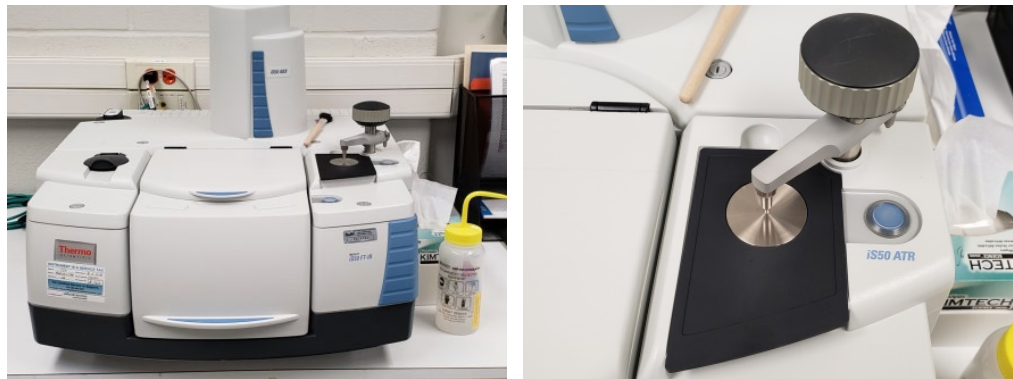
Figure 34. FTIR Spectrometer (left) and Diamond ATR Module (right)
